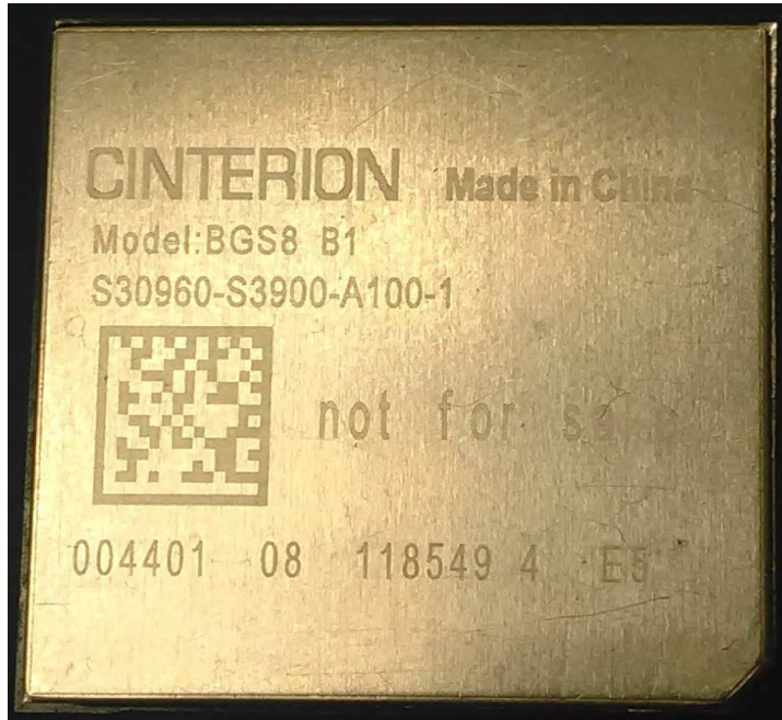
BGS8 - label location lasing on shielding
