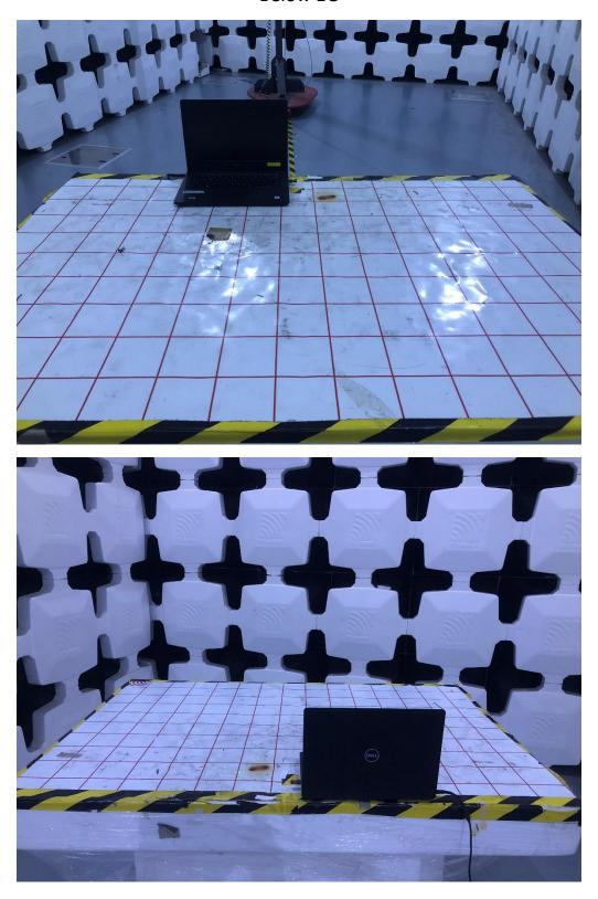
The EUT is Placed at the center of the Turntable.
