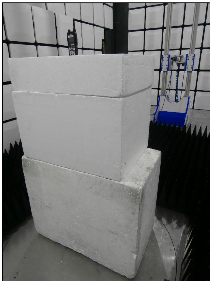
Figure 21 - Test Setup - 18 GHz to 25 GHz - Y Orientation
