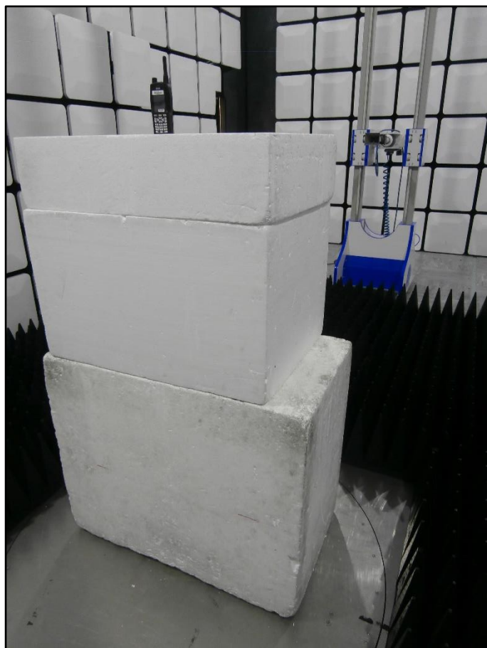
Figure 18 - Test Setup - 1 GHz to 18 GHz - Y Orientation
