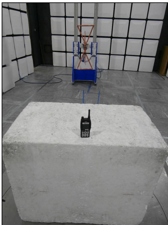
Figure 15 - Test Setup - 30 MHz to 1 GHz - Y Orientation
