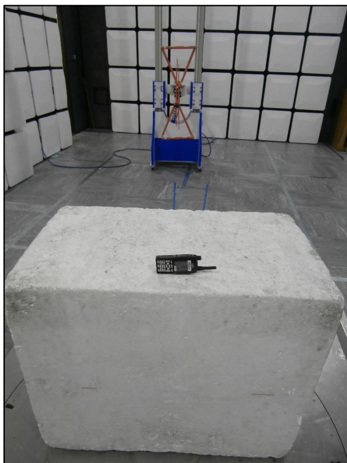
Figure 16 - Test Setup - 30 MHz to 1 GHz - Z Orientation
