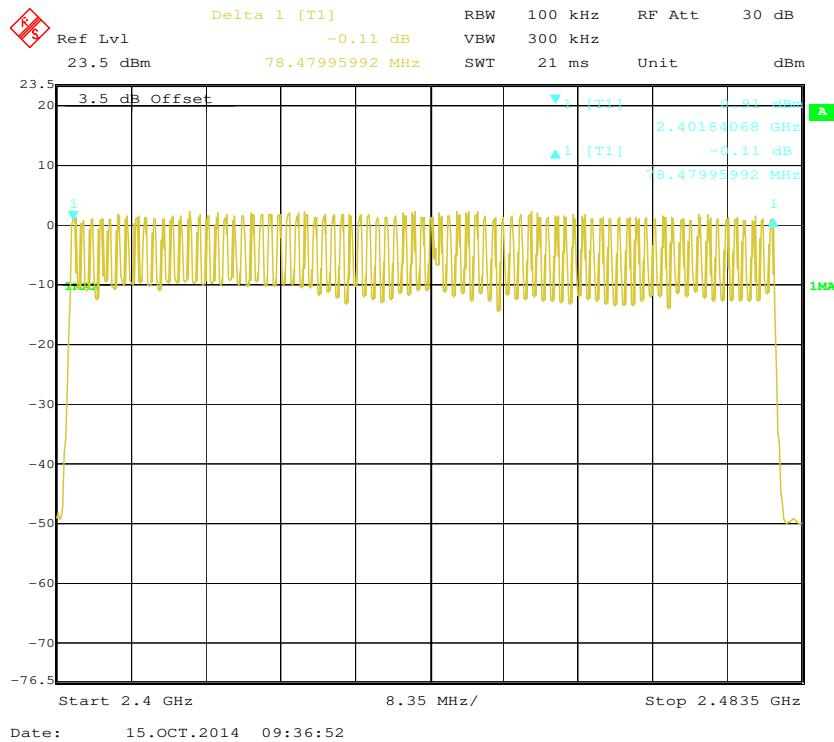
**EDR ( $\pi/4$ -DQPSK): Number of Hopping Channels**
