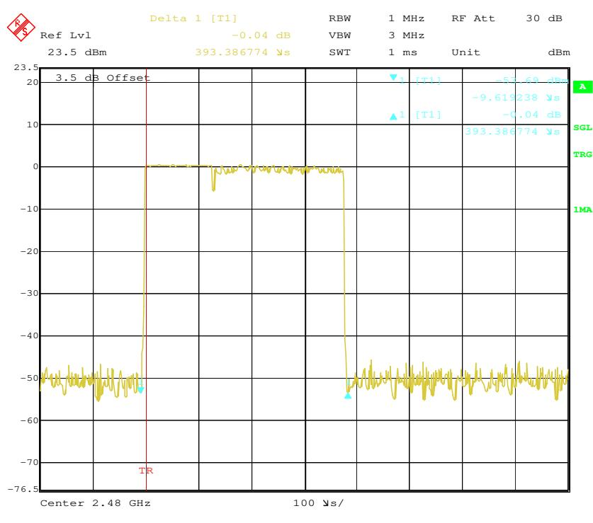
**Pulse time, Low Channel, 2DH3**
