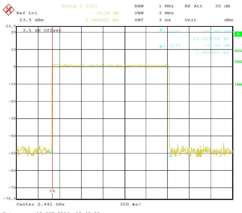
**Pulse time, High Channel, 2DH3**
