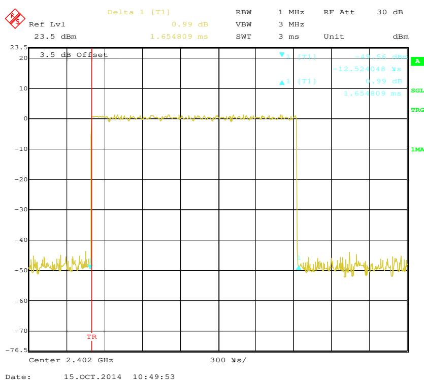
**Pulse time, Middle Channel, 3DH3**
