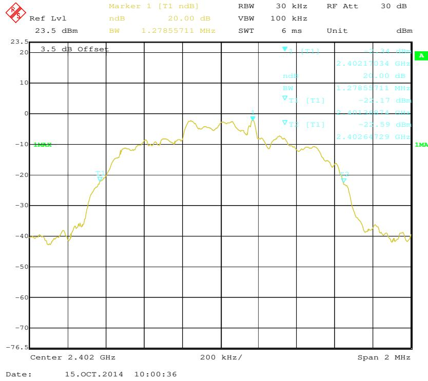
**EDR (8DPSK): Middle Channel**
