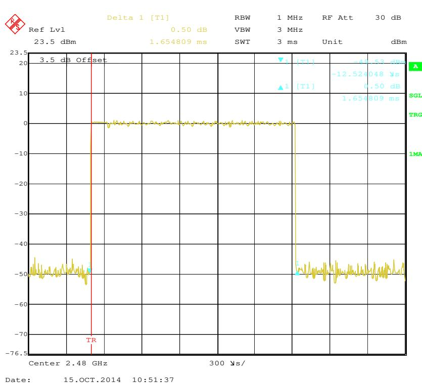
**Pulse time, Low Channel, 3DH5**
