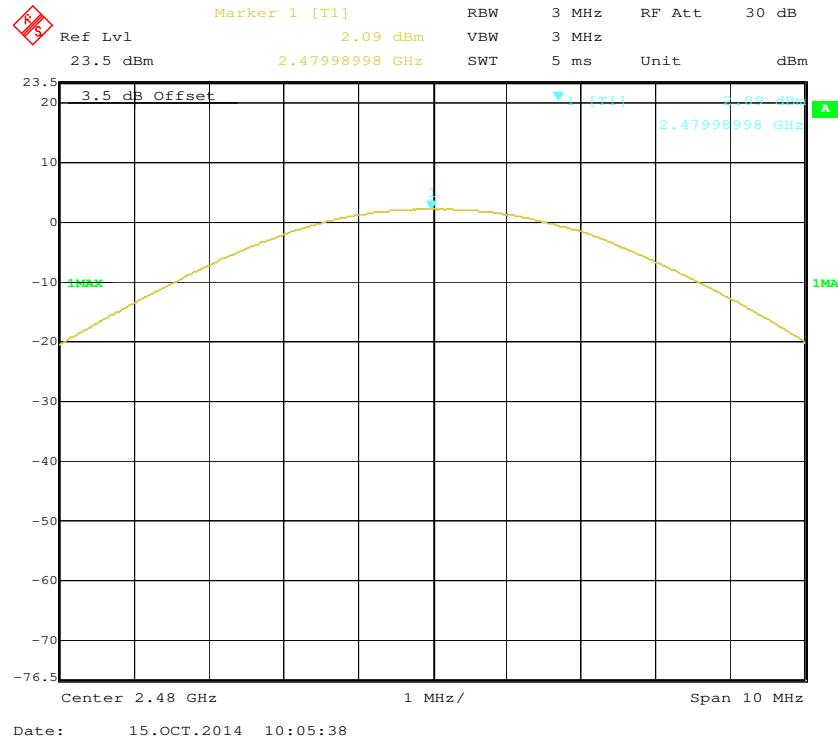
**EDR( $\pi/4$ -DQPSK): Low Channel**
