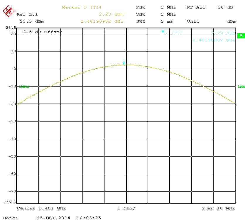
**EDR(8DPSK): Middle Channel**
