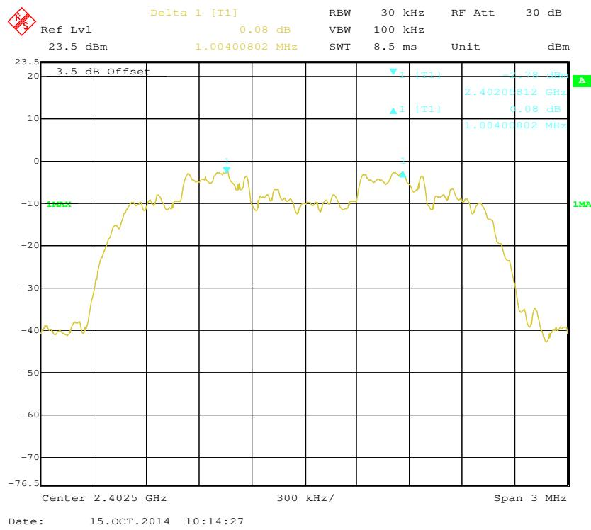
**EDR ( $\pi/4$ -DQPSK): Middle Channel**
