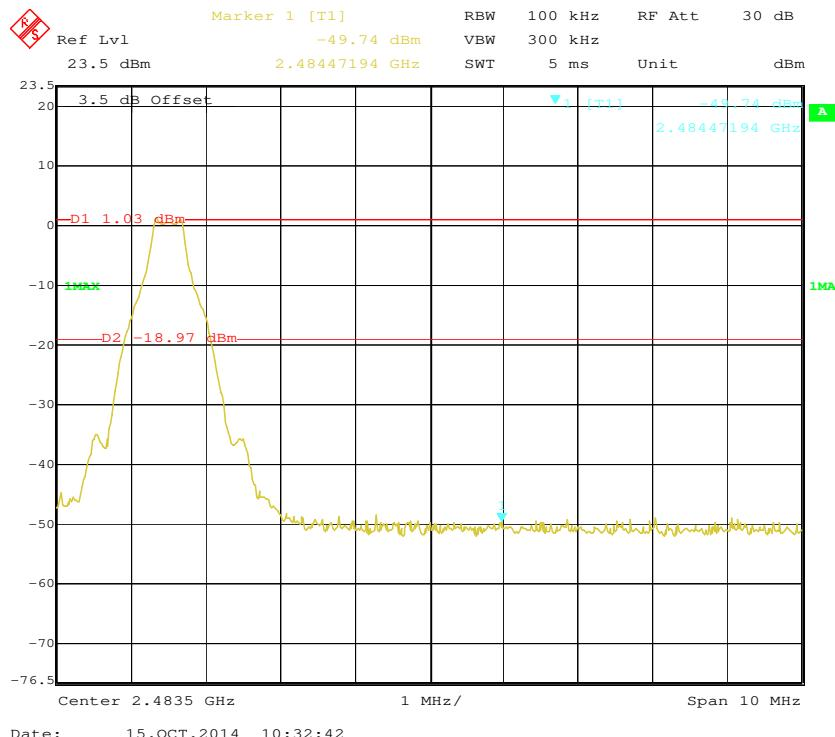
**EDR ( $\pi/4$ -DQPSK): Band Edge-Left Side**
