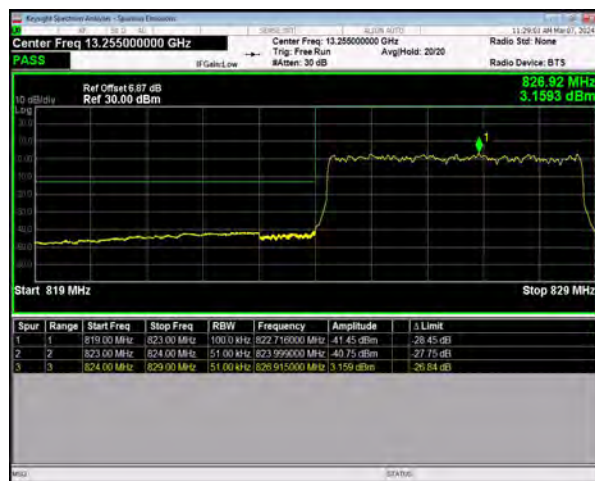
n5 SCS=15kHz DFT_256QAM BW=5MHz LowChannel=165300 RB=25@0
