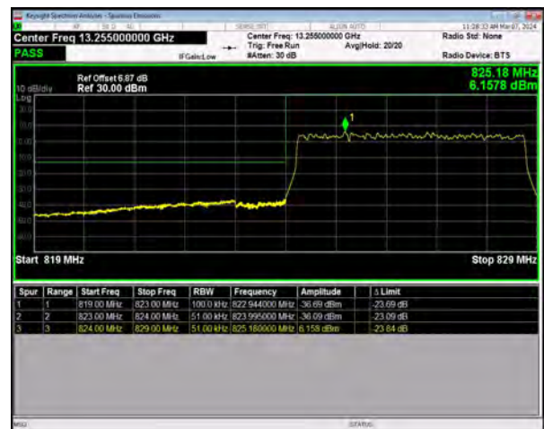
n5 SCS=15kHz DFT_16QAM BW=5MHz LowChannel=165300 RB=25@0
