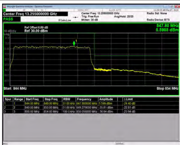
n5 SCS=15kHz DFT_16QAM BW=5MHz HighChannel=169300 RB=25@0
