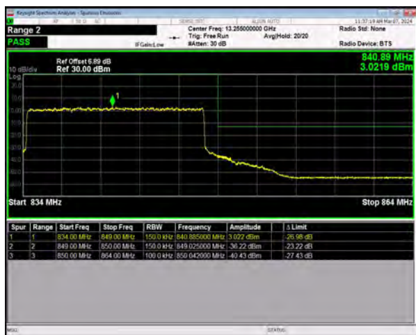
n5 SCS=15kHz DFT_BPSK BW=15MHz HighChannel=168300 RB=75@0
