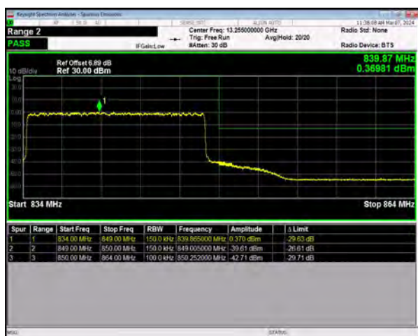
n5 SCS=15kHz DFT_64QAM BW=15MHz HighChannel=168300 RB=75@0
