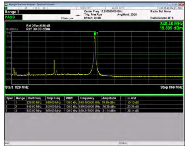
n5 SCS=15kHz DFT_QPSK BW=20MHz HighChannel=167800 RB=1@105
