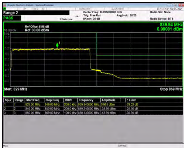
n5 SCS=15kHz DFT_64QAM BW=20MHz HighChannel=167800 RB=100@0
