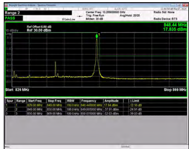
n5 SCS=15kHz DFT_16QAM BW=20MHz HighChannel=167800 RB=1@105
