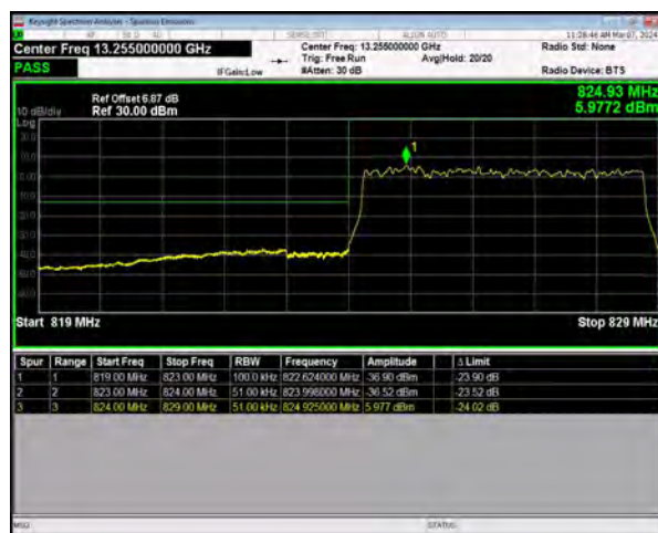
n5 SCS=15kHz DFT_64QAM BW=5MHz LowChannel=165300 RB=25@0
