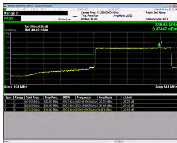
n5 SCS=15kHz DFT_64QAM BW=20MHz LowChannel=166800 RB=100@0
