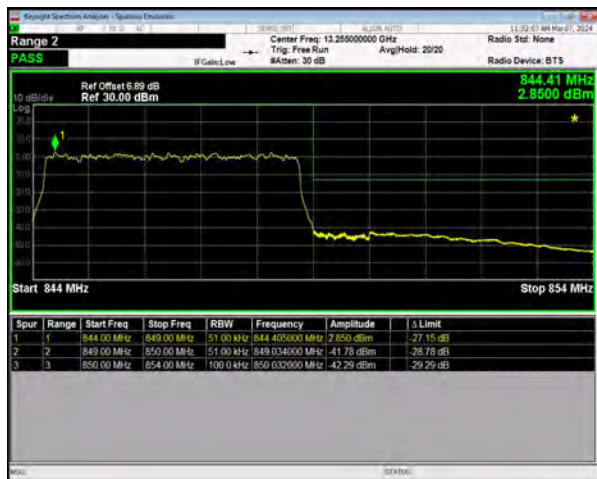
n5 SCS=15kHz DFT_256QAM BW=5MHz HighChannel=169300 RB=25@0
