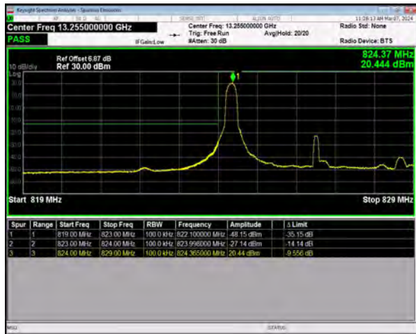
n5 SCS=15kHz DFT_QPSK BW=5MHz LowChannel=165300 RB=1@0
