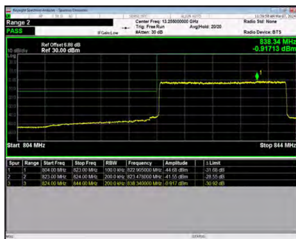
n5 SCS=15kHz DFT_256QAM BW=20MHz LowChannel=166800 RB=100@0
