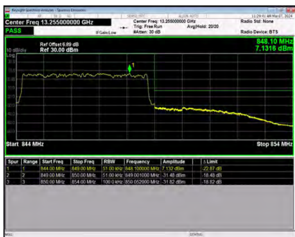
n5 SCS=15kHz DFT_QPSK BW=5MHz HighChannel=169300 RB=25@0
