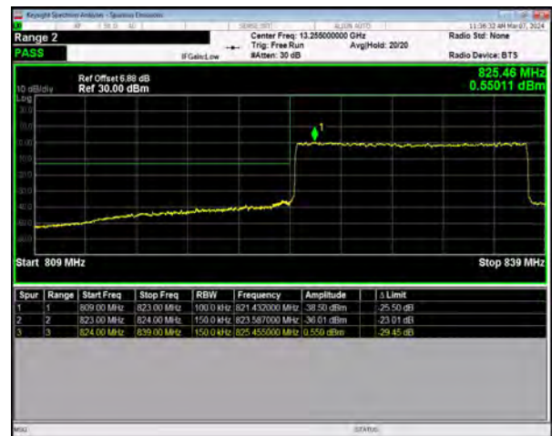
n5 SCS=15kHz DFT_64QAM BW=15MHz LowChannel=166300 RB=75@0
