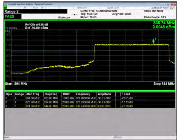
n5 SCS=15kHz DFT_BPSK BW=20MHz LowChannel=166800 RB=100@0
