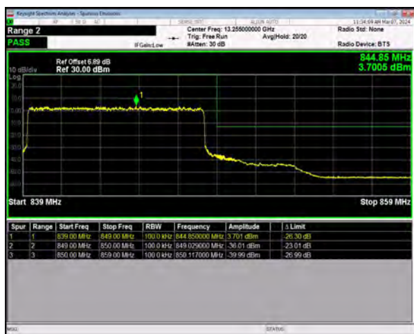
n5 SCS=15kHz DFT_BPSK BW=10MHz HighChannel=168800
