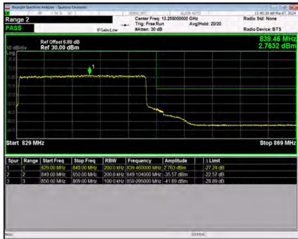
n5 SCS=15kHz DFT_BPSK BW=20MHz HighChannel=167800 RB=100@0
