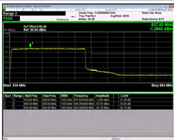
n5 SCS=15kHz DFT_256QAM BW=15MHz HighChannel=168300 RB=75@0
