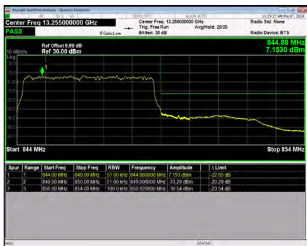
n5 SCS=15kHz DFT_BPSK BW=5MHz HighChannel=169300 RB=25@0
