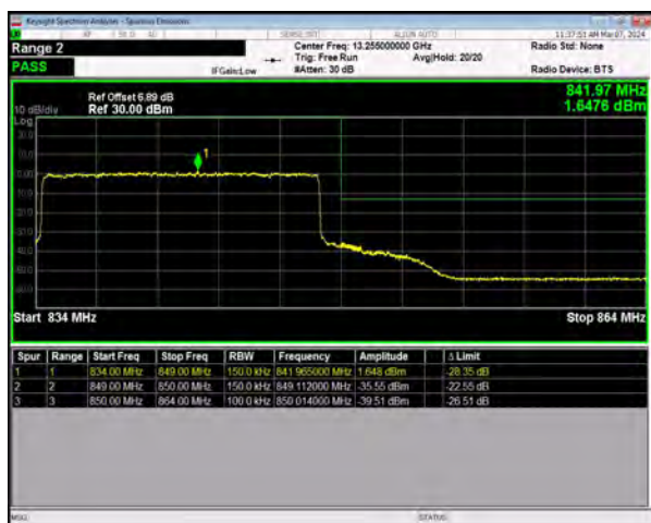
n5 SCS=15kHz DFT_16QAM BW=15MHz HighChannel=168300 RB=75@0
