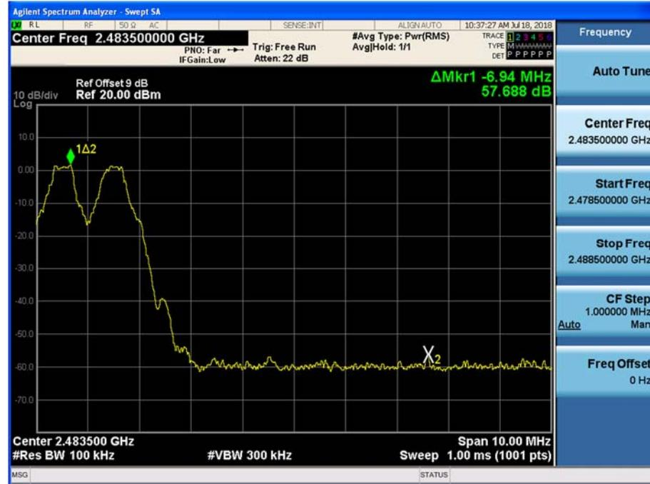
Test Plots with hopping (8DPSK)
