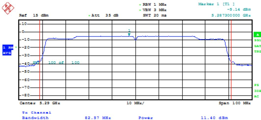
**Section 15.407 Subclause (b) (2) / RSS-210 A9.2. (2). Undesirable radiated emissions (Transmitter) 1 to 40 GHz**
