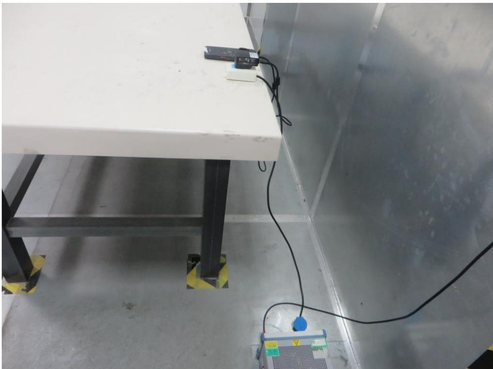
Description: Radiated Spurious Emission Test Setup Below 1GHz
