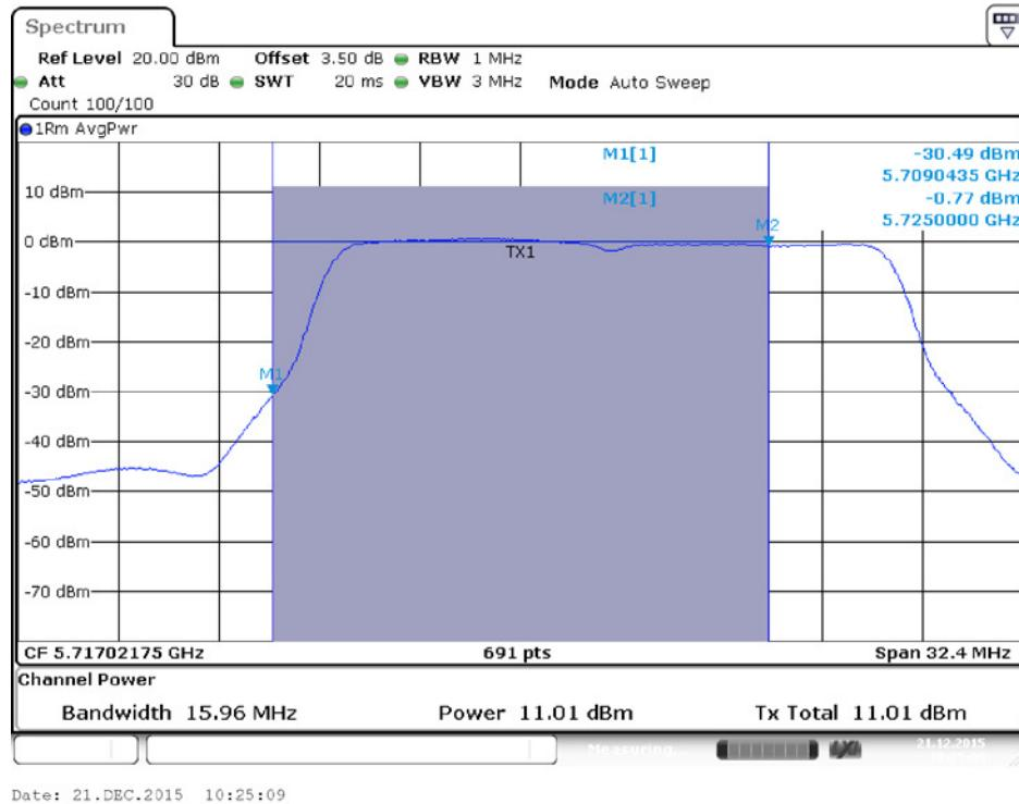
**Conducted Output Power Plot on Configuration IEEE 802.11ac MCS0/Nss1 VHT20 / Chain 4 / 5720 MHz (UNII2C)**
