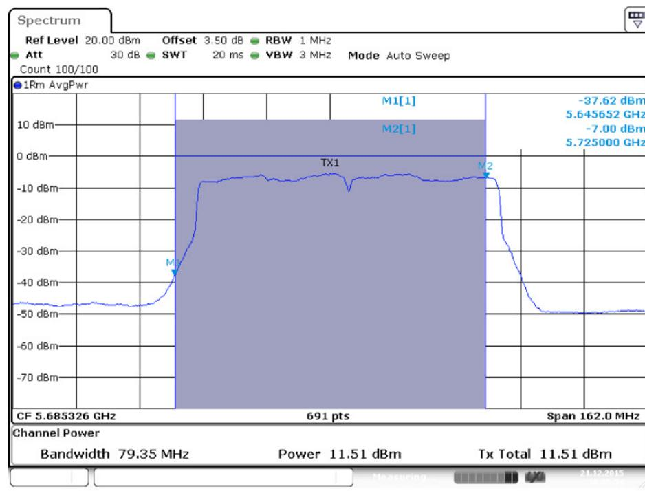
**Conducted Output Power Plot on Configuration IEEE 802.11ac MCS0/Nss1 VHT80 / Chain 1 / 5690 MHz (UNII 3)**
