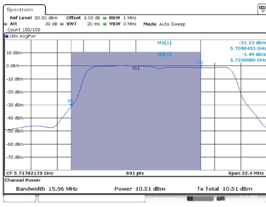
**Conducted Output Power Plot on Configuration IEEE 802.11ac MCS0/Nss1 VHT20 / Chain 3 / 5720 MHz (UNII2C)**
