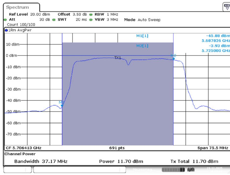
**Conducted Output Power Plot on Configuration IEEE 802.11ac MCS0/Nss1 VHT40 / Chain 1 / 5710 MHz (UNII 3)**
