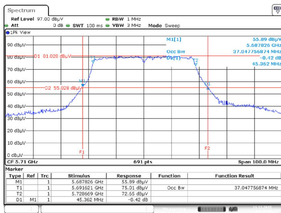
**26dB Bandwidth and 99% Occupied Bandwidth Plot on Configuration IEEE 802.11ac MCS0/Nss1
