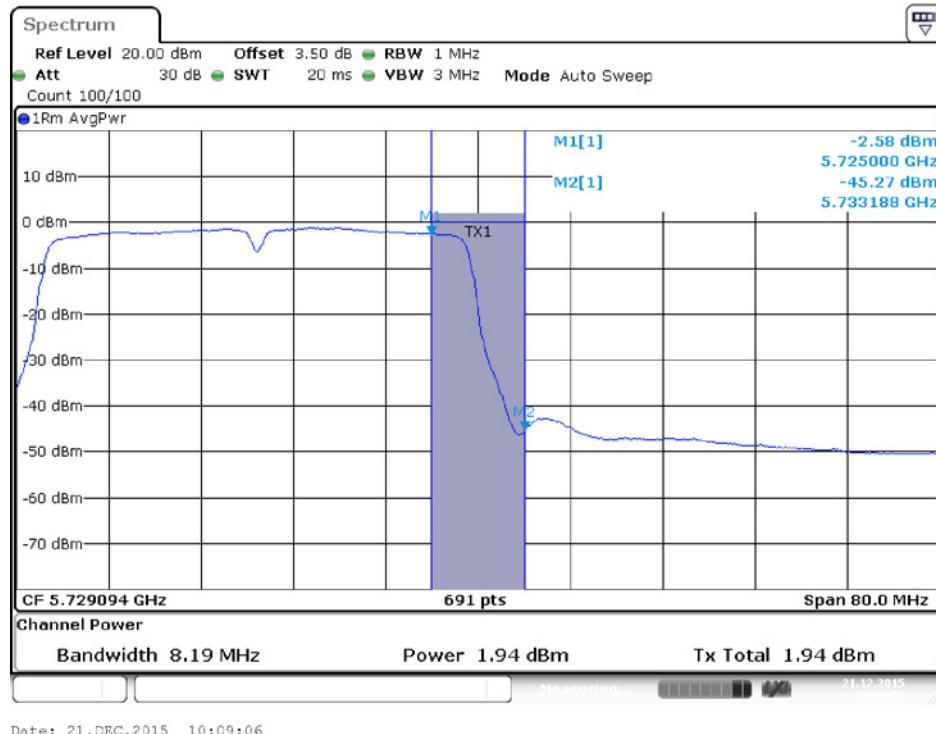
**Conducted Output Power Plot on Configuration IEEE 802.11ac MCS0/Nss1 VHT40 / Chain 2 / 5710 MHz (UNII 3)**
