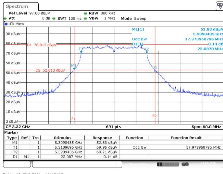
**26dB Bandwidth and 99% Occupied Bandwidth Plot on Configuration IEEE 802.11ac MCS0/ Nss1**
