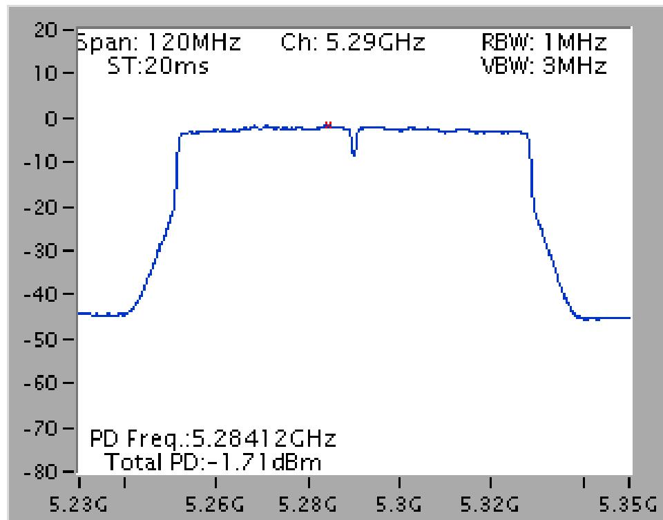
**Power Density Plot on Configuration IEEE 802.11ac MCS0/Nss1 VHT80 / Chain 1 + Chain 2 + Chain 3
