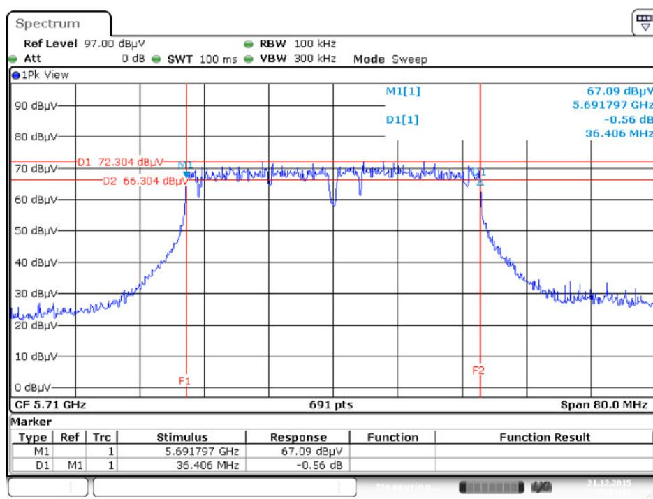
**6 dB Bandwidth Plot on Configuration IEEE 802.11ac MCS0/Nss1 VHT80 / Chain 1 + Chain 2 + Chain 3 + Chain 4 / 5690 MHz**
