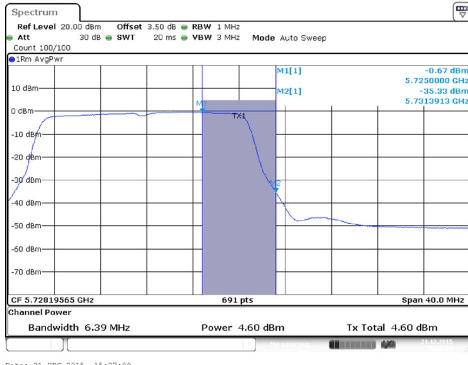
**Conducted Output Power Plot on Configuration IEEE 802.11ac MCS0/Nss1 VHT20 / Chain 4 / 5720 MHz (UNII 3)**
