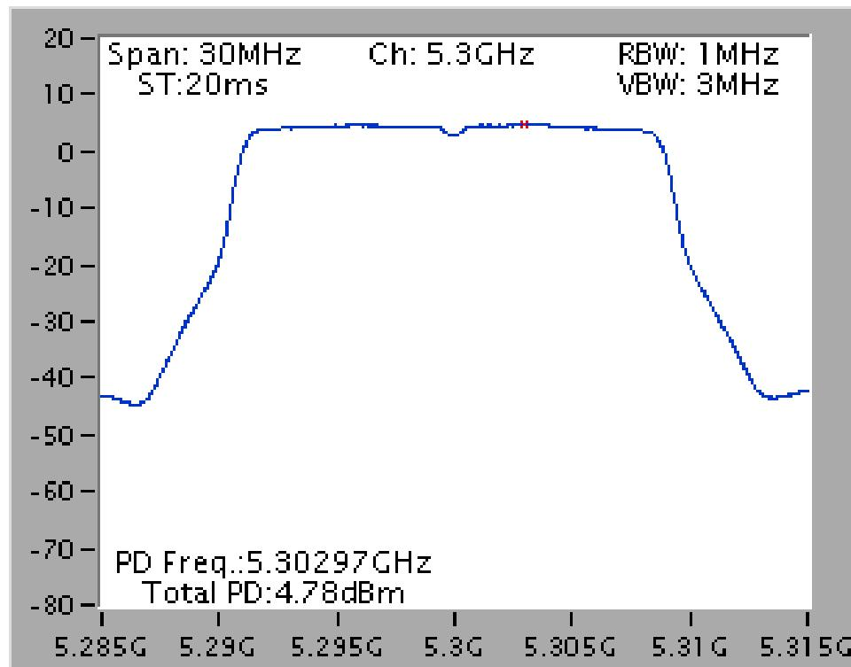
**Power Density Plot on Configuration IEEE 802.11ac MCS0/Nss1 VHT20 / Chain 1 + Chain 2 + Chain 3
