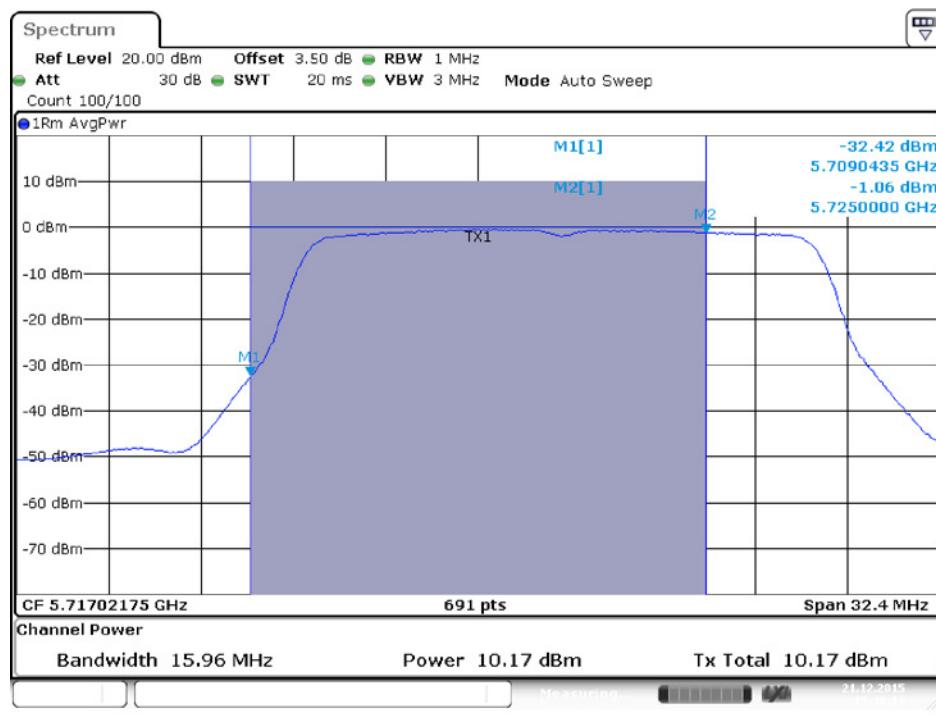
**Conducted Output Power Plot on Configuration IEEE 802.11ac MCS0/Nss1 VHT20 / Chain 1 / 5720 MHz (UNII 3)**
