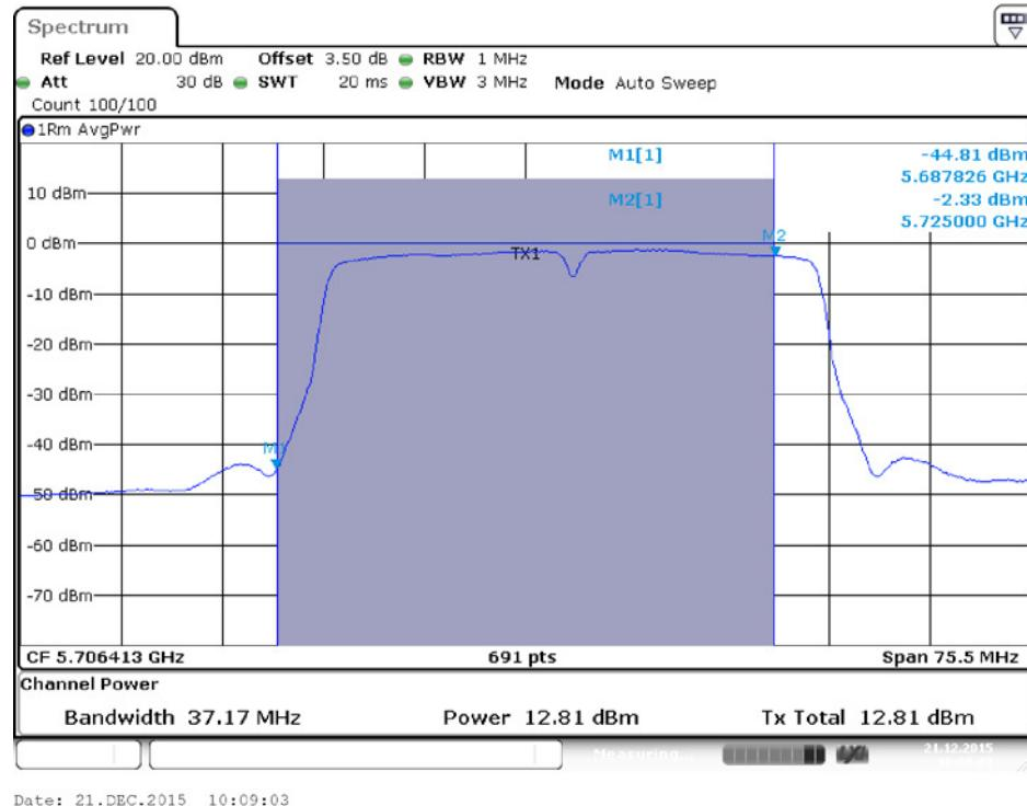
**Conducted Output Power Plot on Configuration IEEE 802.11ac MCS0/Nss1 VHT40 / Chain 2 / 5710 MHz (UNII2C)**
