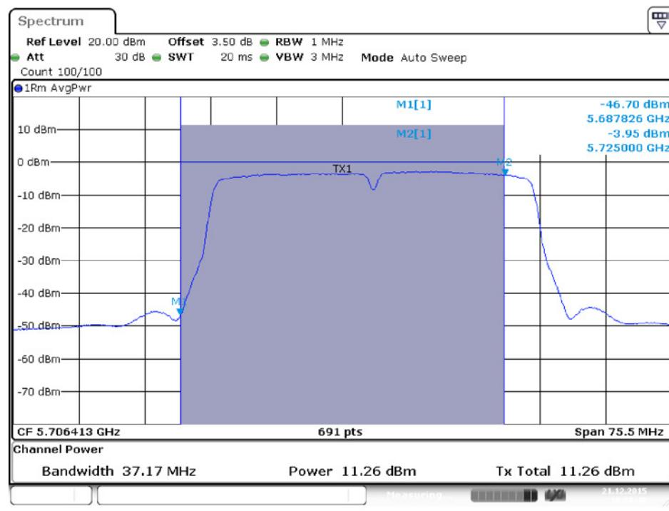
**Conducted Output Power Plot on Configuration IEEE 802.11ac MCS0/Nss1 VHT40 / Chain 3 / 5710 MHz (UNII2C)**
