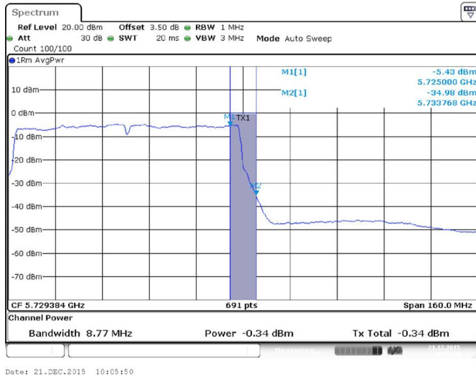
**Conducted Output Power Plot on Configuration IEEE 802.11ac MCS0/Nss1 VHT80 / Chain 2 / 5690 MHz (UNII 3)**
