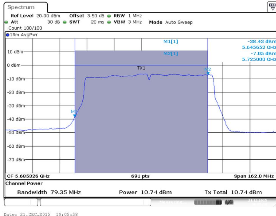
**Conducted Output Power Plot on Configuration IEEE 802.11ac MCS0/Nss1 VHT80 / Chain 4 / 5690 MHz (UNII2C)**
