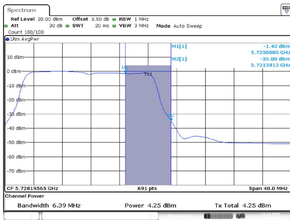
**Conducted Output Power Plot on Configuration IEEE 802.11ac MCS0/Nss1 VHT40 / Chain 1 / 5710 MHz (UNII2C)**
