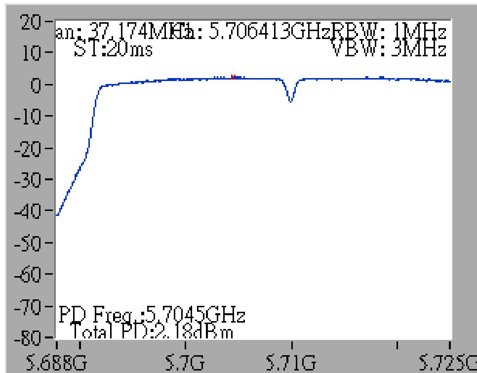
**Power Density Plot on Configuration IEEE 802.11ac MCS0/Nss1 VHT40 / Chain 1 + Chain 2 + Chain 3
