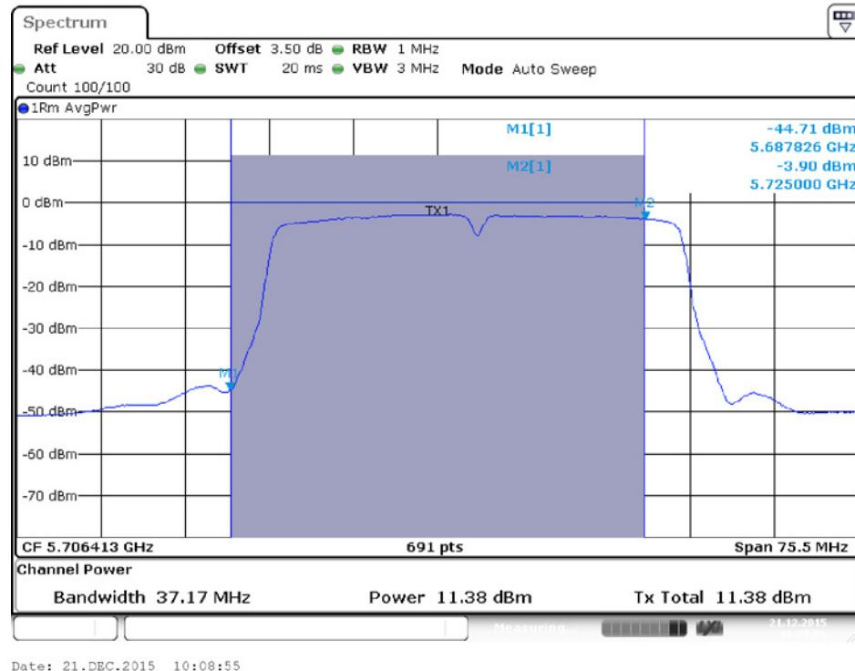
**Conducted Output Power Plot on Configuration IEEE 802.11ac MCS0/Nss1 VHT40 / Chain 4 / 5710 MHz (UNII2C)**
