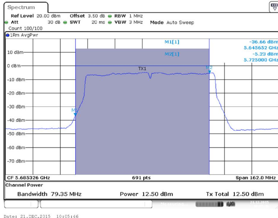
**Conducted Output Power Plot on Configuration IEEE 802.11ac MCS0/Nss1 VHT80 / Chain 2 / 5690 MHz (UNII2C)**
