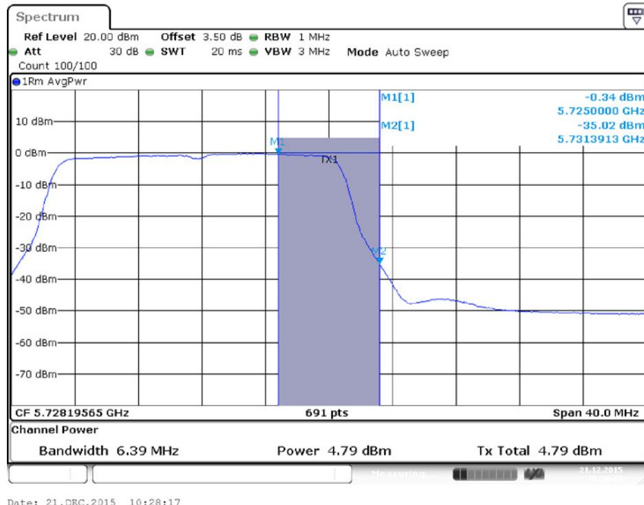
**Conducted Output Power Plot on Configuration IEEE 802.11ac MCS0/Nss1 VHT20 / Chain 2 / 5720 MHz (UNII 3)**
