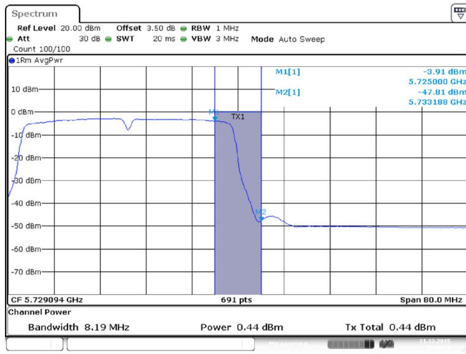
**Conducted Output Power Plot on Configuration IEEE 802.11ac MCS0/Nss1 VHT80 / Chain 1 / 5690 MHz (UNII2C)**
