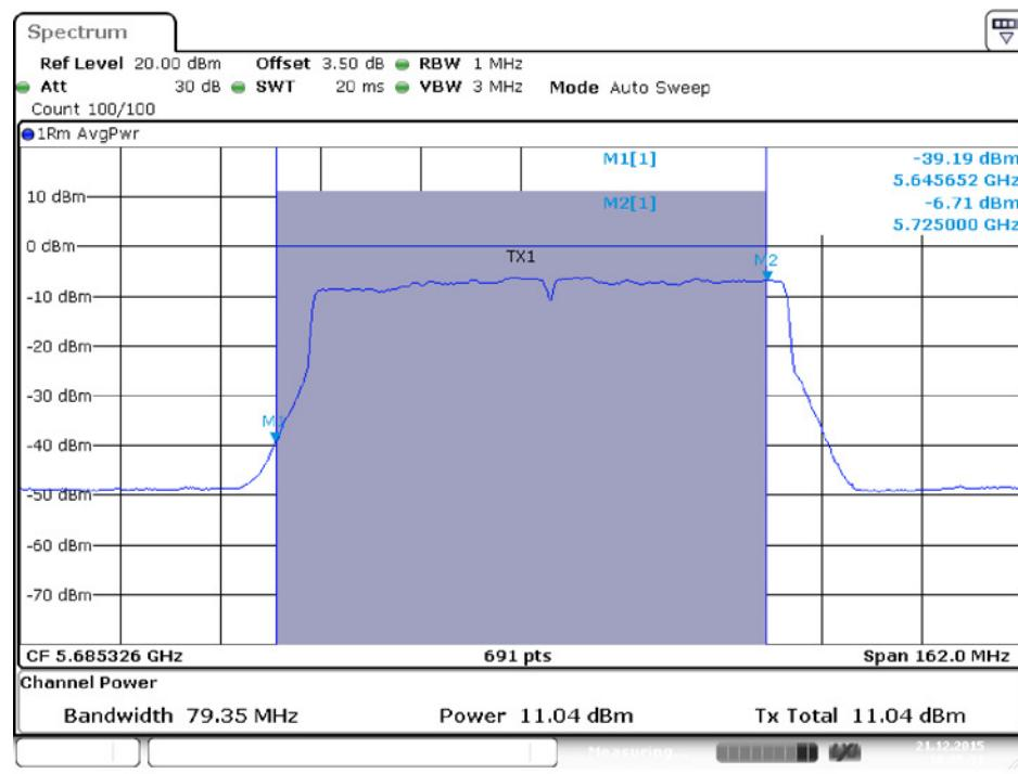
**Conducted Output Power Plot on Configuration IEEE 802.11ac MCS0/Nss1 VHT80 / Chain 3 / 5690 MHz (UNII2C)**
