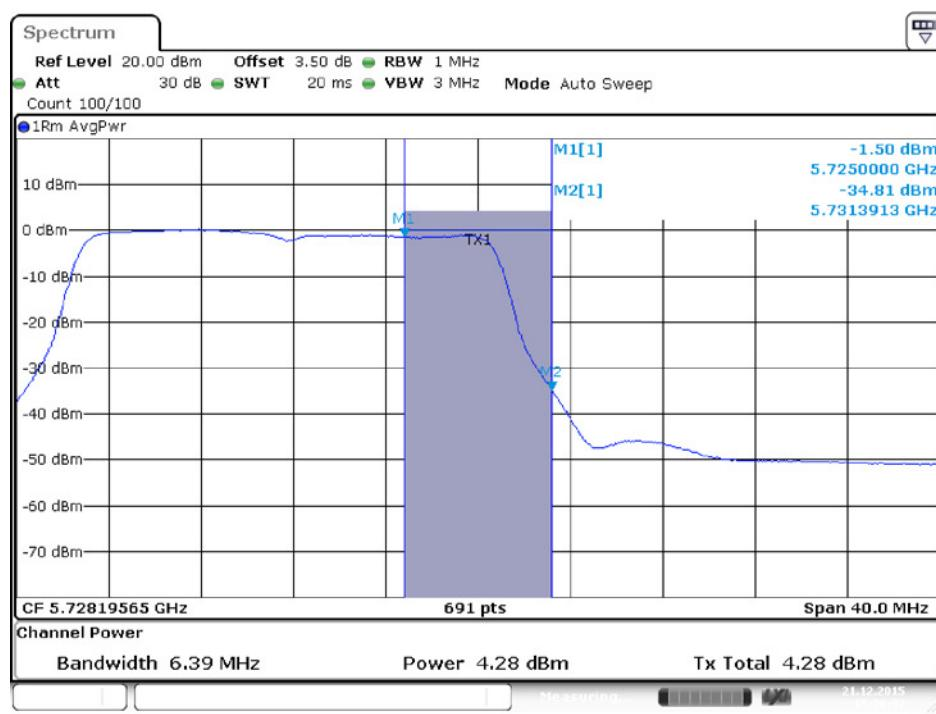
**Conducted Output Power Plot on Configuration IEEE 802.11ac MCS0/Nss1 VHT20 / Chain 3 / 5720 MHz (UNII 3)**
