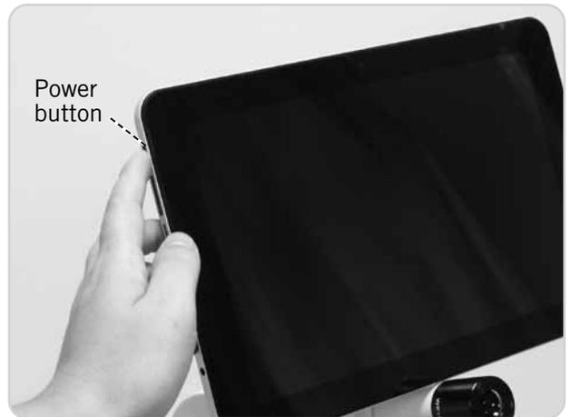
**Step 4:** Press and hold the power button for 2-3 seconds to boot the Moticam T2.
