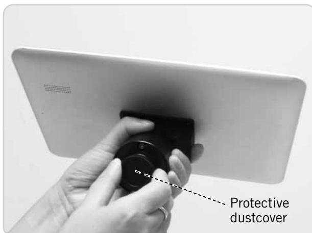
**Step 1:** Unscrew the protective dust cover from the bottom of the Moticam T2 to expose the imaging sensor to light.
