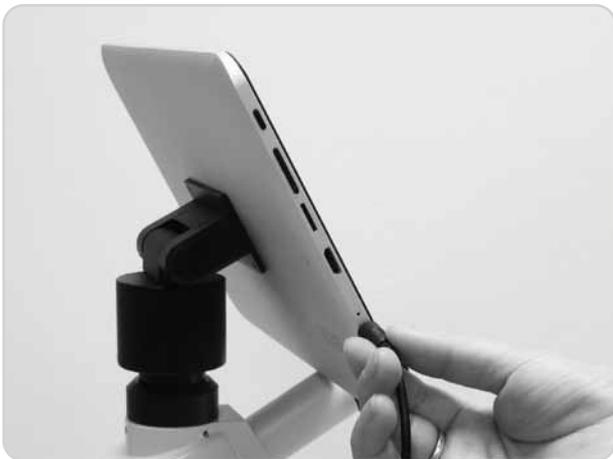
**Step 3:** Plug in the Moticam T2 power supply and press the power button to start.
