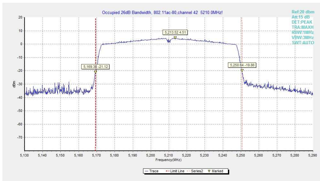
Fig.29 Occupied 26dB Bandwidth (802. 11ac-HT80, 5210MHz)
