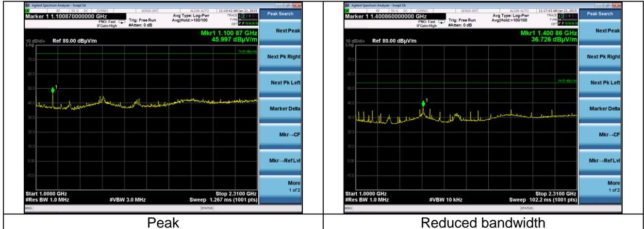
**Note:** In addition to investigation with the radio disabled, the radio module was tested stand-alone and confirms that emissions seen are not those of the radio module.
