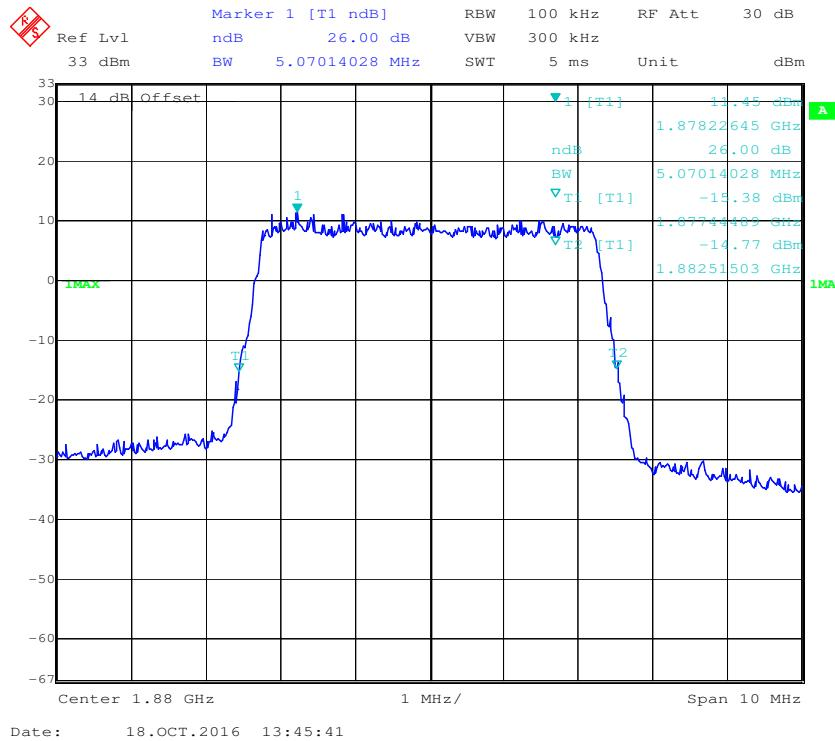
**16-QAM (5.0 MHz) - 26 dB Bandwidth, Middle channel**
