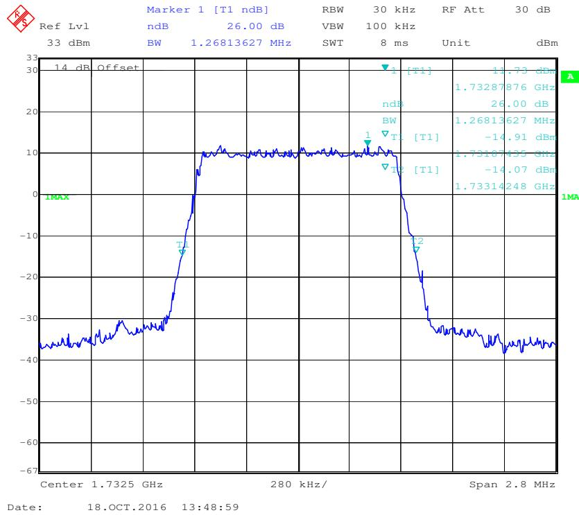
**QPSK (3.0 MHz) - 26 dB Bandwidth, Middle channel**
