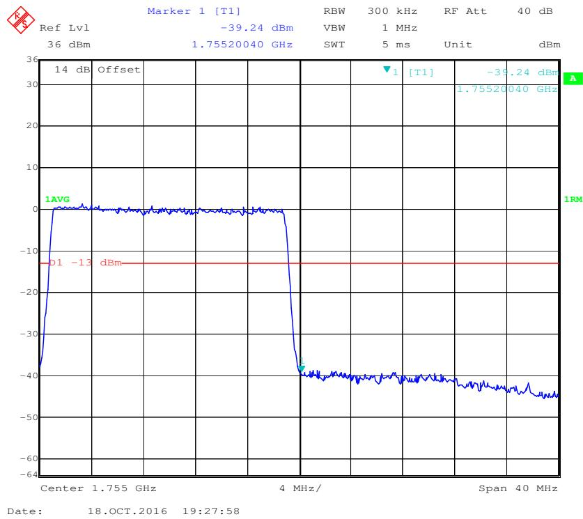
**Band 5:****QPSK (1.4 MHz, FULL RB) - Left Band Edge**
