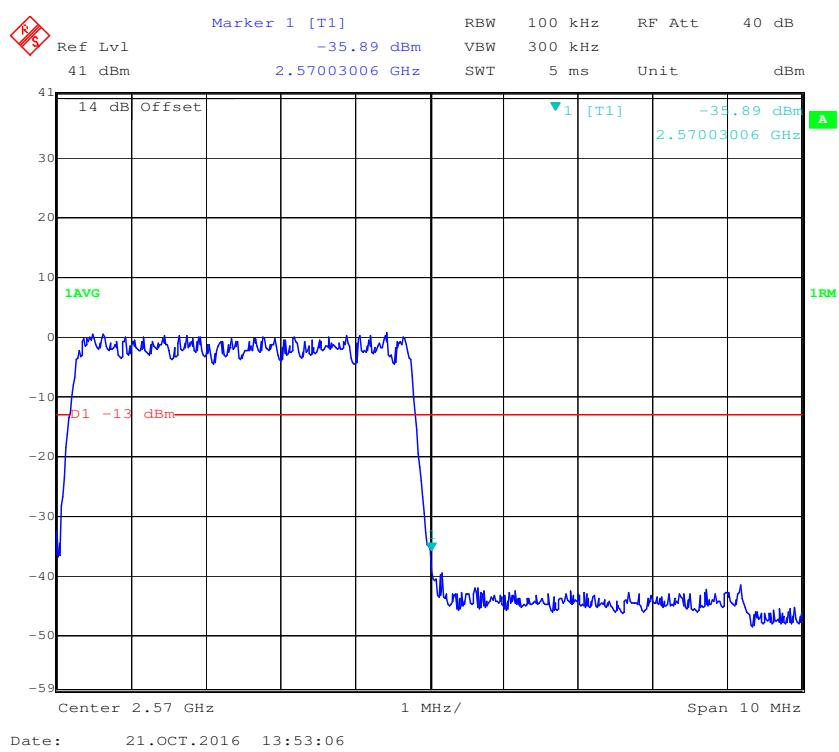
**16-QAM (5.0 MHz, FULL RB) - Left Band Edge**
