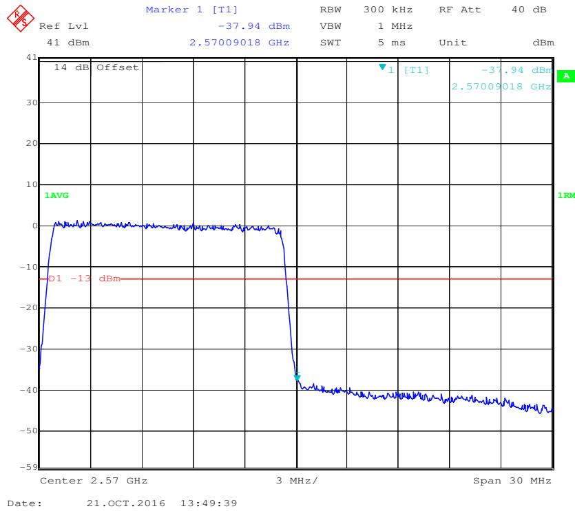
**QPSK (20.0 MHz, FULL RB) - Left Band Edge**
