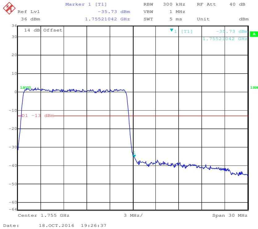
**QPSK (20.0 MHz, FULL RB) - Left Band Edge**
