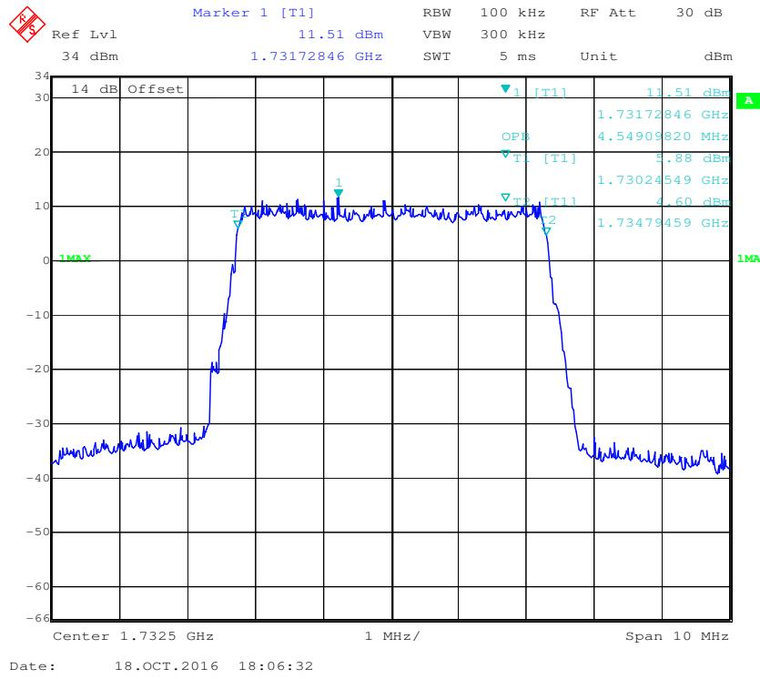
**16-QAM (5.0 MHz) - 99% Occupied Bandwidth, Middle channel**
