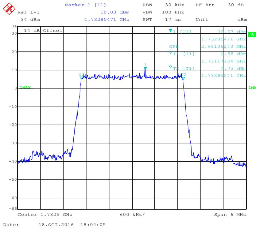
**16-QAM (3.0 MHz) - 99% Occupied Bandwidth, Middle channel**
