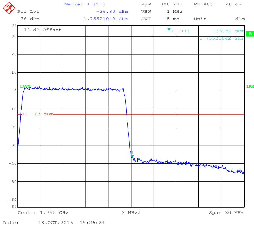
**16-QAM (15.0 MHz, FULL RB) - Left Band Edge**
