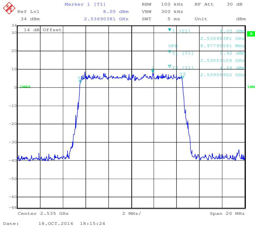
**QPSK (15.0 MHz) -99% Occupied Bandwidth, Middle channel**
