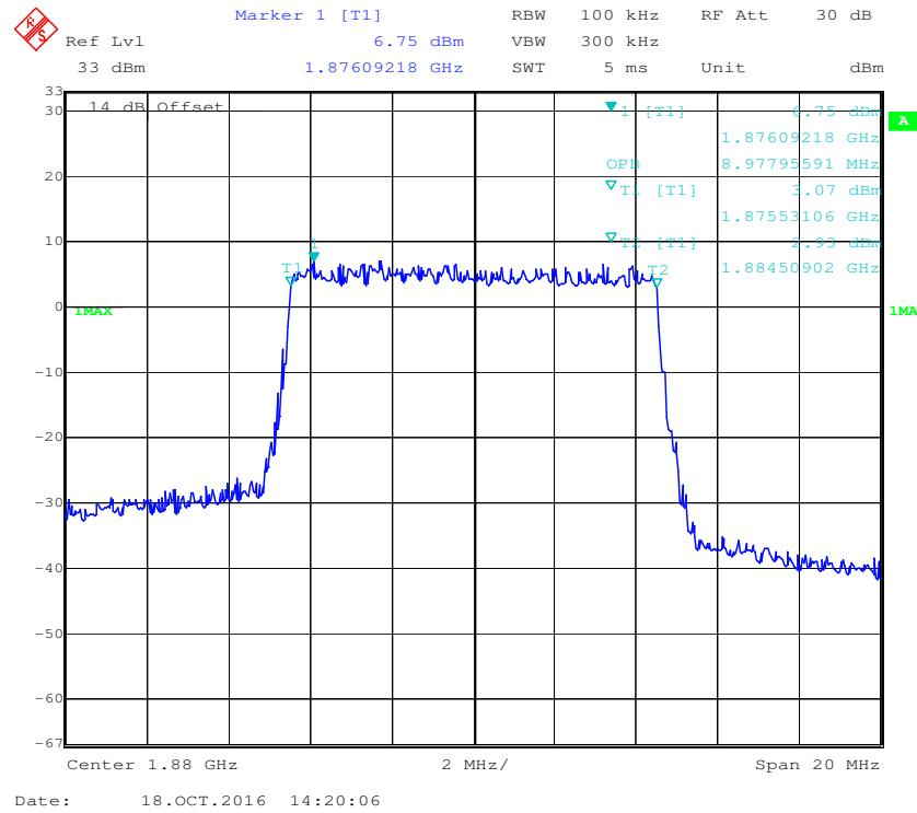
**16-QAM (10.0 MHz) - 99% Occupied Bandwidth, Middle channel**
