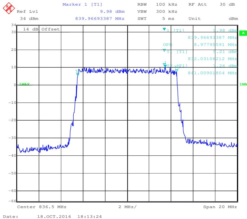
**QPSK (1.4 MHz) -26 dB Bandwidth, Middle channel**
