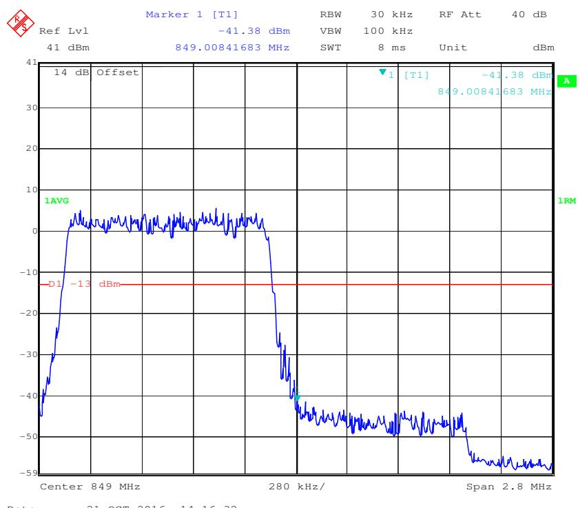
**16-QAM (1.4 MHz, FULL RB) - Left Band Edge**
