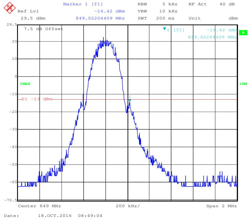
**Cellular Band, Left Band Edge for EGPRS Mode**
