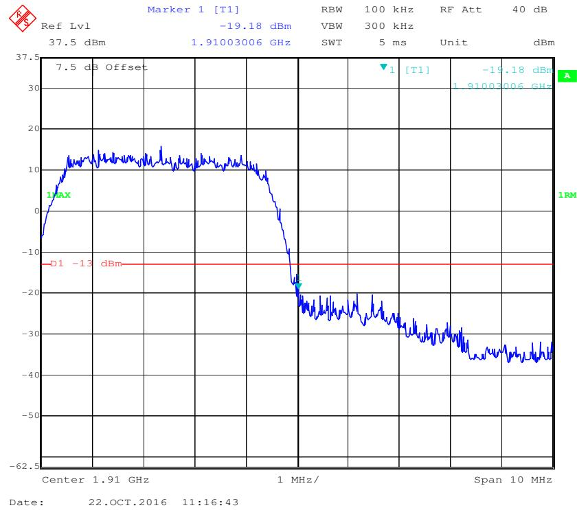
**PCS Band, Left Band Edge for HSUPA (BPSK) Mode**
