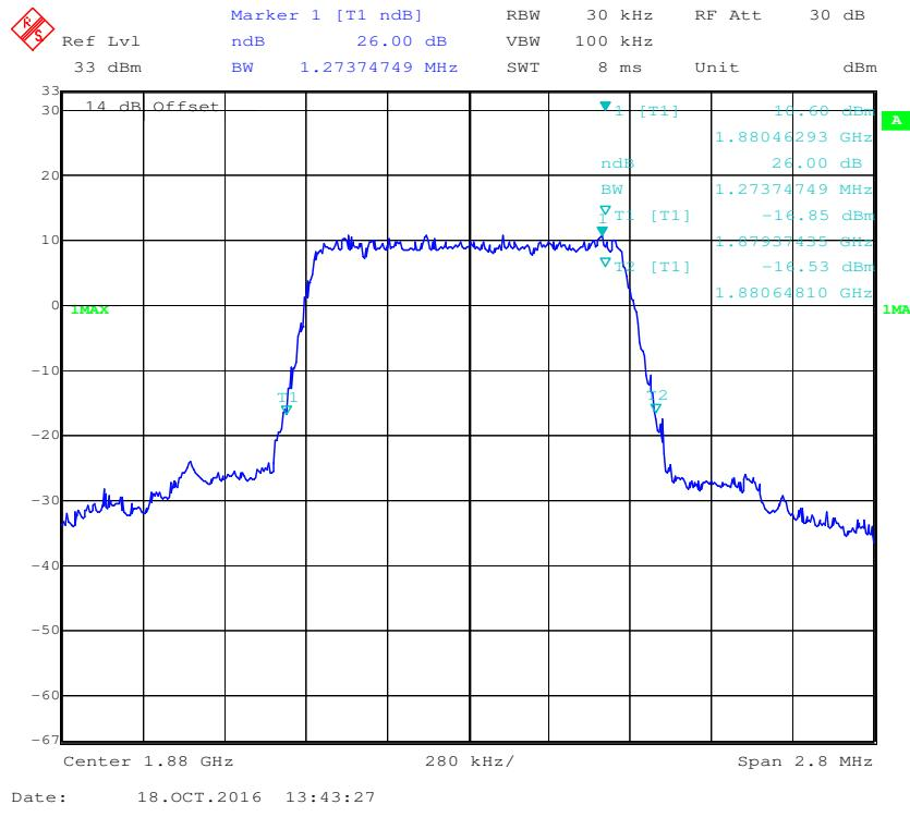
**QPSK (3.0 MHz) - 26 dB Bandwidth, Middle channel**
