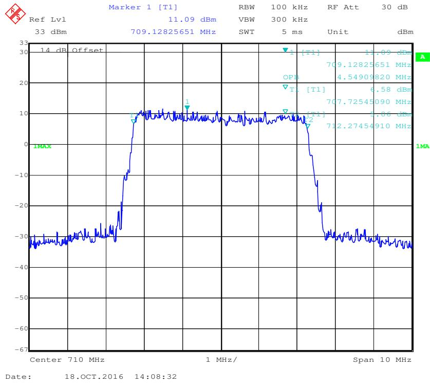
**16-QAM (5.0 MHz) - 99% Occupied Bandwidth, Middle channel**
