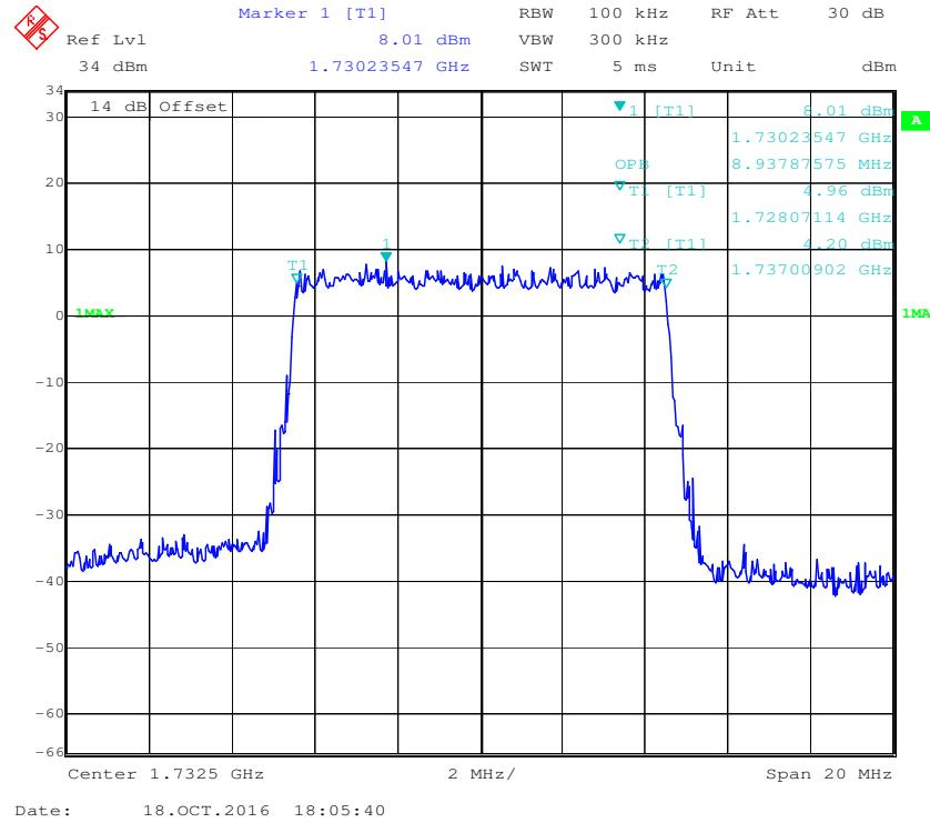
**QPSK (15.0 MHz) - 99% Occupied Bandwidth, Middle channel**
