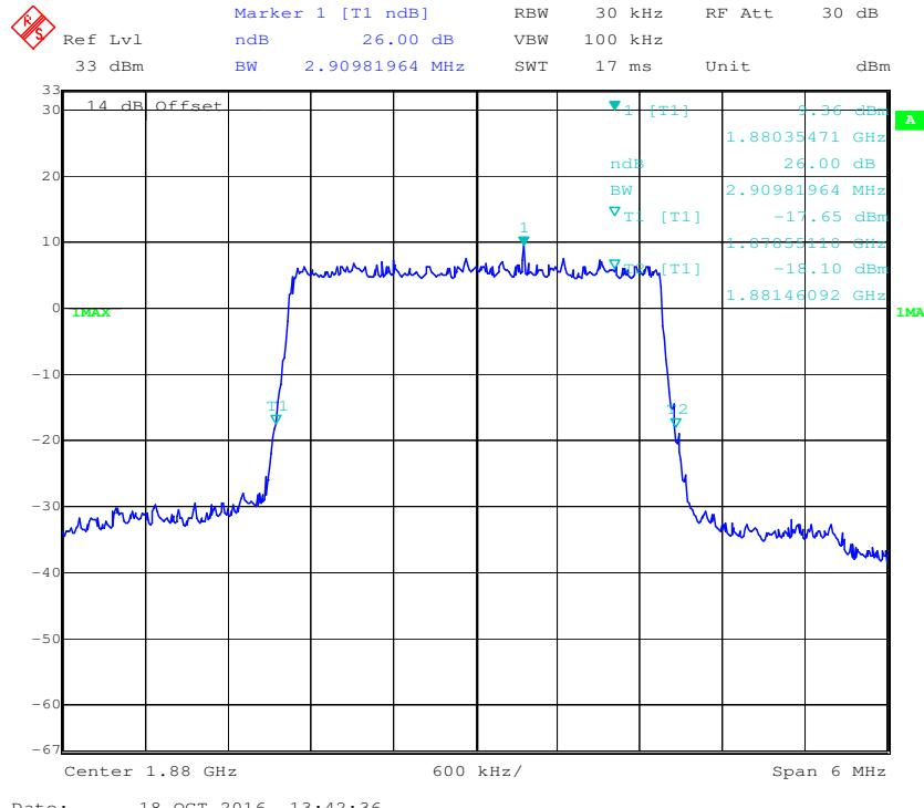
**16-QAM (3.0 MHz) - 26 dB Bandwidth, Middle channel**
