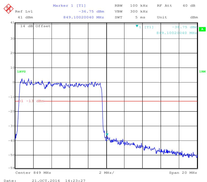
**16-QAM (10.0 MHz, FULL RB) - Left Band Edge**
