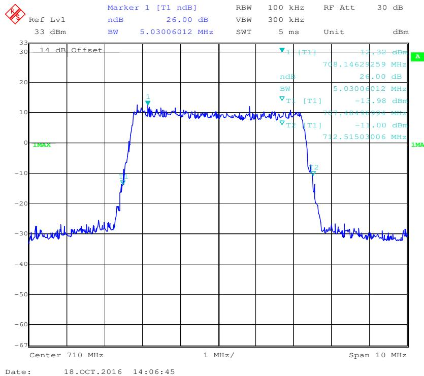
**QPSK (10.0 MHz) - 26 dB Bandwidth, Middle channel**
