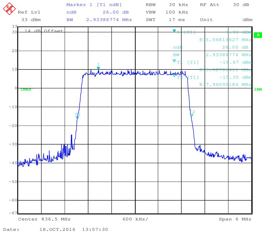
**QPSK (5.0 MHz) - 26 dB Bandwidth, Middle channel**
