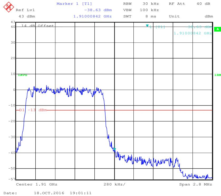
**QPSK (3.0 MHz, FULL RB) - Left Band Edge**
