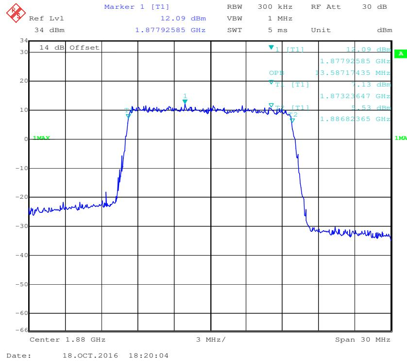
**16-QAM (15.0 MHz) - 99% Occupied Bandwidth, Middle channel**
