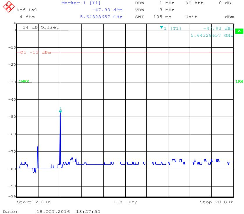
**30 MHz - 1 GHz (5.0 MHz, Middle Channel)**
