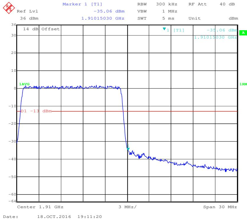
**QPSK (20.0 MHz, FULL RB) - Left Band Edge**
