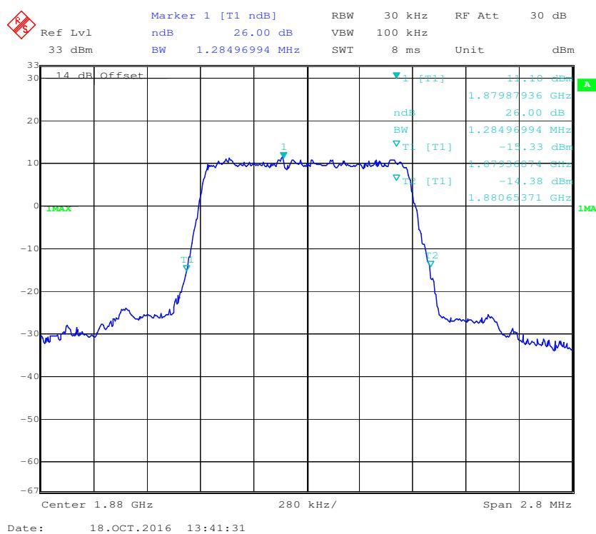
**16-QAM (1.4 MHz) - 26 dB Bandwidth, Middle channel**
