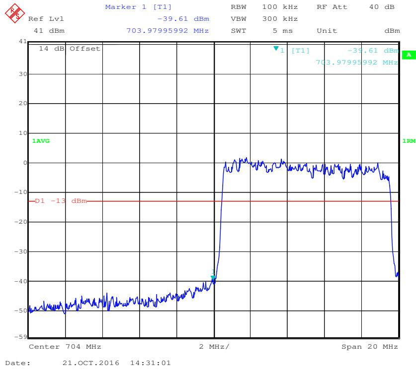
**QPSK (10.0 MHz, FULL RB) - Right Band Edge**
