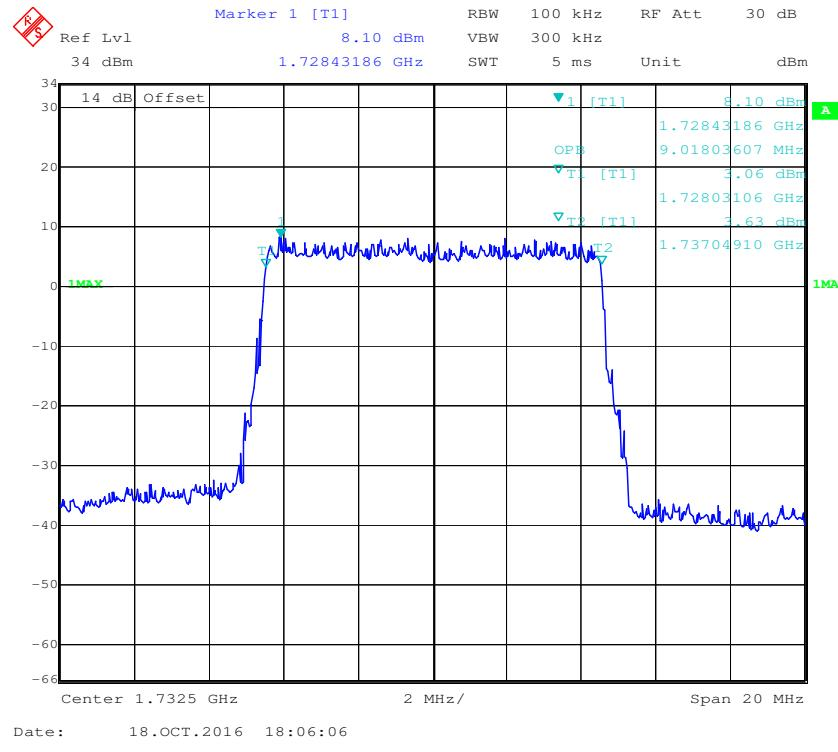
**16-QAM (10.0 MHz) - 99% Occupied Bandwidth, Middle channel**
