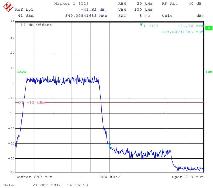
**QPSK (3.0 MHz, FULL RB) - Left Band Edge**
