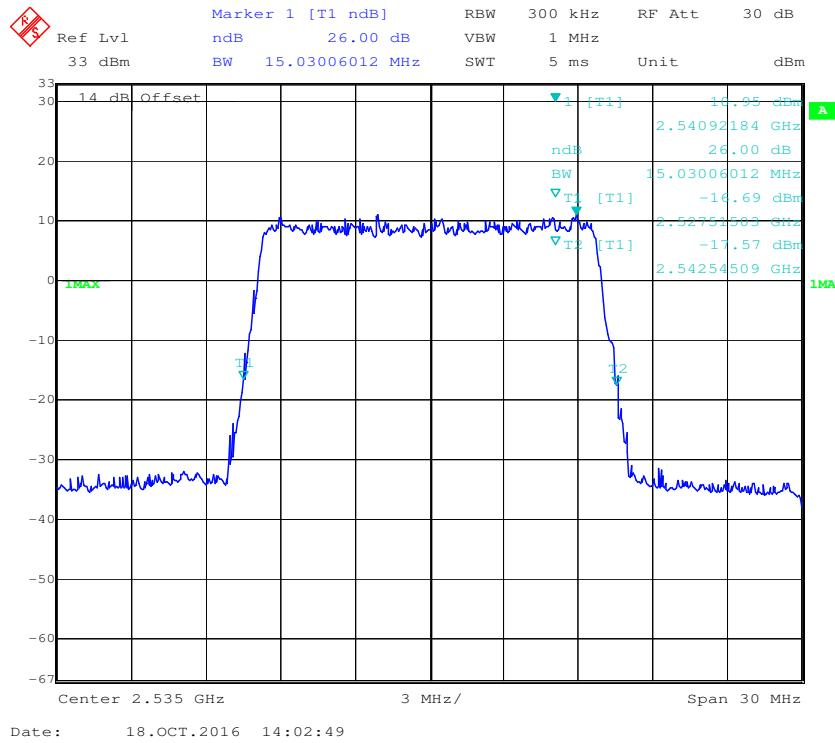
**QPSK (3.0 MHz) -26 dB Bandwidth, Middle channel**
