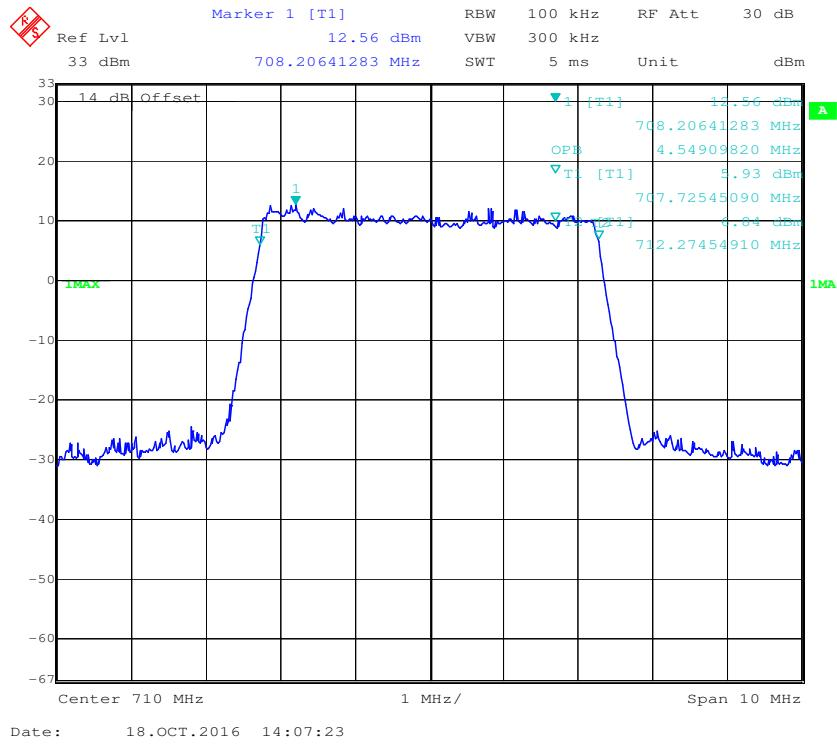
**QPSK (10.0 MHz) - 99% Occupied Bandwidth, Middle channel**
