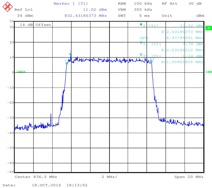
**16-QAM (10.0 MHz) -99% Occupied Bandwidth, Middle channel**
