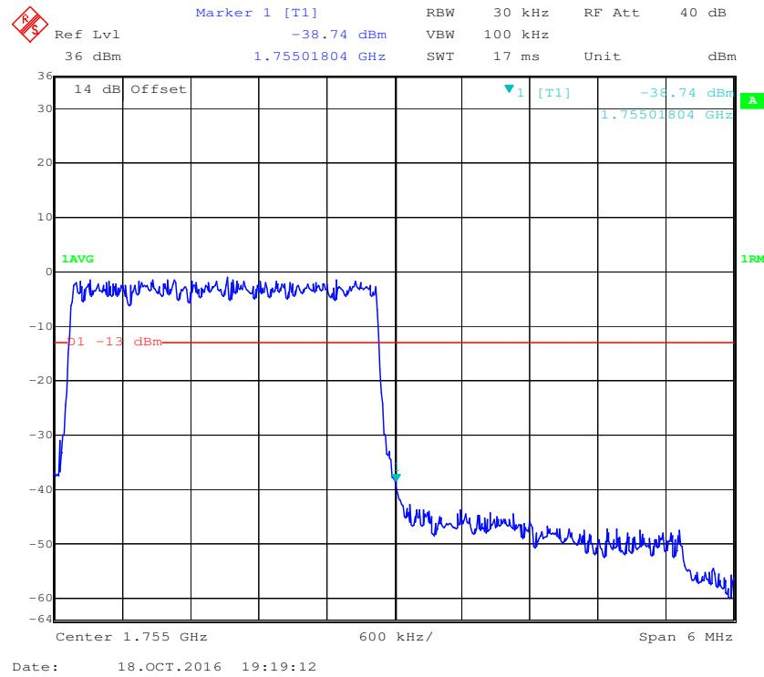
**16-QAM (3.0 MHz, FULL RB) - Left Band Edge**
