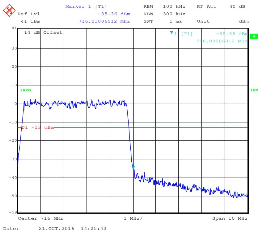
**16-QAM (5.0 MHz, FULL RB) - Left Band Edge**
