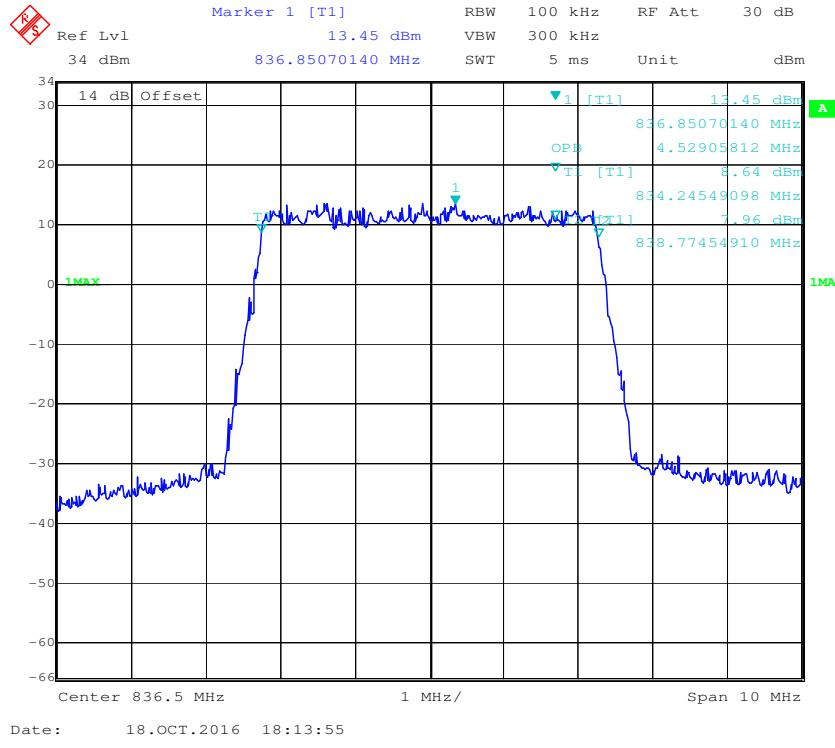
**QPSK (10.0 MHz) -99% Occupied Bandwidth, Middle channel**
