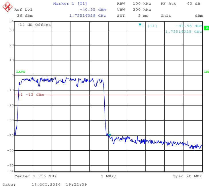
**QPSK (15.0 MHz, FULL RB) - Left Band Edge**
