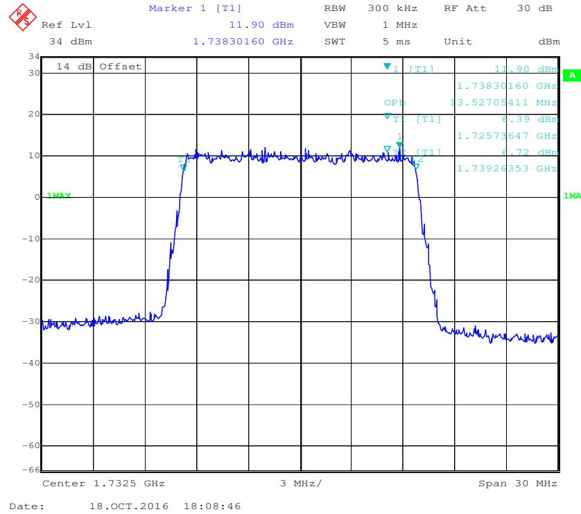
**QPSK (20.0 MHz) - 99% Occupied Bandwidth, Middle channel**
