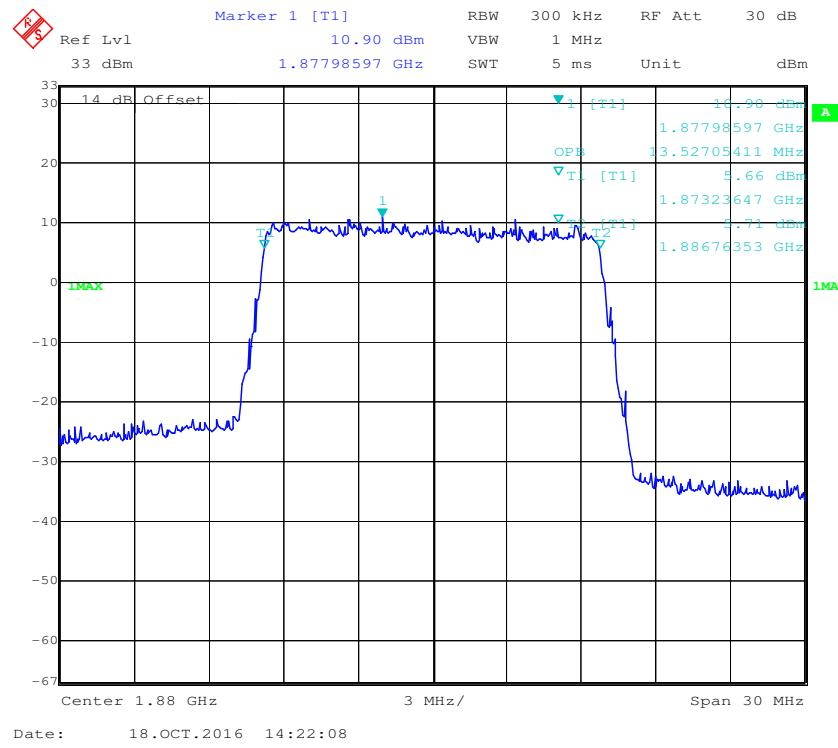
**QPSK (20.0 MHz) - 99% Occupied Bandwidth, Middle channel**
