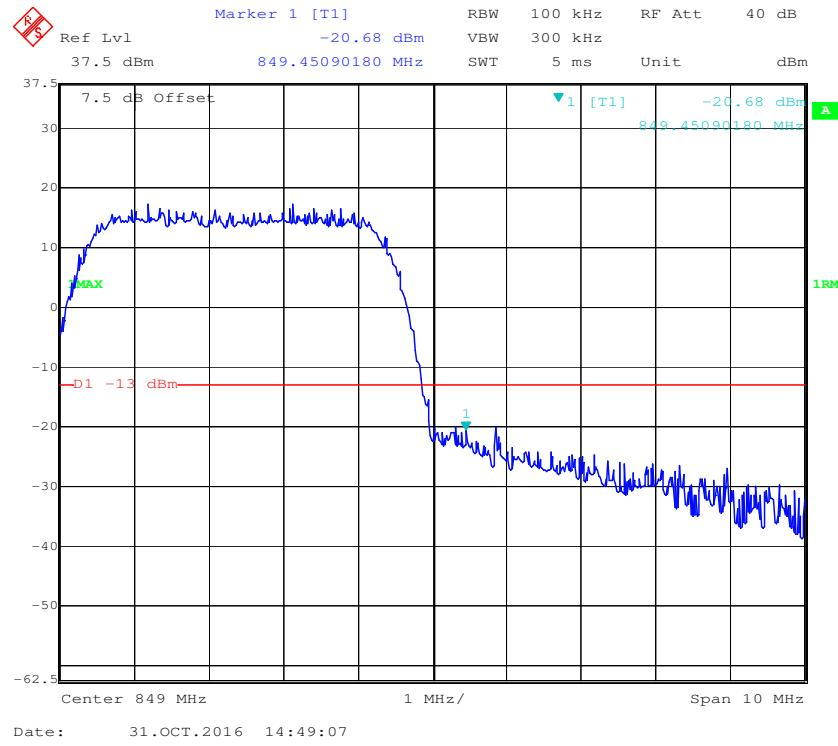
**PCS Band, Left Band Edge for GSM (GMSK) Mode**
