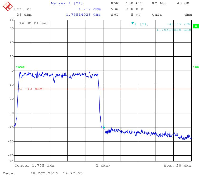
**16-QAM (10.0 MHz, FULL RB) - Left Band Edge**
