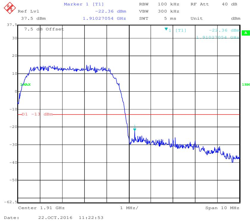
**Band 2:****QPSK (1.4 MHz, FULL RB) - Left Band Edge**
