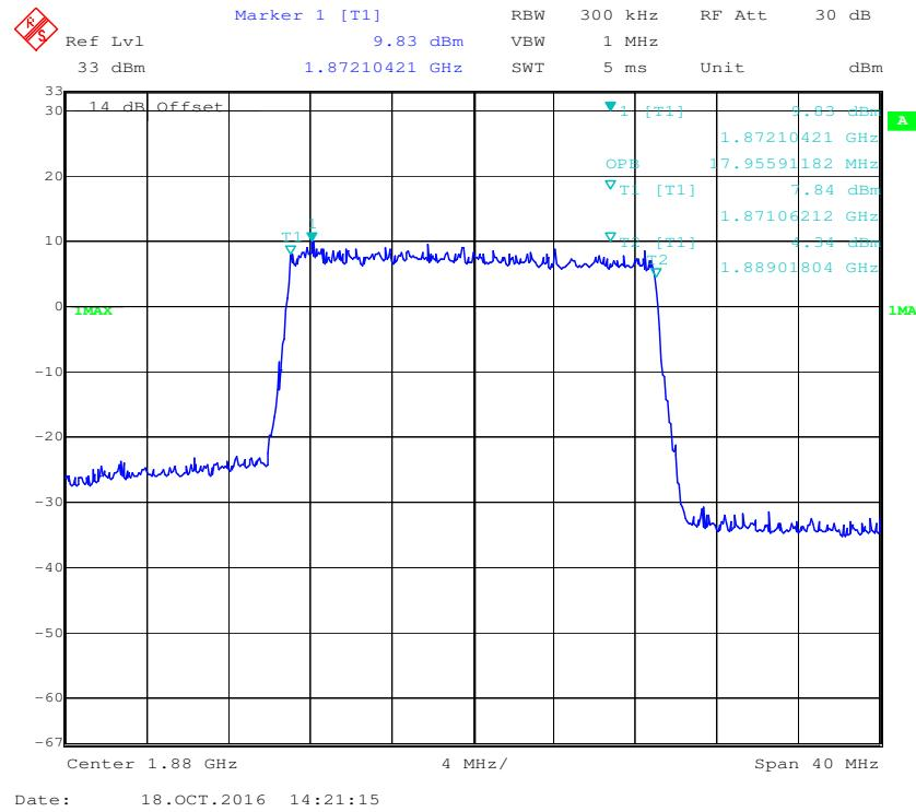
**16-QAM (20.0 MHz) - 99% Occupied Bandwidth, Middle channel**
