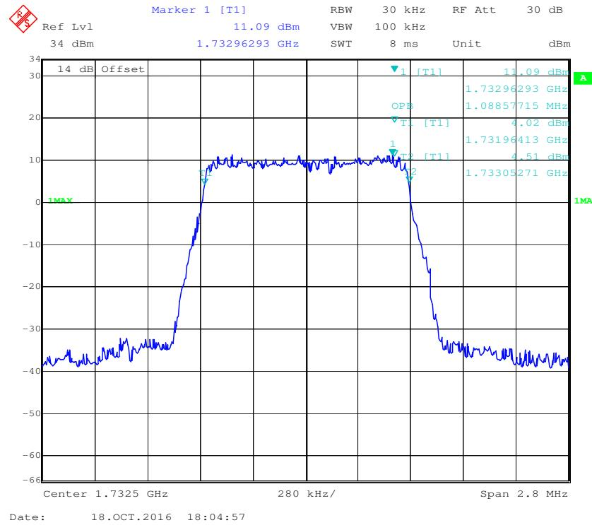
**QPSK (3.0 MHz) - 99% Occupied Bandwidth, Middle channel**
