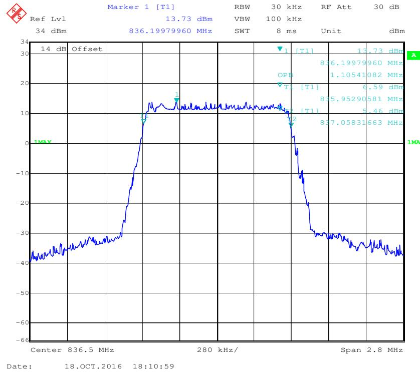
**QPSK (3.0 MHz) -99% Occupied Bandwidth, Middle channel**
