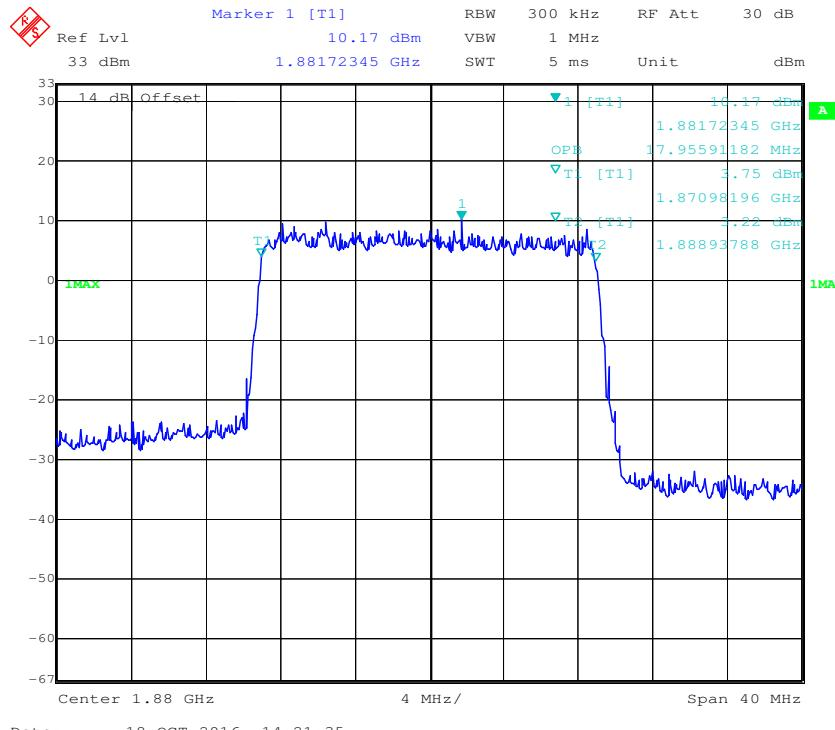
**QPSK (1.4 MHz) - 26 dB Bandwidth, Middle channel**
