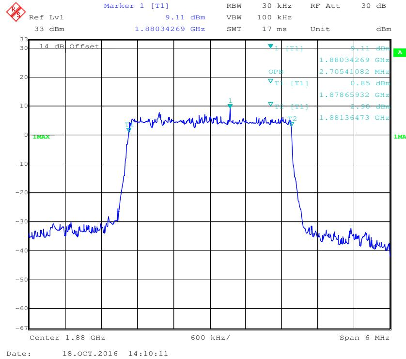
**16-QAM (3.0 MHz) - 99% Occupied Bandwidth, Middle channel**
