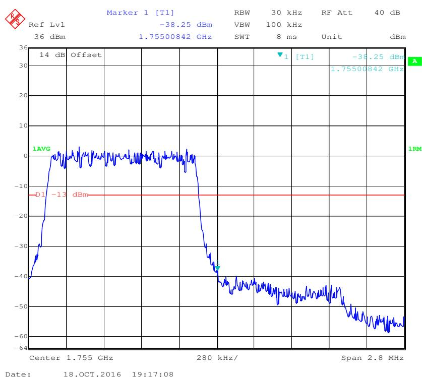
**16-QAM (1.4 MHz, FULL RB) - Left Band Edge**
