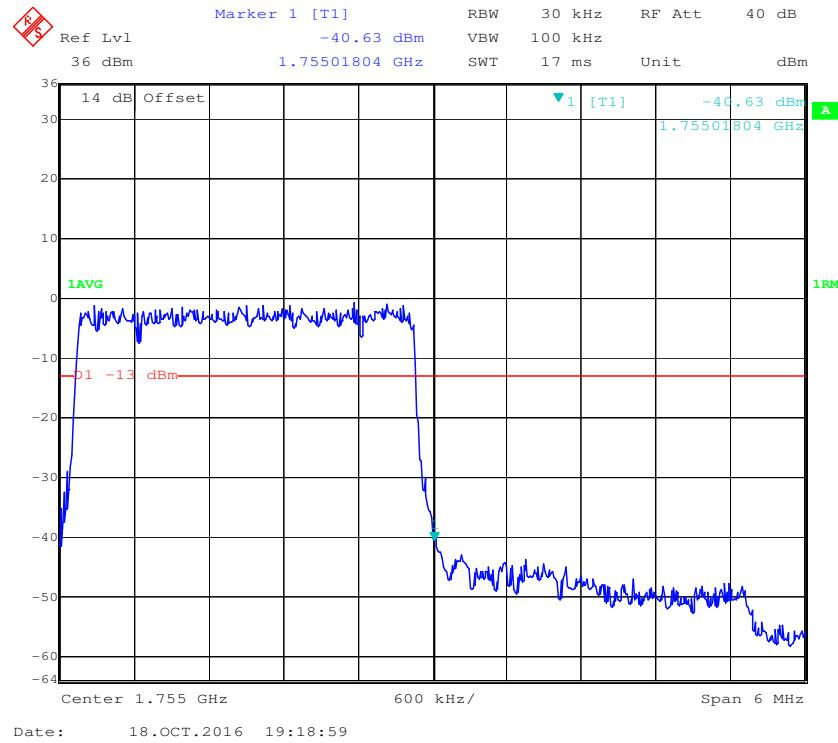
**QPSK (5.0 MHz, FULL RB) - Left Band Edge**
