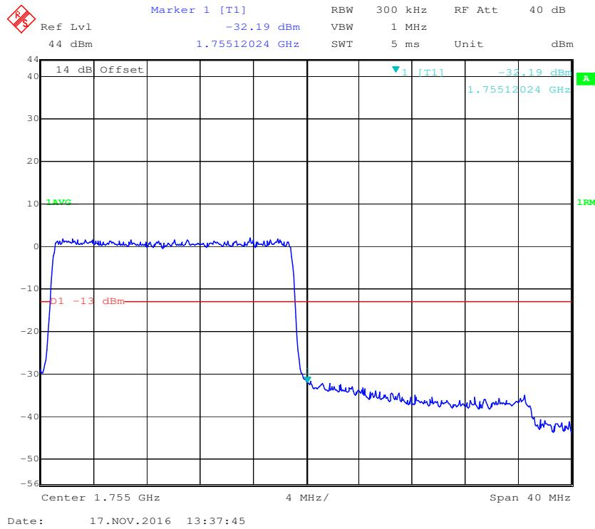
**16-QAM (20.0 MHz, FULL RB) - Left Band Edge**
