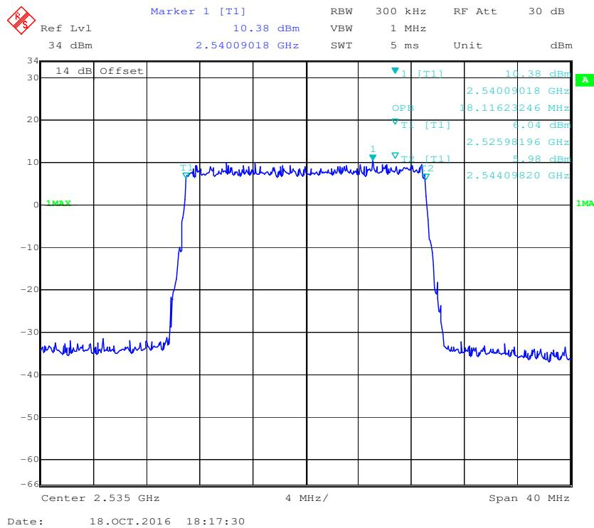
**QPSK (5.0 MHz) - 26 dB Bandwidth, Middle channel**
