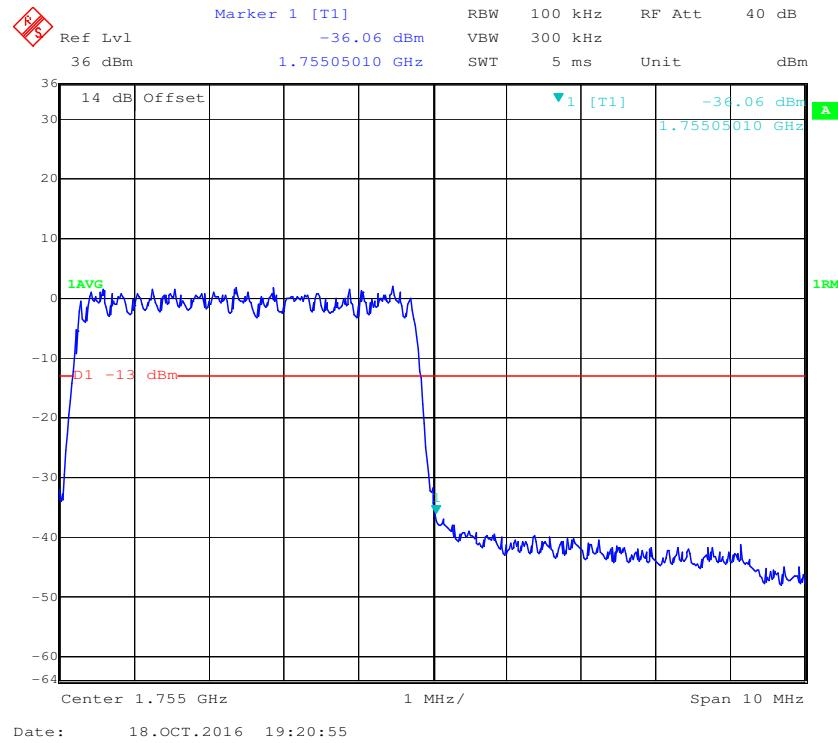
**16-QAM (5.0 MHz, FULL RB) - Left Band Edge**
