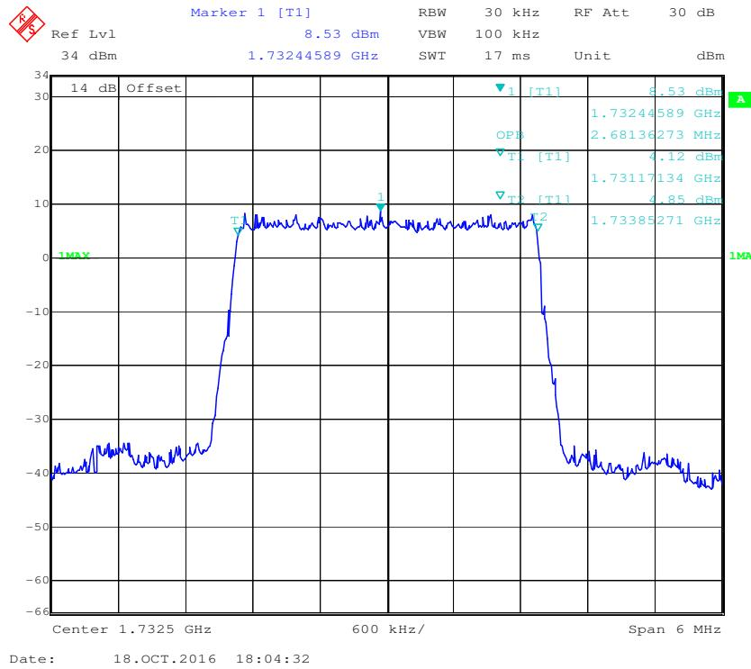
**QPSK (5.0 MHz) - 99% Occupied Bandwidth, Middle channel**
