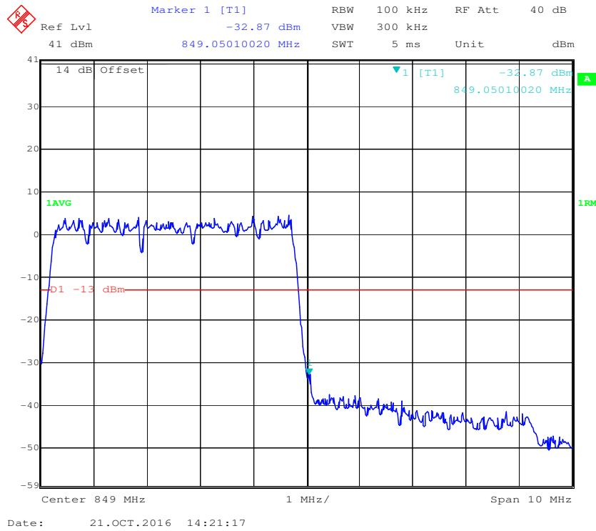
**16-QAM (5.0 MHz, FULL RB) - Left Band Edge**
