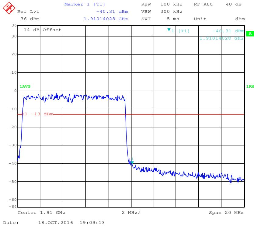
**16-QAM (10.0 MHz, FULL RB) - Left Band Edge**
