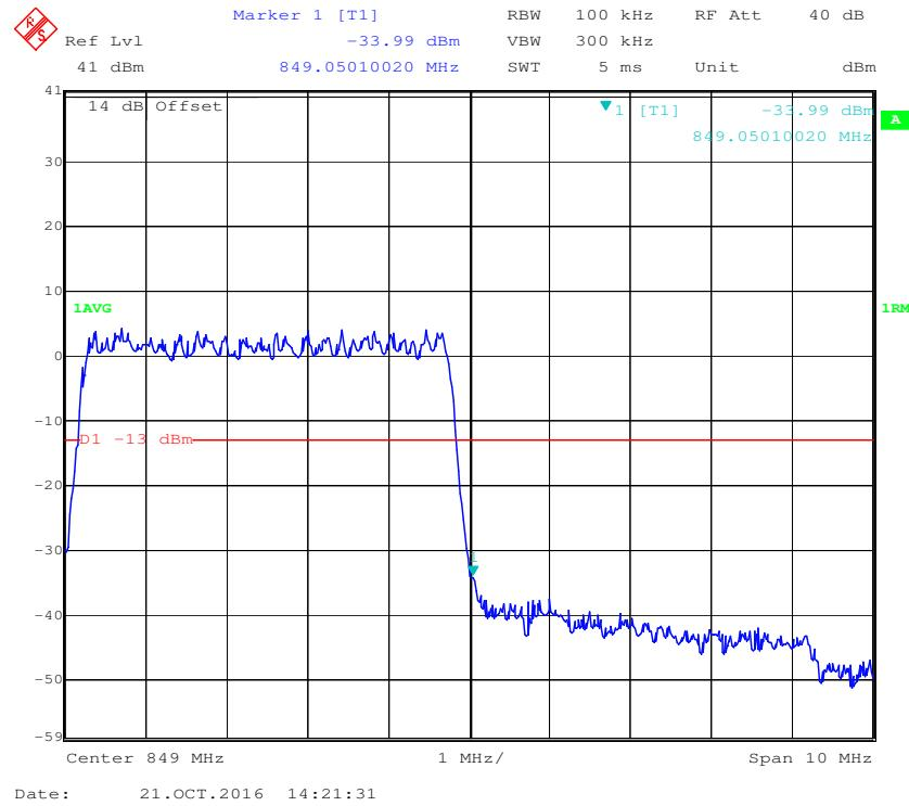
**QPSK (10.0 MHz, FULL RB) - Left Band Edge**
