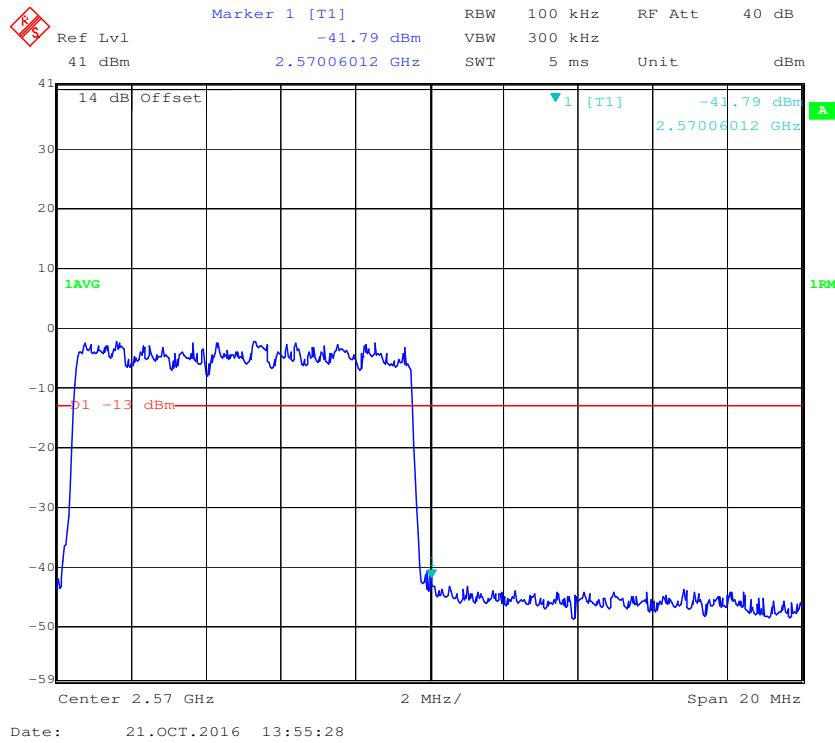
**16-QAM (10.0 MHz, FULL RB) - Left Band Edge**
