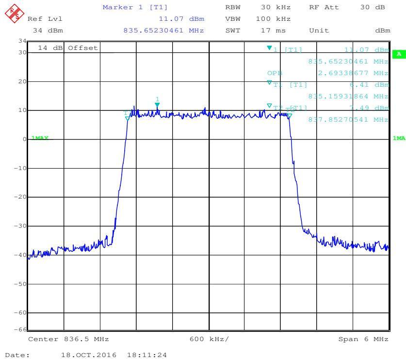
**QPSK (5.0 MHz) - 99% Occupied Bandwidth, Middle channel**
