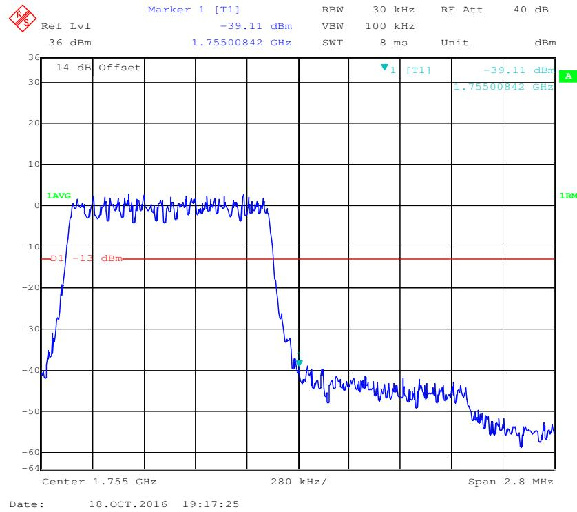
**QPSK (3.0 MHz, FULL RB) - Left Band Edge**
