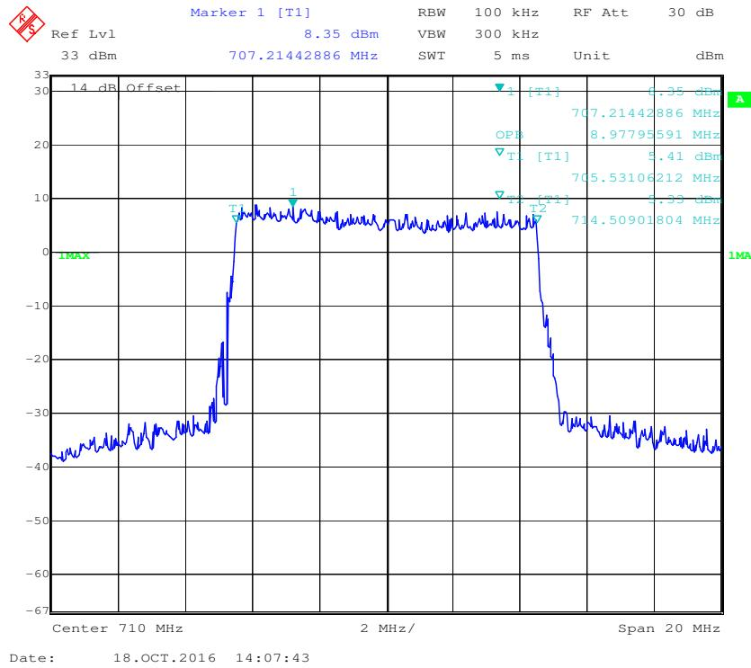
**QPSK (5.0 MHz) - 26 dB Bandwidth, Middle channel**
