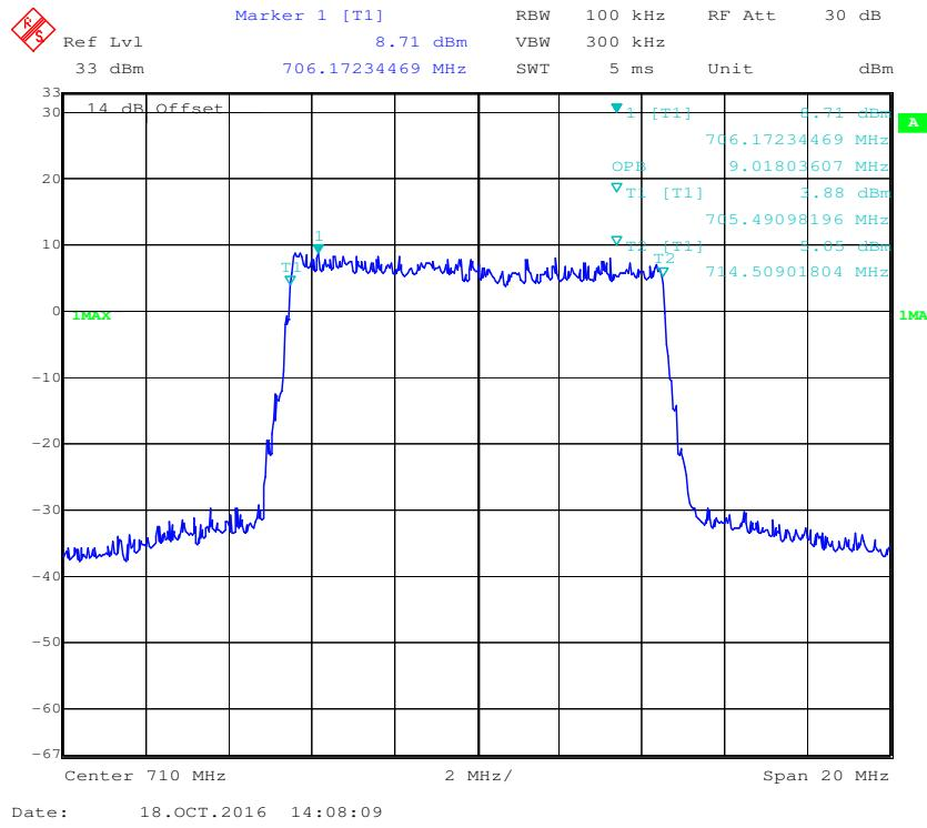
**16-QAM (10.0MHz) - 99% Occupied Bandwidth, Middle channel**
