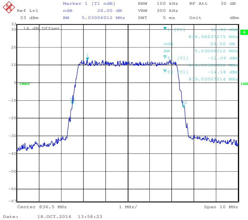
**QPSK (10.0 MHz) -26 dB Bandwidth, Middle channel**
