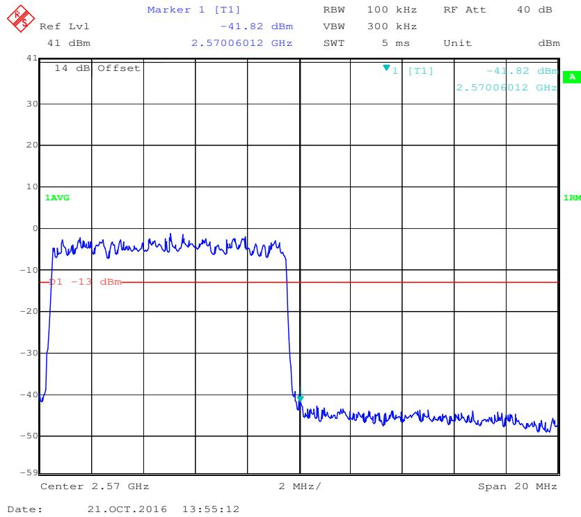
**QPSK (15.0 MHz, FULL RB) - Left Band Edge**
