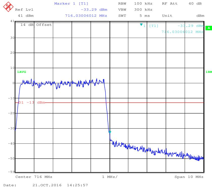
**QPSK (10.0 MHz, FULL RB) - Left Band Edge**
