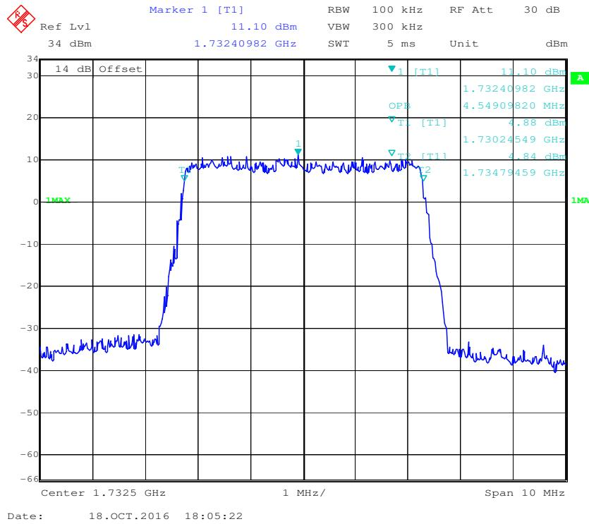
**QPSK (10.0 MHz) - 99% Occupied Bandwidth, Middle channel**
