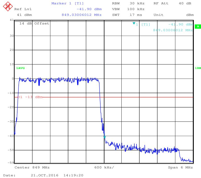
**16-QAM (3.0 MHz, FULL RB) - Left Band Edge**
