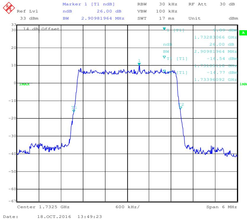
**QPSK (5.0 MHz) - 26 dB Bandwidth, Middle channel**
