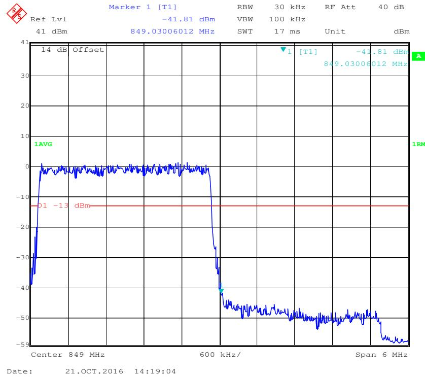
**QPSK (5.0 MHz, FULL RB) - Left Band Edge**
