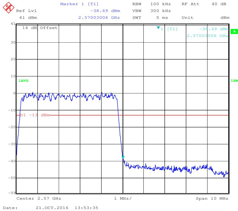
**QPSK (10.0 MHz, FULL RB) - Left Band Edge**
