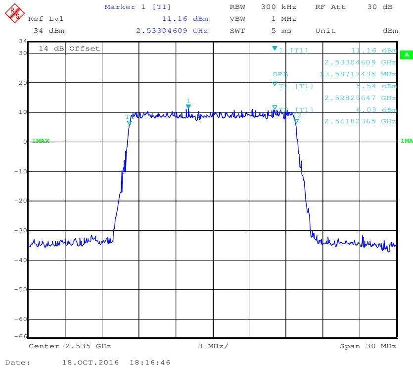
**16-QAM (15.0 MHz) -99% Occupied Bandwidth, Middle channel**
