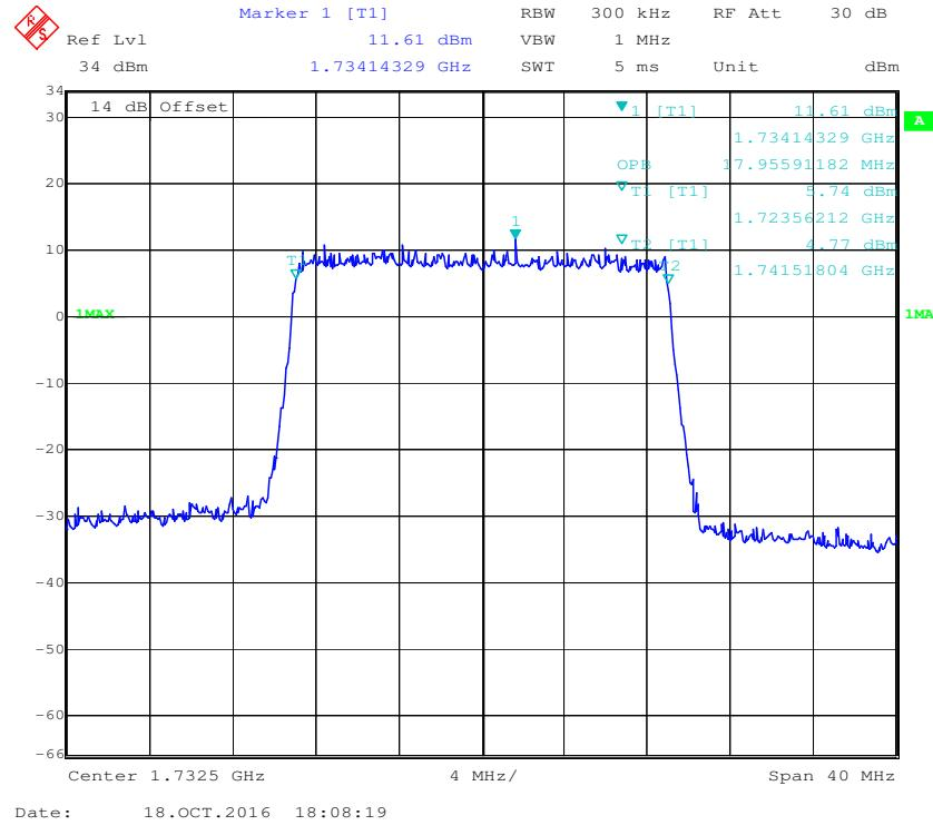
**QPSK (1.4 MHz) - 26 dB Bandwidth, Middle channel**
