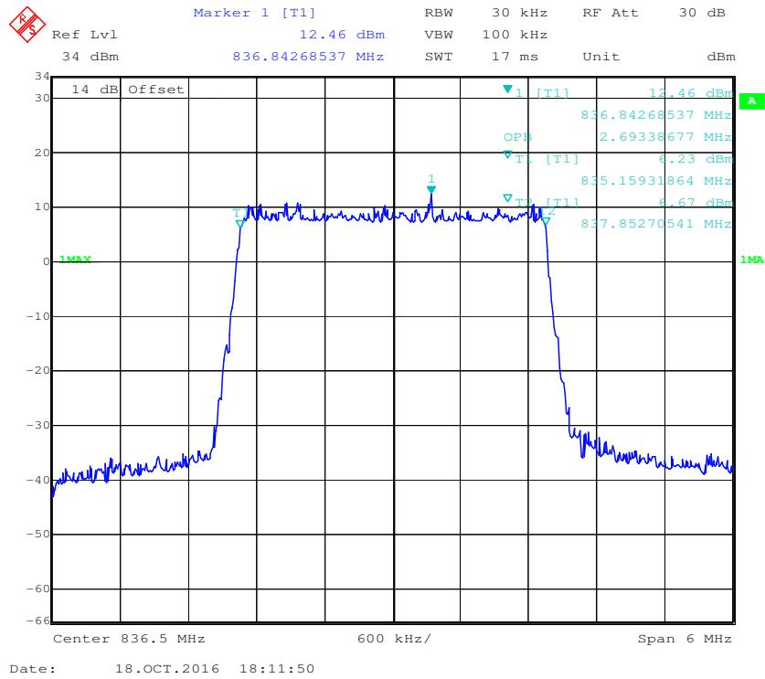
**16-QAM (3.0 MHz) - 99% Occupied Bandwidth, Middle channel**
