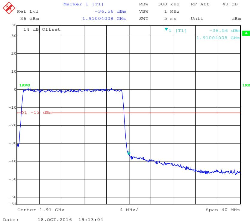
**Band 4:****QPSK (1.4 MHz, FULL RB) - Left Band Edge**
