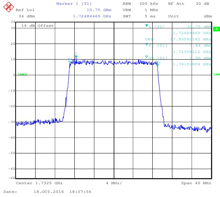
**16-QAM (20.0 MHz) - 99% Occupied Bandwidth, Middle channel**
