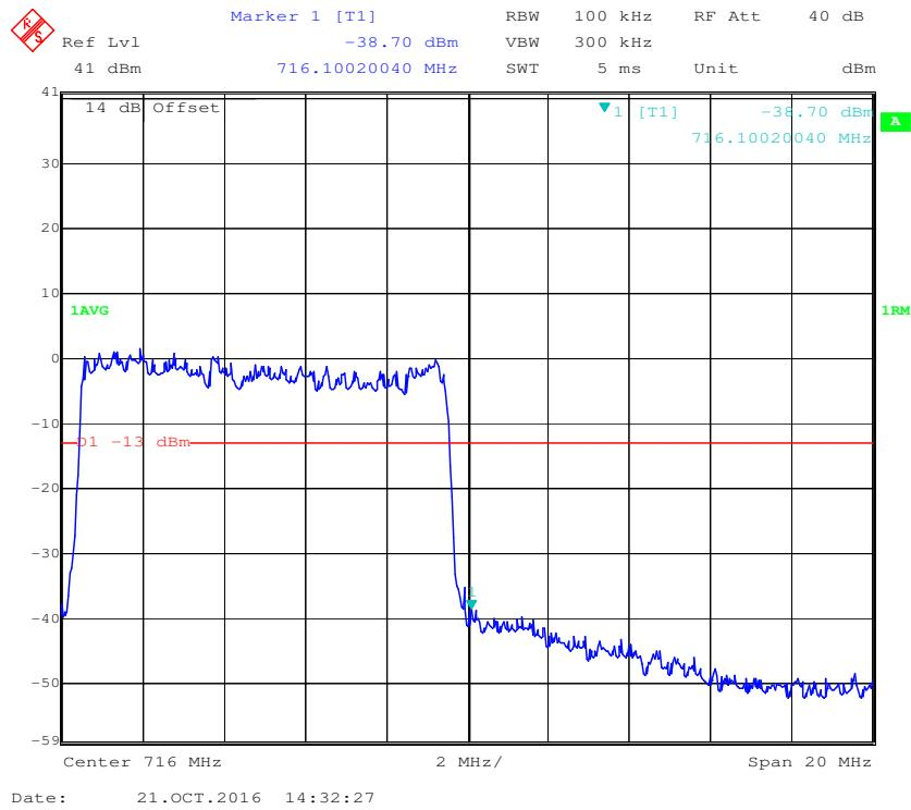
**16-QAM (10.0 MHz, FULL RB) - Left Band Edge**
