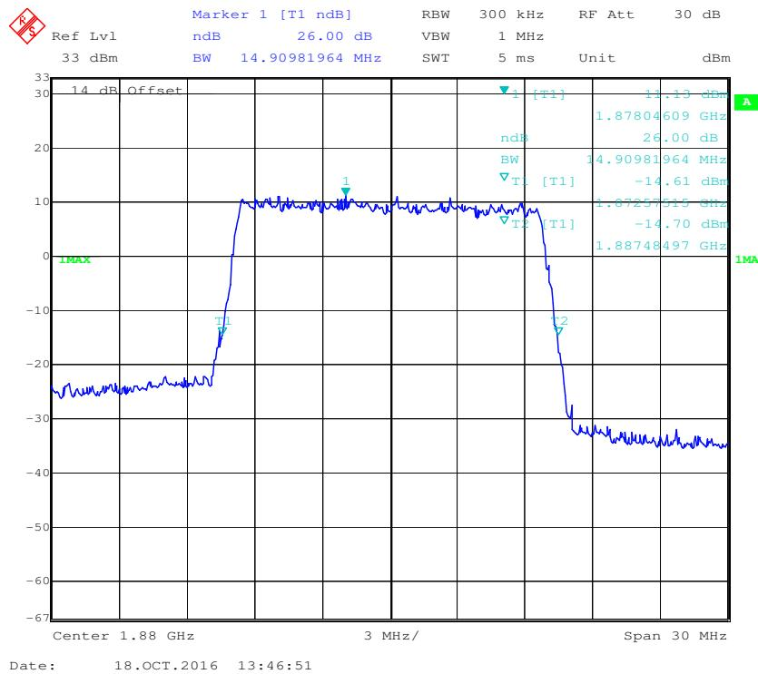
**16-QAM (15.0 MHz) - 26 dB Bandwidth, Middle channel**
