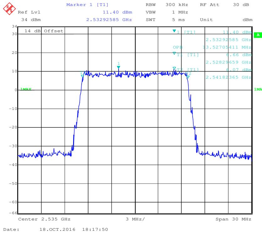
**QPSK (20.0 MHz) -99% Occupied Bandwidth, Middle channel**
