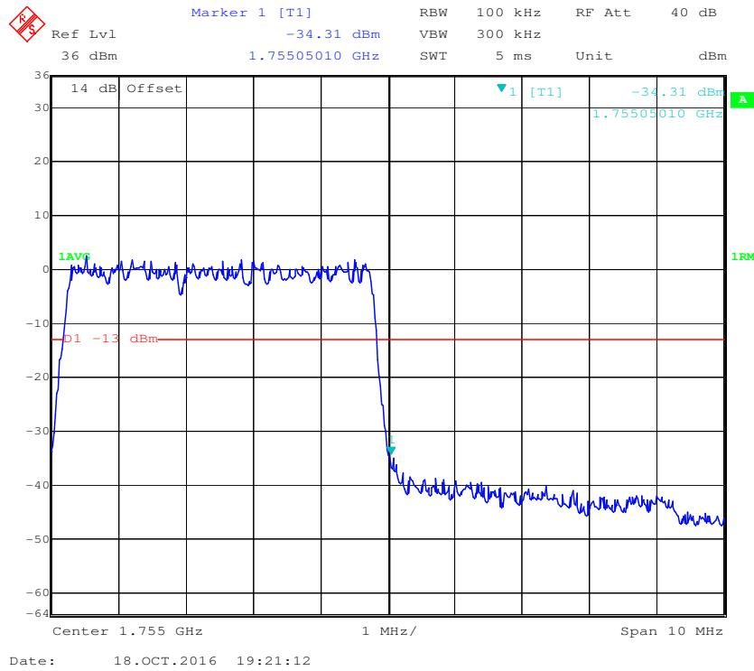
**QPSK (10.0 MHz, FULL RB) - Left Band Edge**
