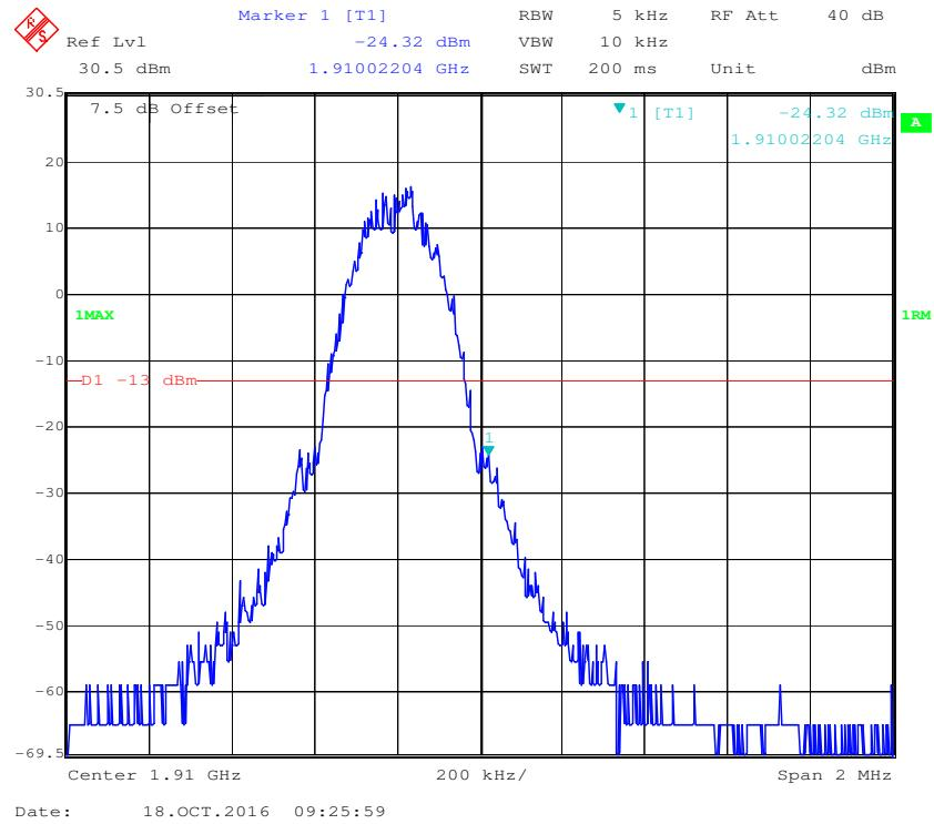
**PCS Band, Left Band Edge for RMC (BPSK) Mode**
