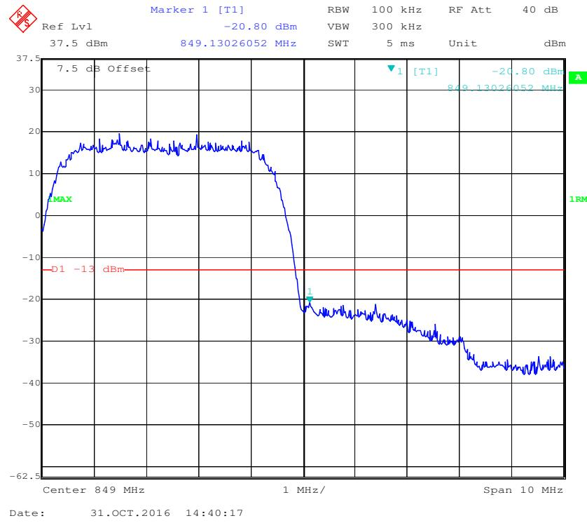
**Cellular Band, Left Band Edge for HSDPA (16QAM) Mode**
