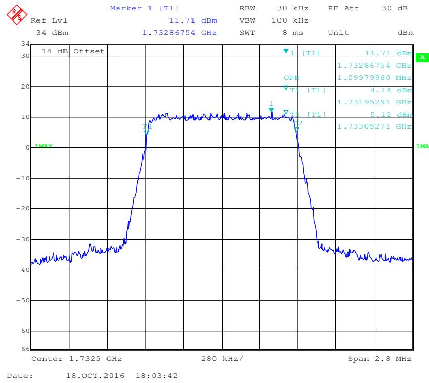
**16-QAM (1.4 MHz) - 99% Occupied Bandwidth, Middle channel**
