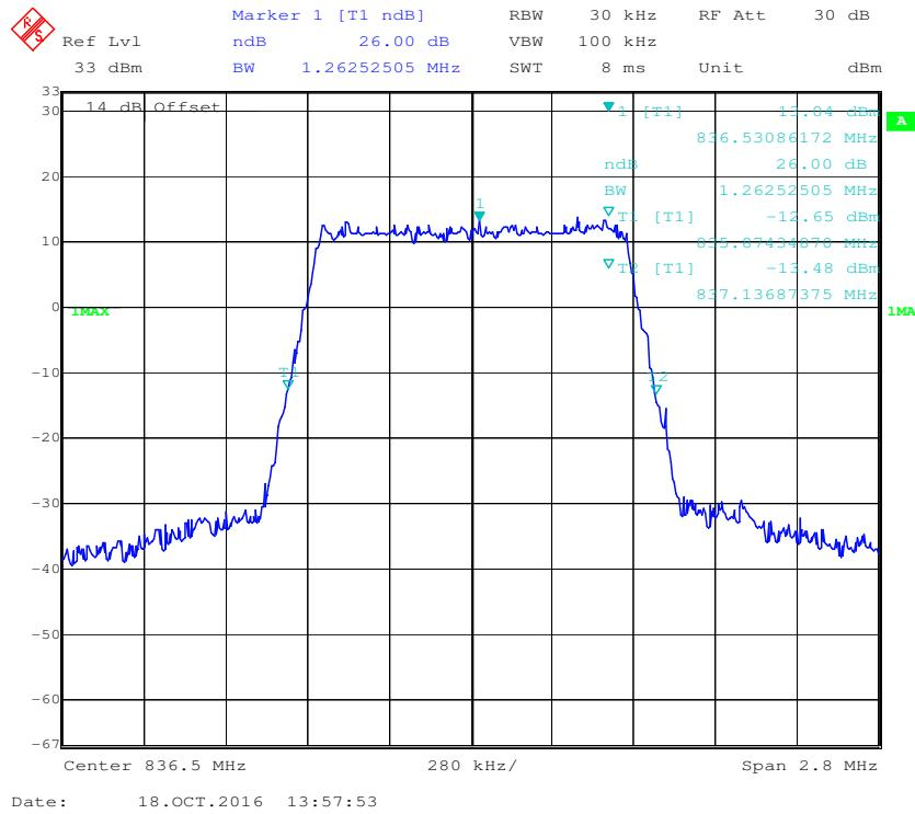
**QPSK (3.0 MHz) -26 dB Bandwidth, Middle channel**
