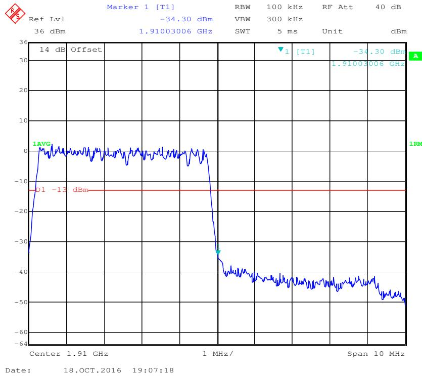
**QPSK (10.0 MHz, FULL RB) - Left Band Edge**
