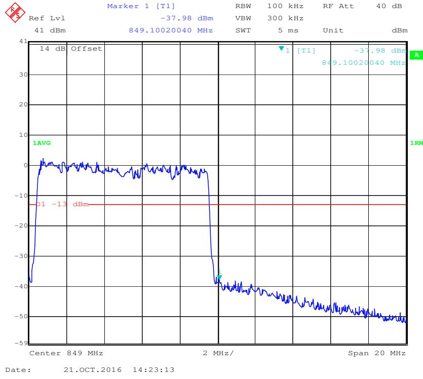
**Band 7:****QPSK (5.0 MHz, FULL RB) - Left Band Edge**
