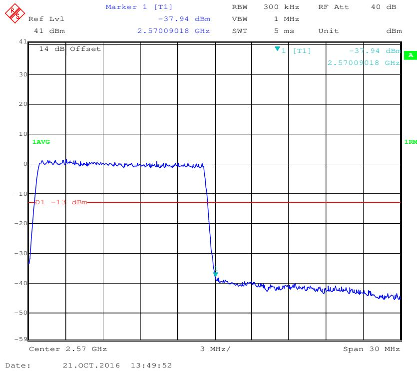
**16-QAM (15.0 MHz, FULL RB) - Left Band Edge**
