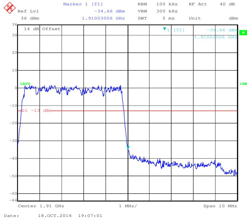
**16-QAM (5.0 MHz, FULL RB) - Left Band Edge**
