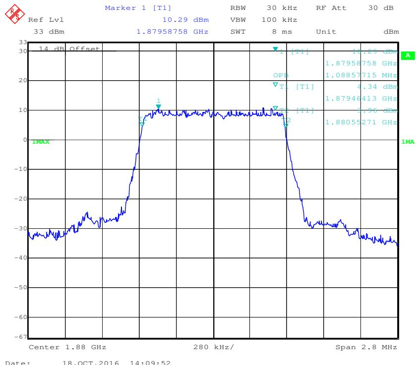
**16-QAM (1.4 MHz) - 99% Occupied Bandwidth, Middle channel**
