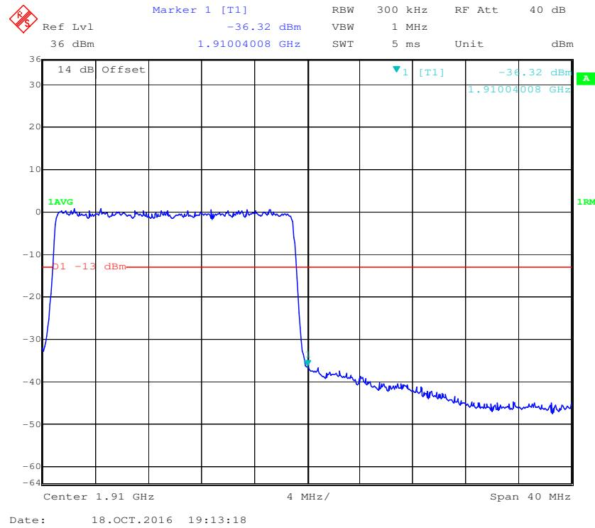
**16-QAM (20.0 MHz, FULL RB) - Left Band Edge**
