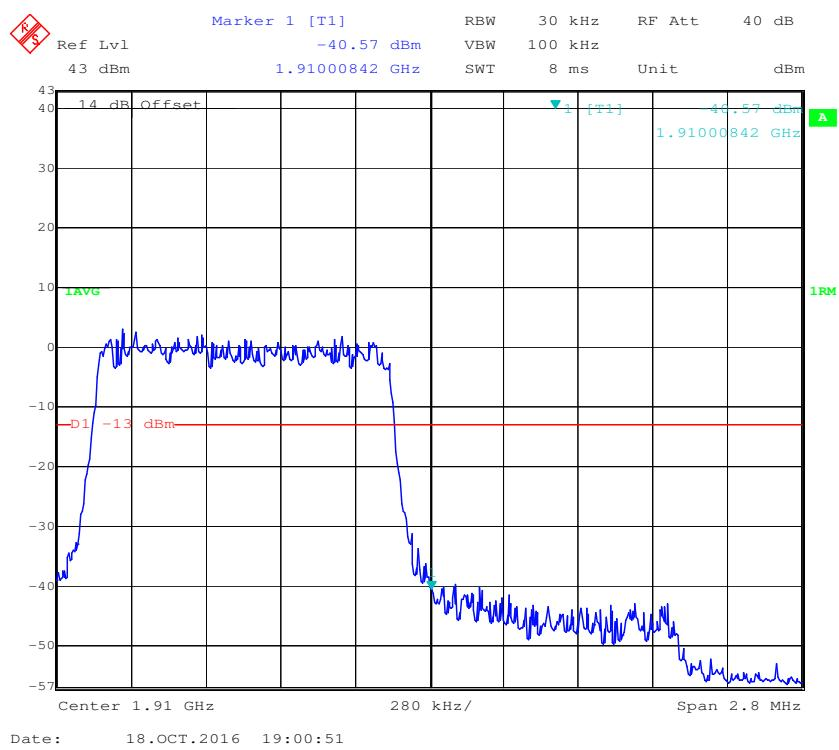
**16-QAM (1.4 MHz, FULL RB) - Left Band Edge**
