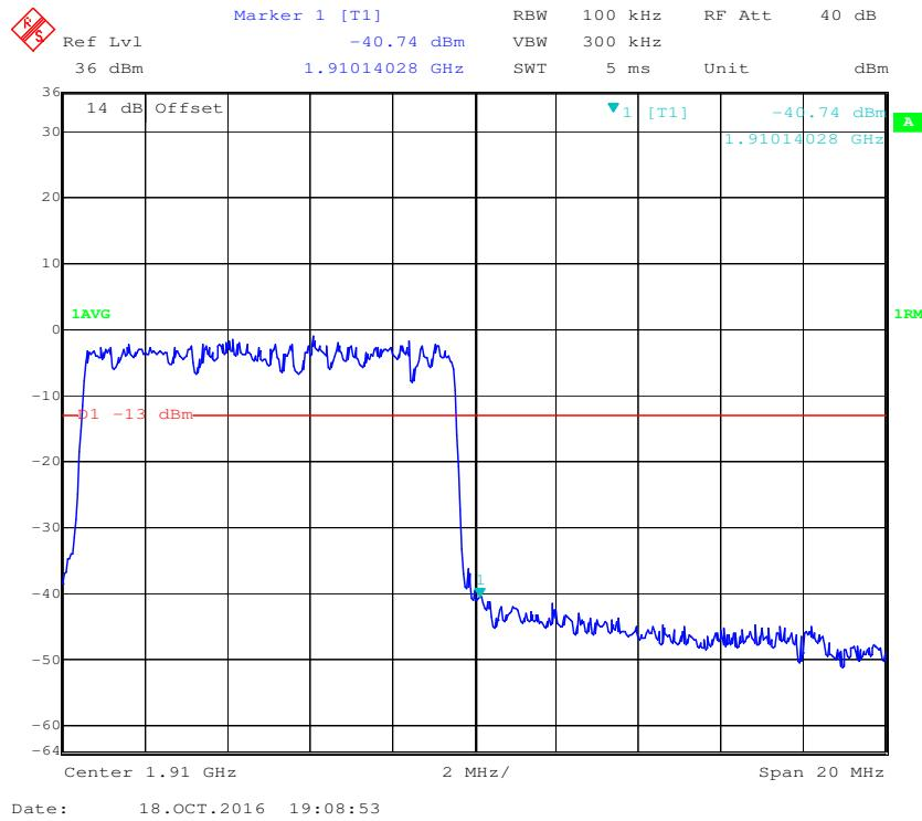
**QPSK (15.0 MHz, FULL RB) - Left Band Edge**
