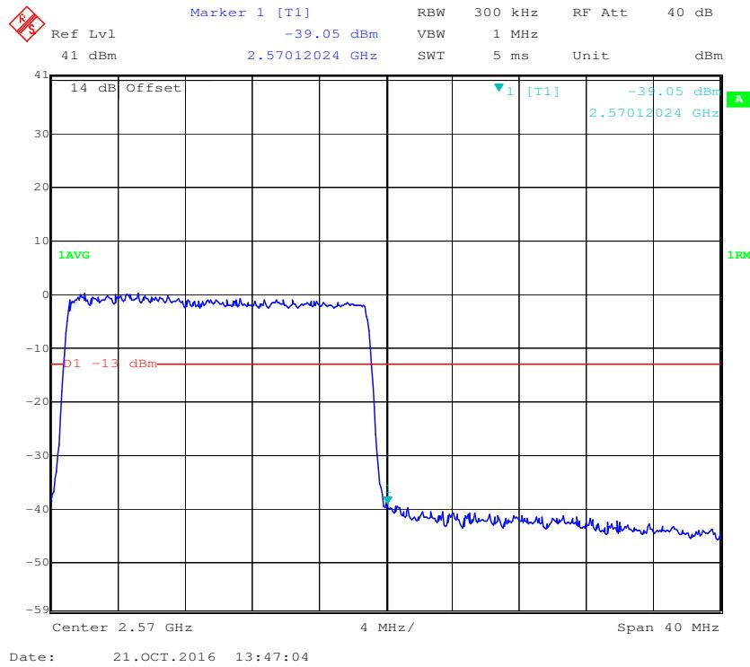
**Band 17:****QPSK (5.0 MHz, FULL RB) - Left Band Edge**
