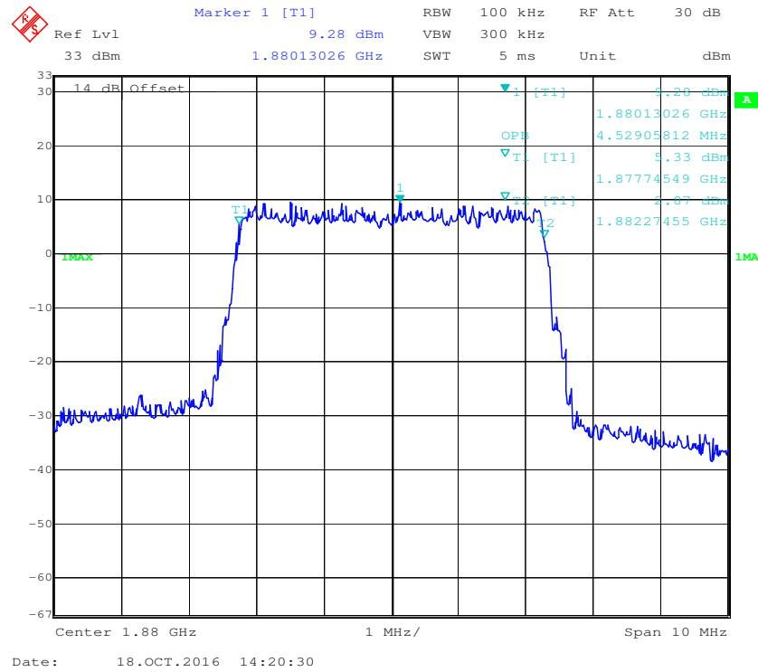
**16-QAM (5.0 MHz) - 99% Occupied Bandwidth, Middle channel**
