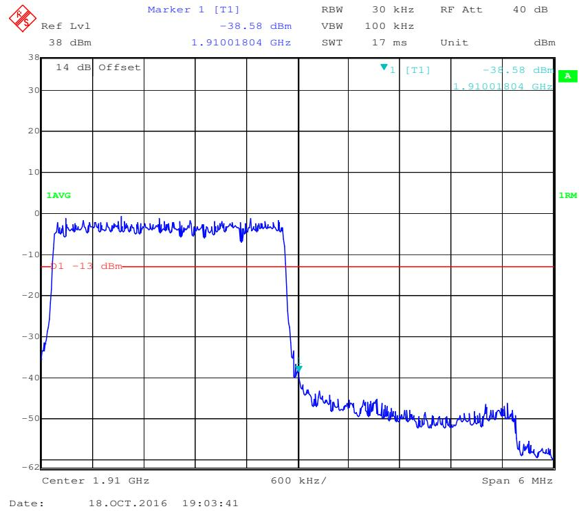
**QPSK (5.0 MHz, FULL RB) - Left Band Edge**
