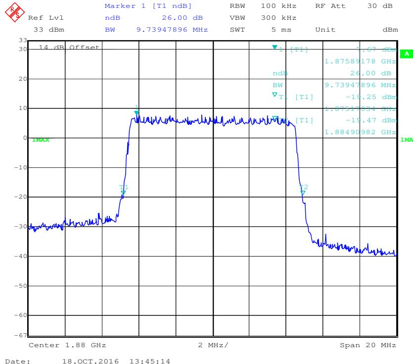
**16-QAM (10.0 MHz) - 26 dB Bandwidth, Middle channel**
