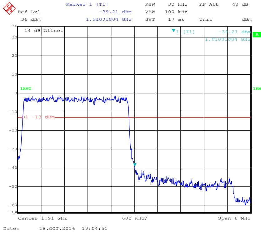
**16-QAM (3.0 MHz, FULL RB) - Left Band Edge**
