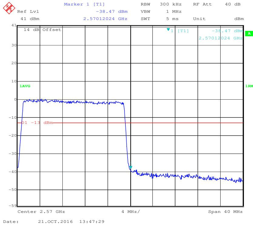
**16-QAM (20.0 MHz, FULL RB) - Left Band Edge**
