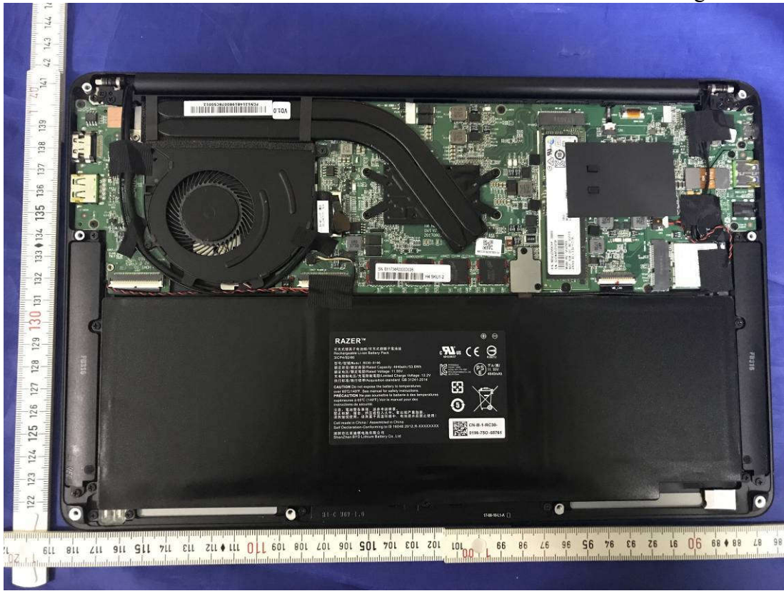
Figure 12 Inside Configuration of the EUT
