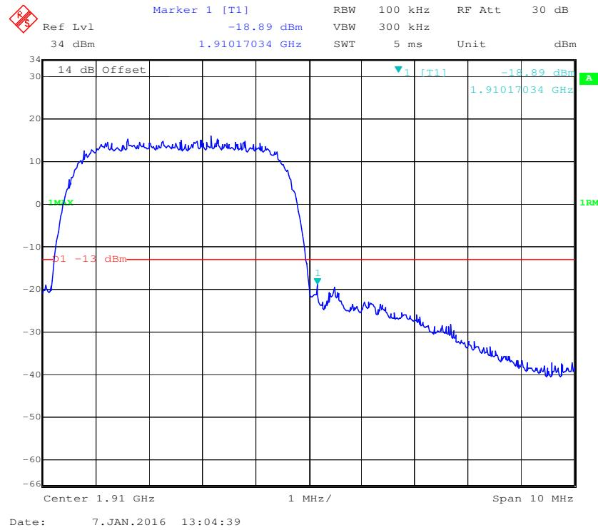
**PCS Band, Left Band Edge for HSDPA (16QAM) Mode**
