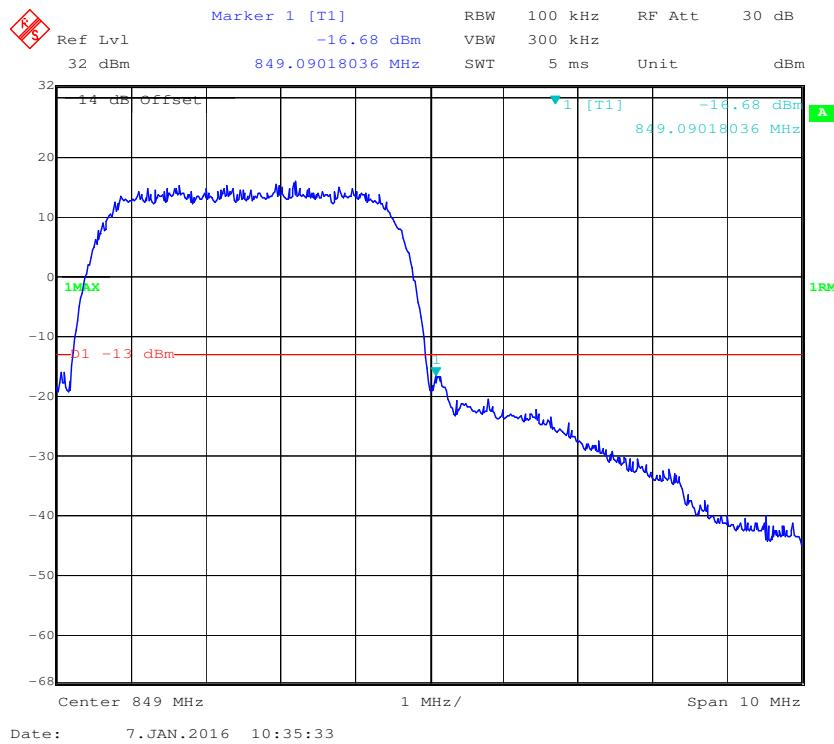
**Cellular Band, Left Band Edge for HSDPA (16QAM) Mode**
