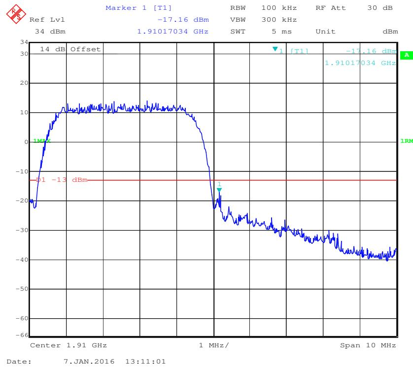
**PCS Band, Left Band Edge for HSUPA (BPSK) Mode**
