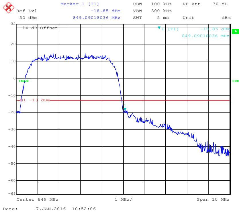
**Cellular Band, Left Band Edge for HSUPA (BPSK) Mode**
