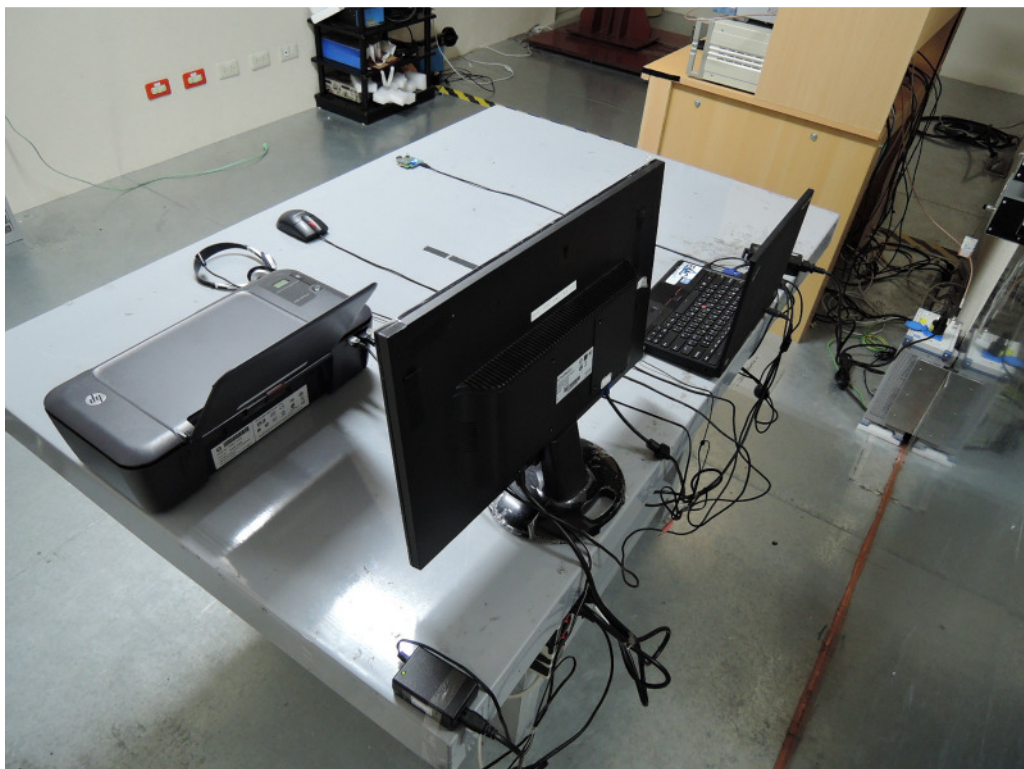
Photograph 5: Set-up for for Mains Conducted testing Back
