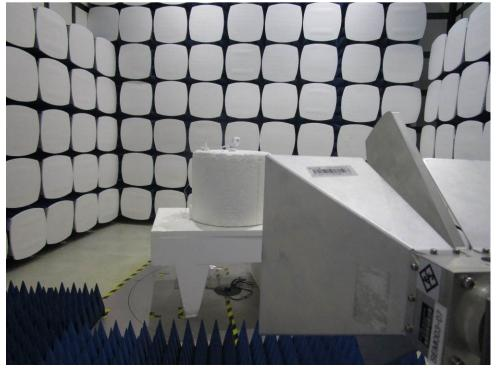
1.3 Radiated Spurious Emissions Test Setup
