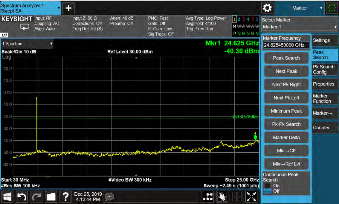
Figure 58: Conducted Spurious Emission & Authorized-band band-edge, 802.11n(HT20), 2437MHz Carrier Level
