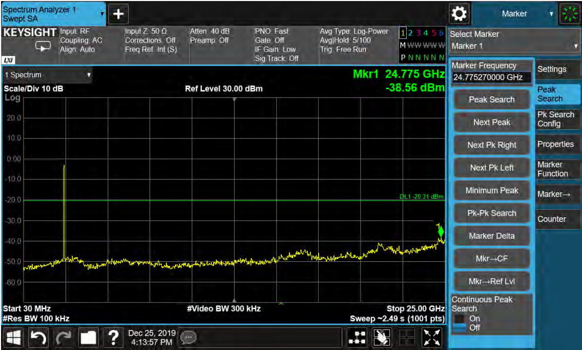
Figure 59: Conducted Spurious Emission & Authorized-band band-edge, 802.11n(HT20), 2462MHz Carrier Level
