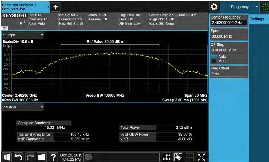
Figure 15: 6dB Bandwidth and 99% Bandwidth, 802.11b, 2462MHz
