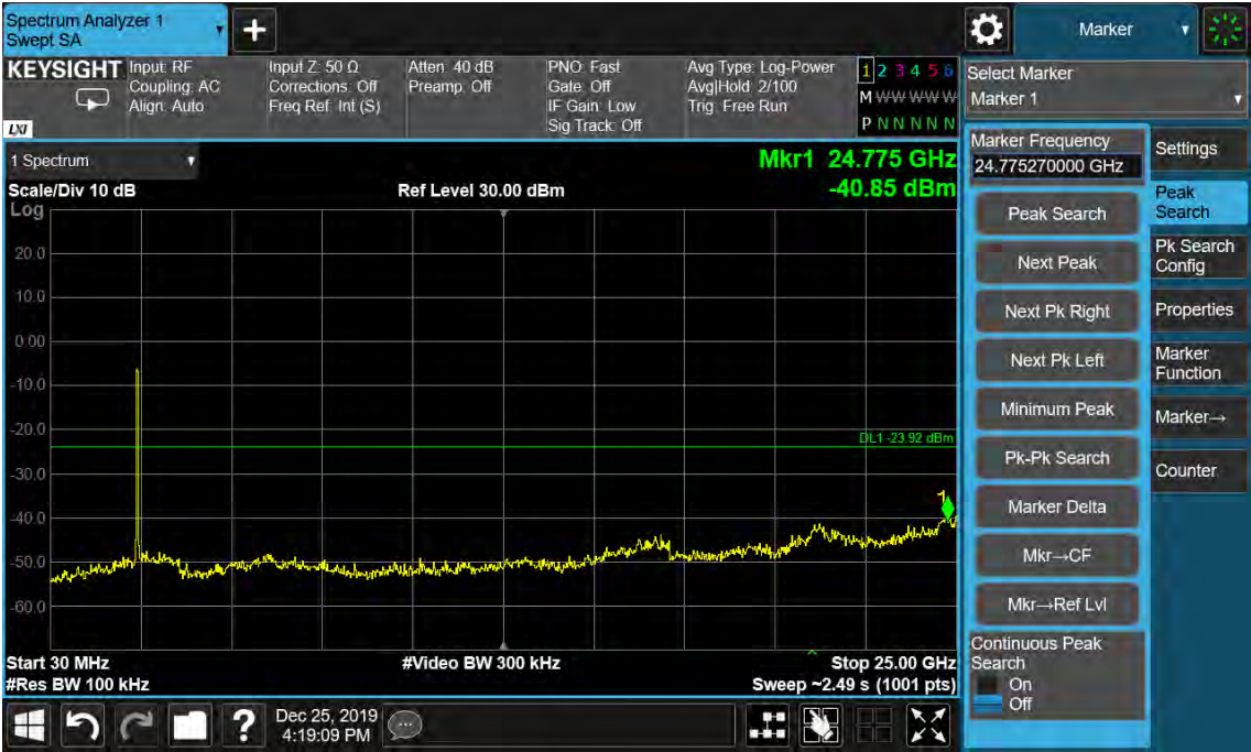
Figure 63: Conducted Spurious Emission & Authorized-band band-edge, 802.11n(HT40), 2452MHz Carrier Level
