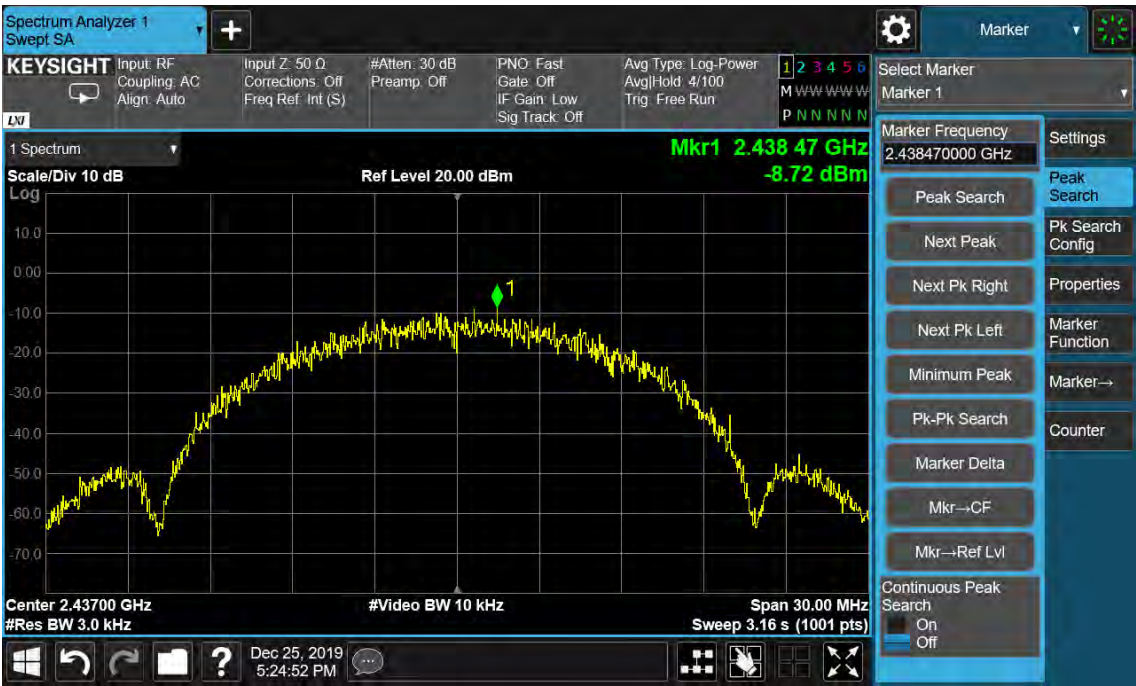
Figure 38: Power Spectral Density, 802.11b, 2437MHz
