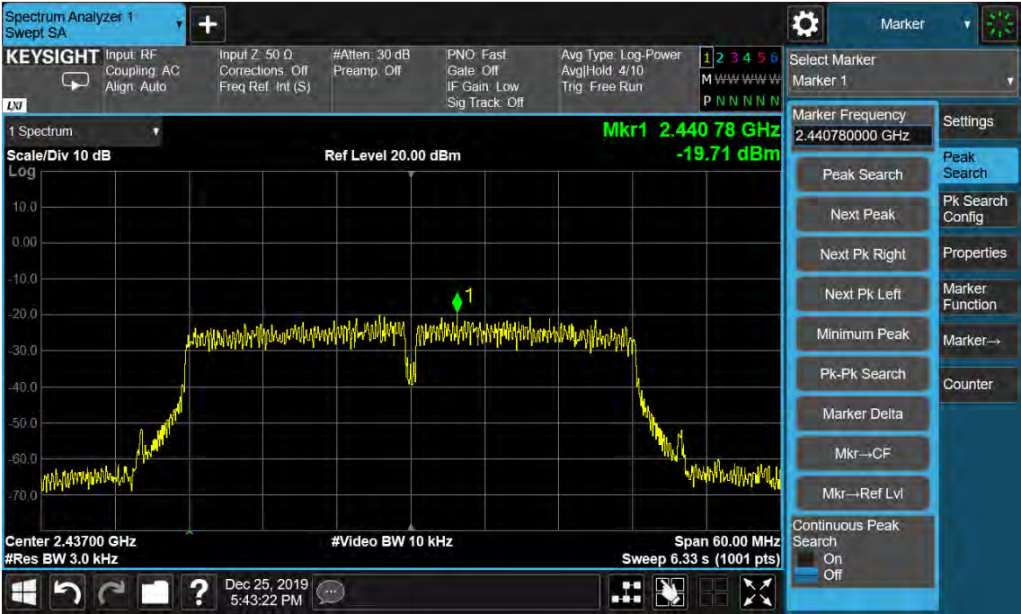
Figure 47: Power Spectral Density, 802.11n(HT40), 2437MHz
