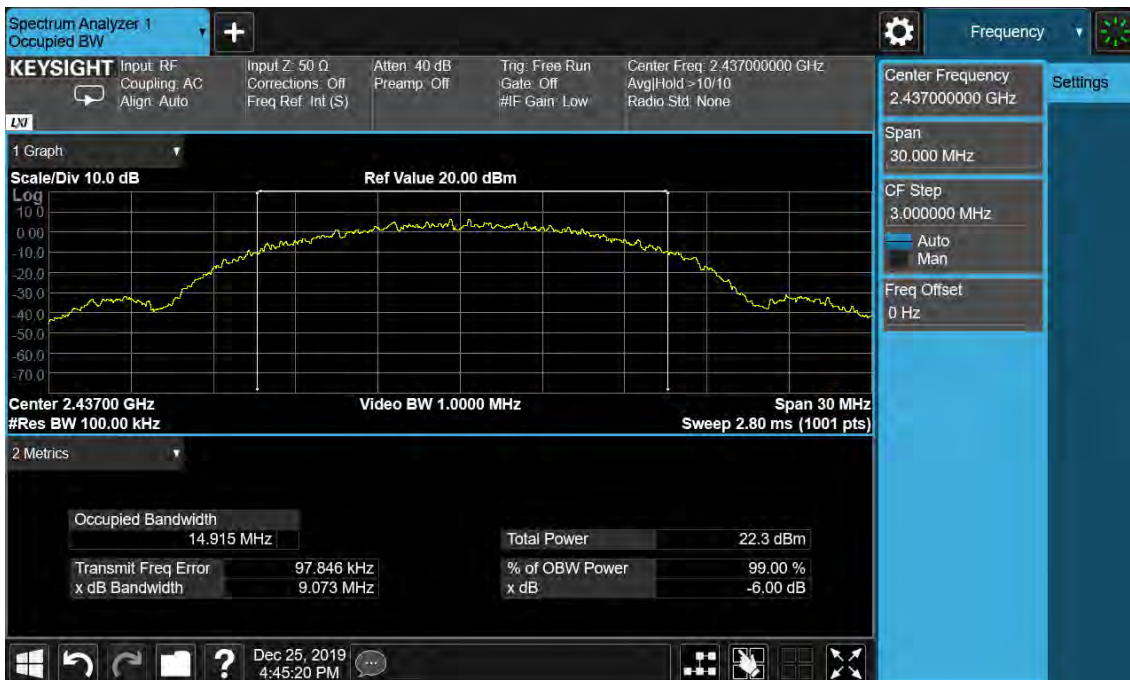
Figure 14: 6dB Bandwidth and 99% Bandwidth, 802.11b, 2437MHz
