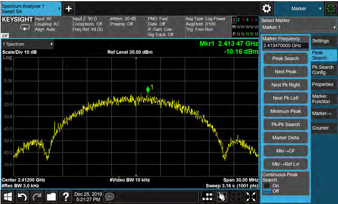
Figure 8: Power Spectral Density, 802.11b, 2422MHz
