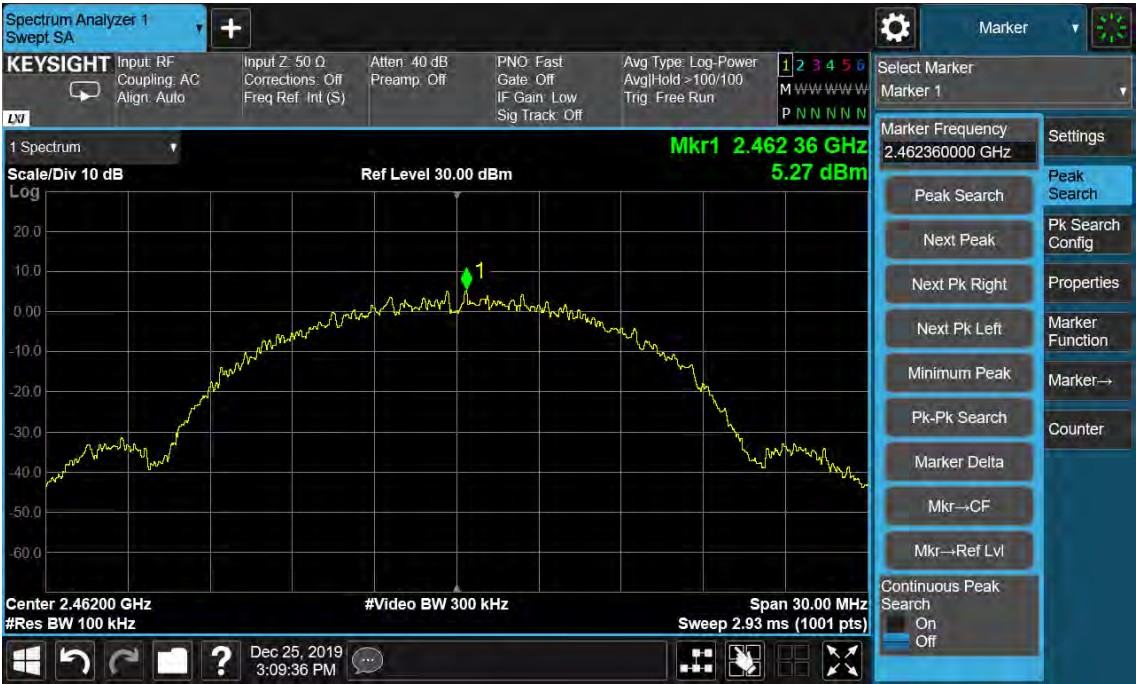
Figure 51: Conducted Spurious Emission & Authorized-band band-edge, 802.11b, 2462MHz Carrier Level
