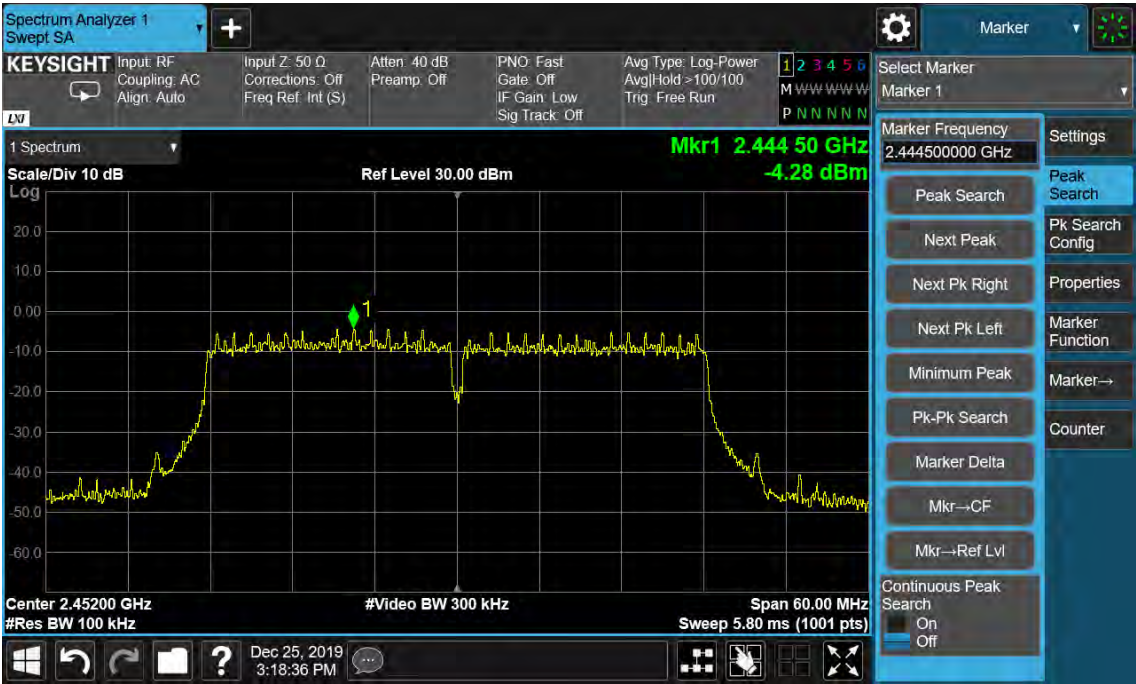
Figure 63: Conducted Spurious Emission & Authorized-band band-edge, 802.11n(HT40), 2452MHz Carrier Level
