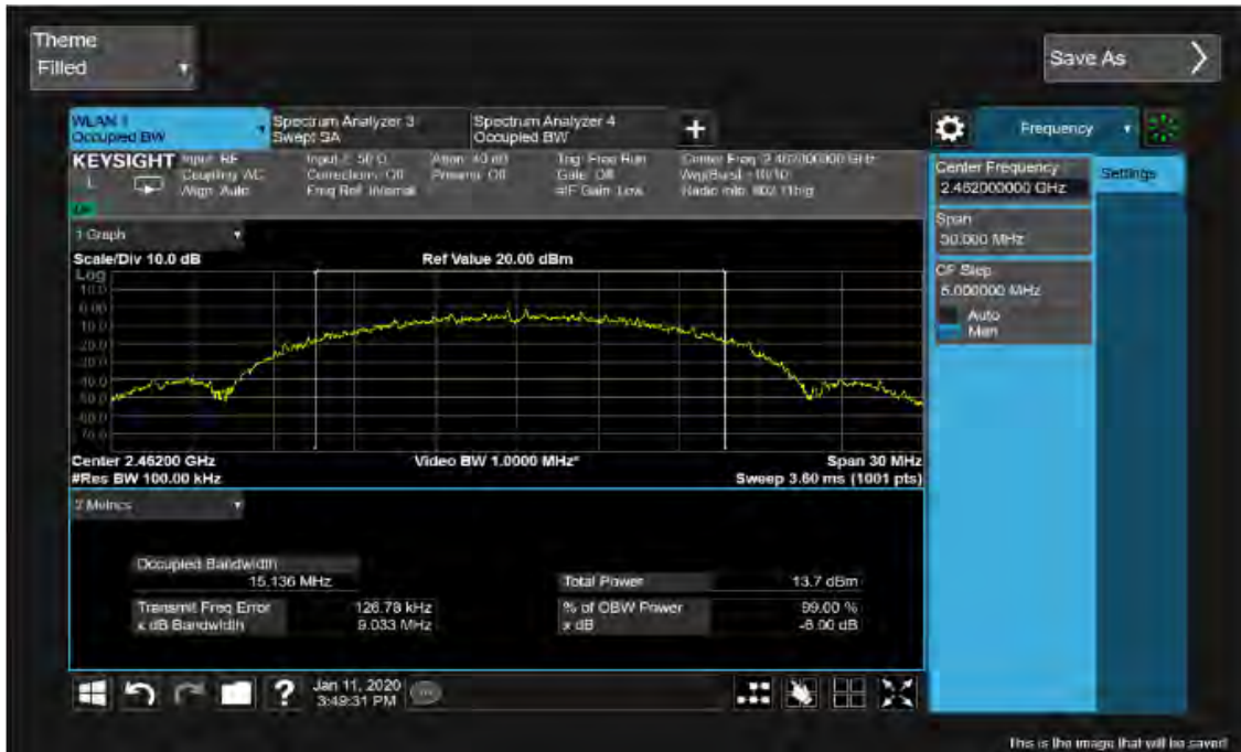
Figure 4: 6dB Bandwidth and 99% Bandwidth, 802.11g, 2412MHz
