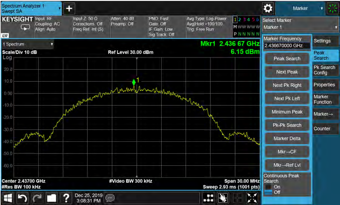
Figure 50: Conducted Spurious Emission & Authorized-band band-edge, 802.11b, 2437MHz Carrier Level
