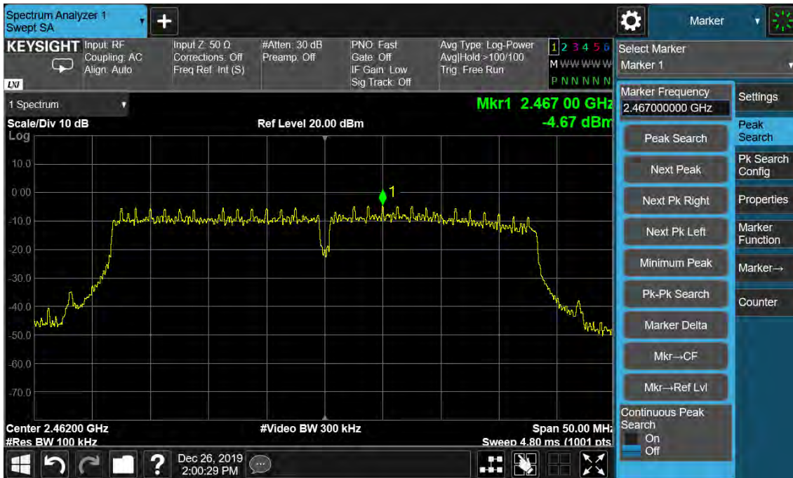
Figure 64: Conducted Spurious Emission & Authorized-band band-edge, 802.11n(HT40), 2462MHz Carrier Level
