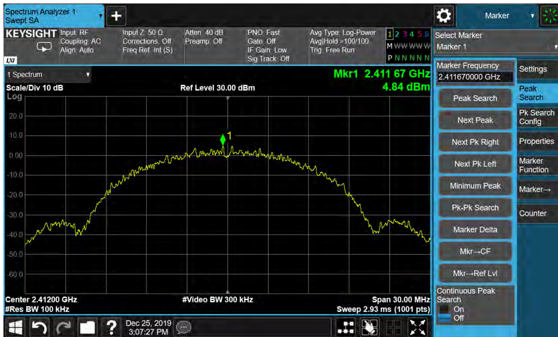
Figure 49: Conducted Spurious Emission & Authorized-band band-edge, 802.11b, 2412MHz Carrier Level
