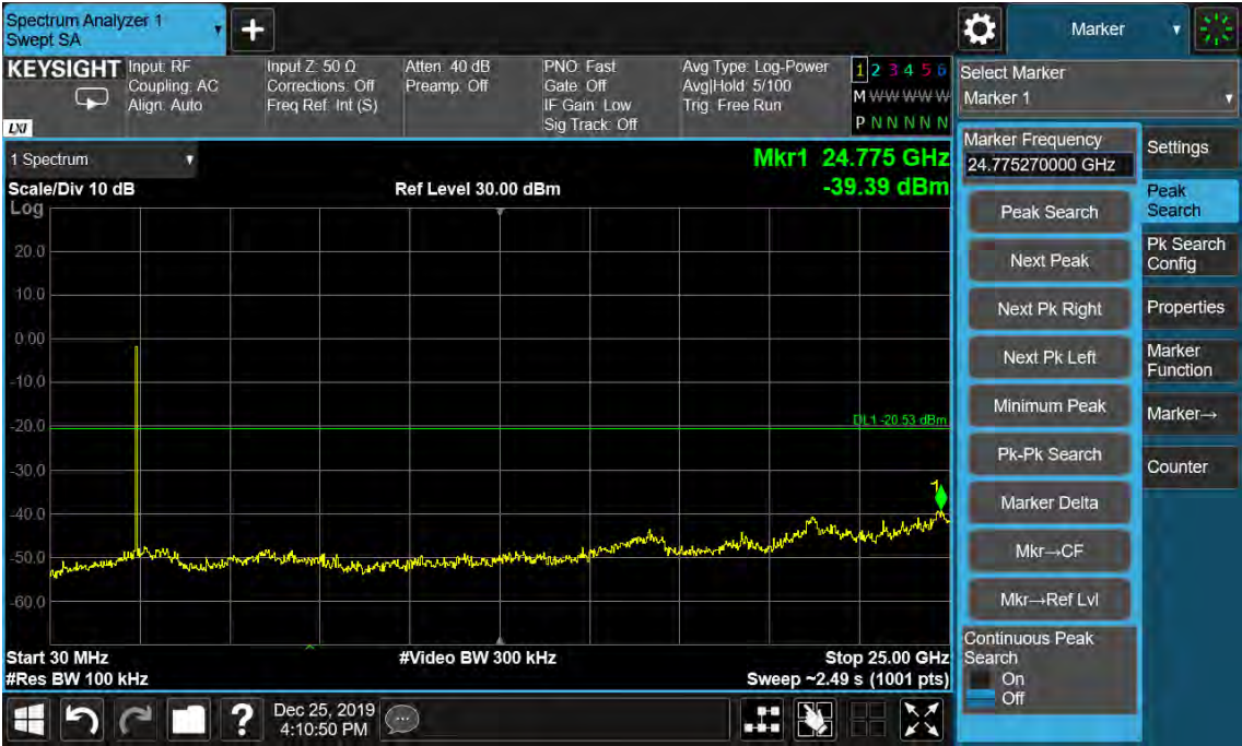
Figure 55: Conducted Spurious Emission & Authorized-band band-edge, 802.11g, 2462MHz Carrier Level
