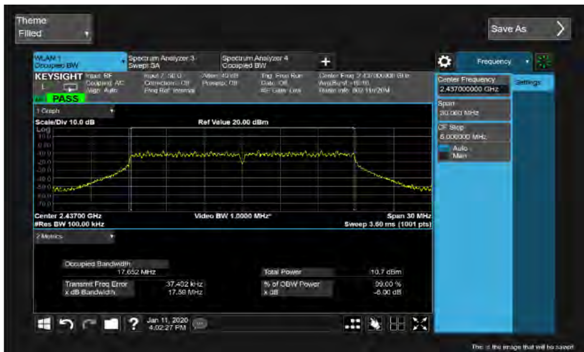
Figure 8: 6dB Bandwidth and 99% Bandwidth, 802.11n(HT20), 2437MHz
