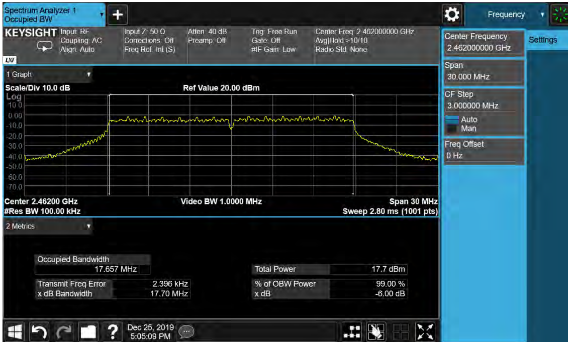
Figure 21: 6dB Bandwidth and 99% Bandwidth, 802.11n(HT20), 2462MHz
