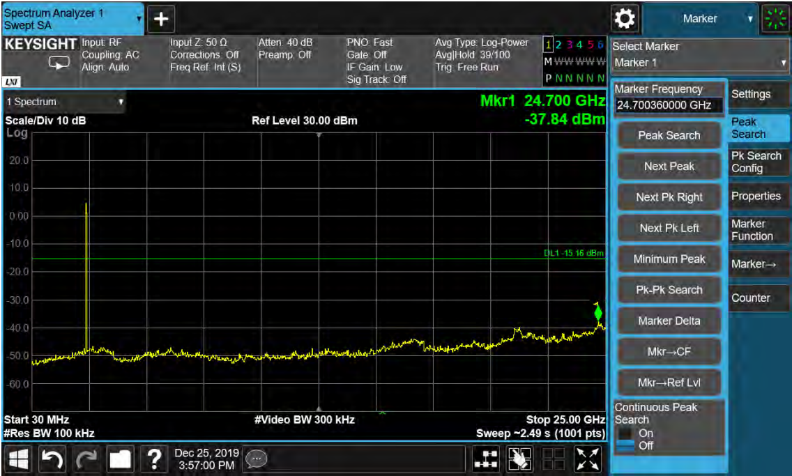
Figure 50: Conducted Spurious Emission & Authorized-band band-edge, 802.11b, 2437MHz Carrier Level
