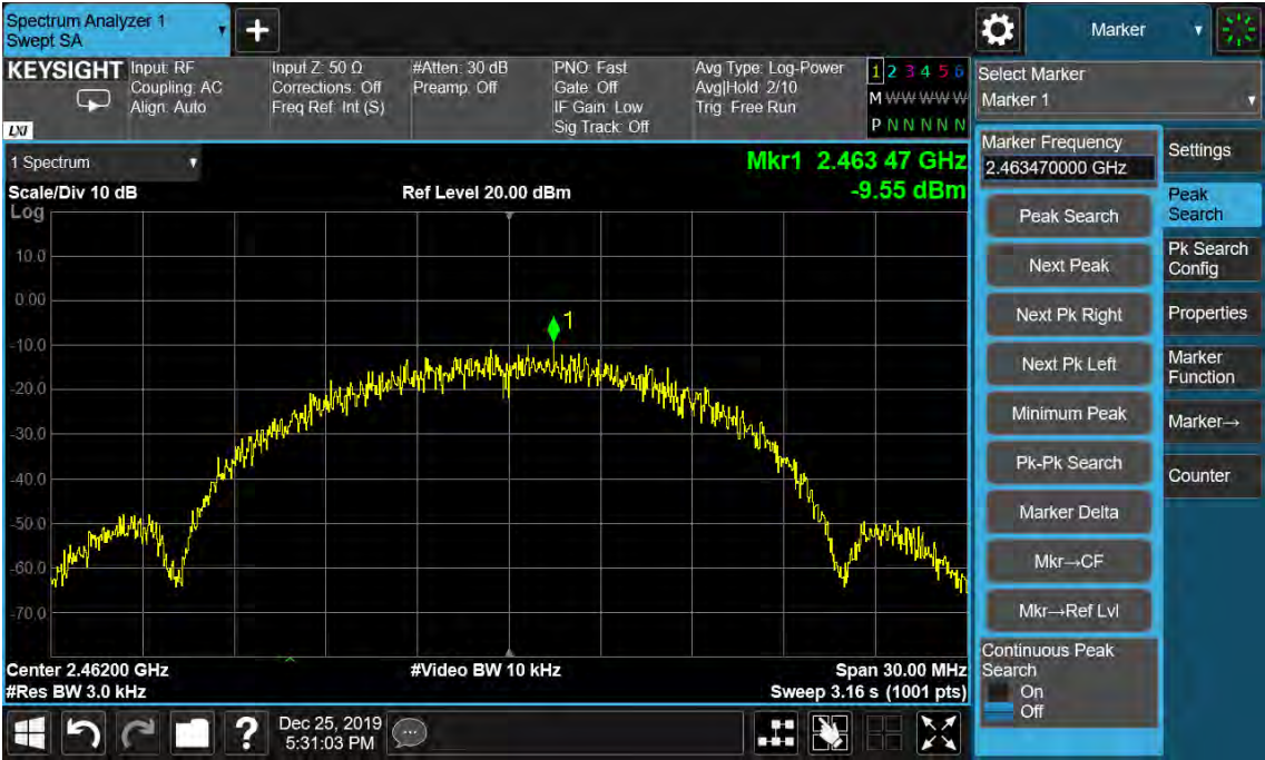
Figure 39: Power Spectral Density, 802.11b, 2452MHz
