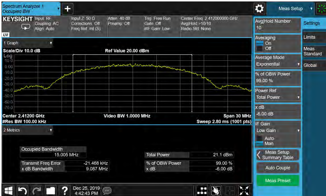
Figure 14: 6dB Bandwidth and 99% Bandwidth, 802.11b, 2437MHz
