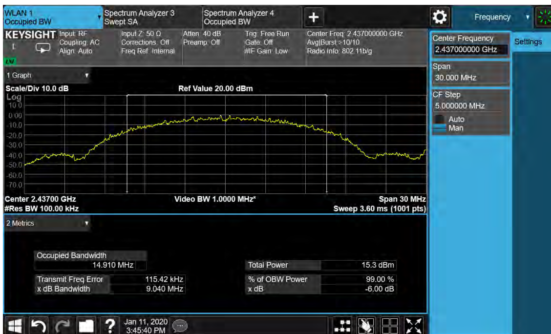
Figure 2: 6dB Bandwidth and 99% Bandwidth, 802.11b, 2437MHz
