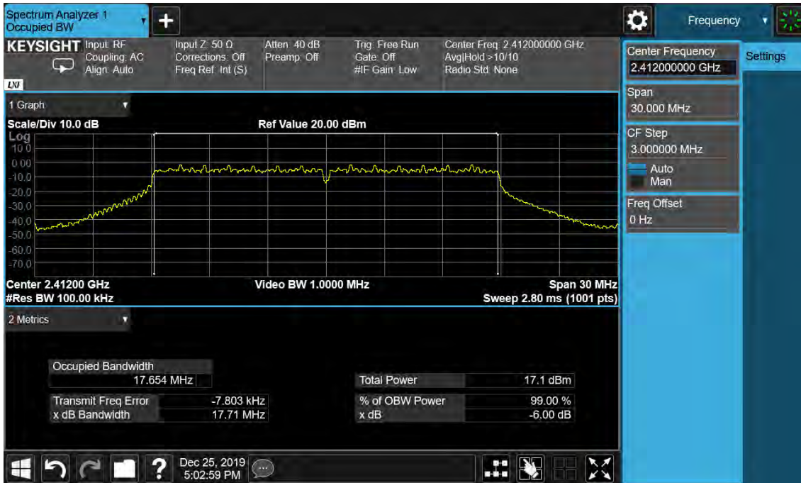
Figure 19: 6dB Bandwidth and 99% Bandwidth, 802.11n(HT20), 2412MHz
