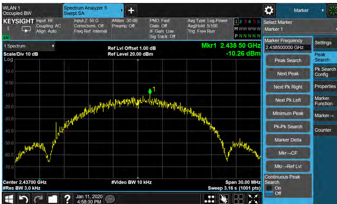
Figure 26: Power Spectral Density, 802.11b, 2437MHz
