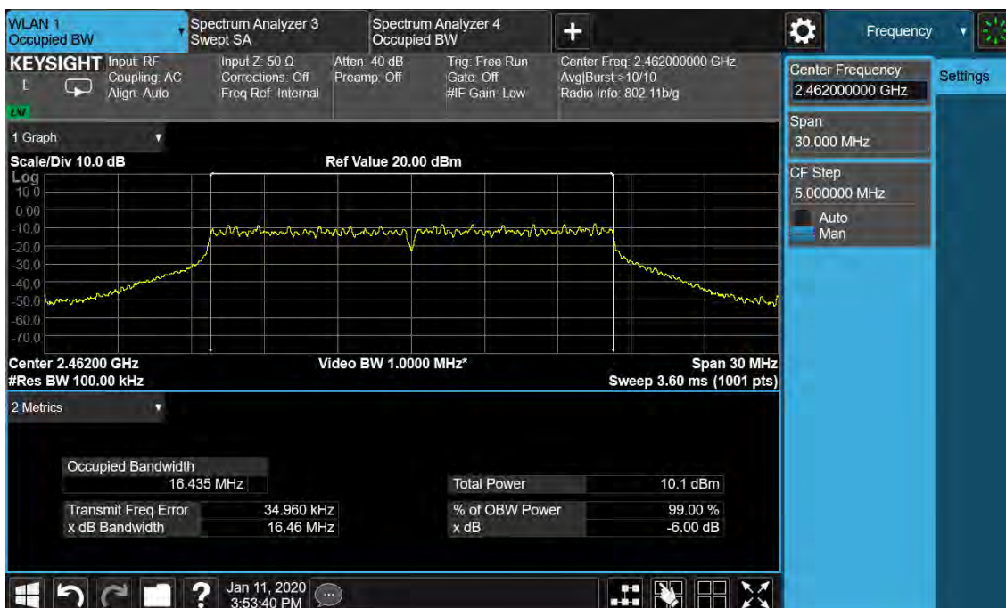
Figure 6: 6dB Bandwidth and 99% Bandwidth, 802.11g, 2462MHz
