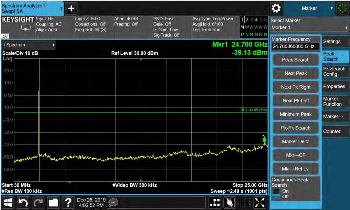
Figure 51: Conducted Spurious Emission & Authorized-band band-edge, 802.11b, 2462MHz Carrier Level
