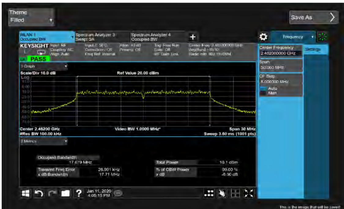
Figure 10: 6dB Bandwidth and 99% Bandwidth, 802.11n(HT40), 2422MHz
