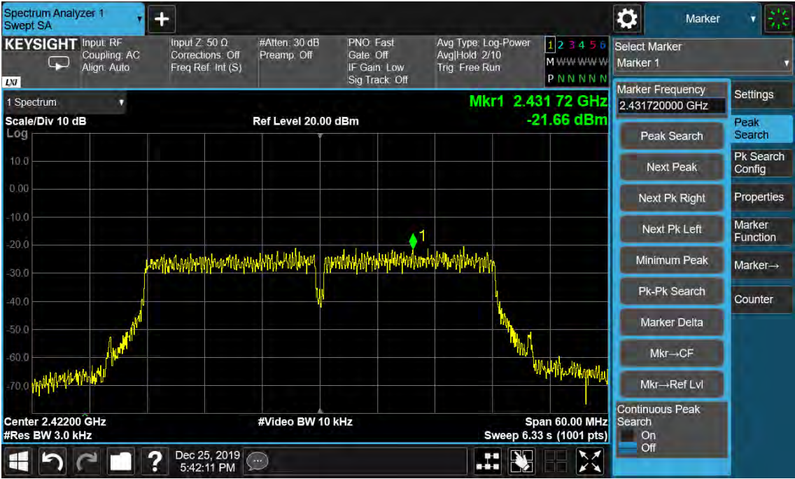
Figure 46: Power Spectral Density, 802.11n(HT40), 2422MHz
