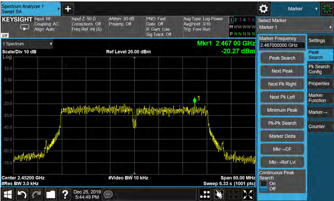
Figure 48: Power Spectral Density, 802.11n(HT40), 2452MHz
