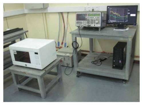
Radiated Emission Test Set-up (30 -1,000MHz):
