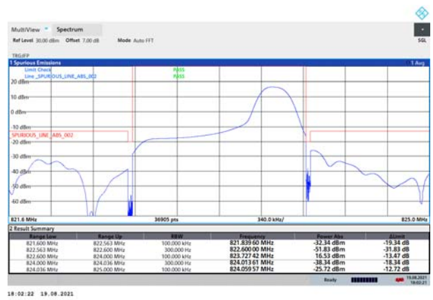
LTE eMTC Band 26 QPSK 1.4MHz CH-High 100%RB
