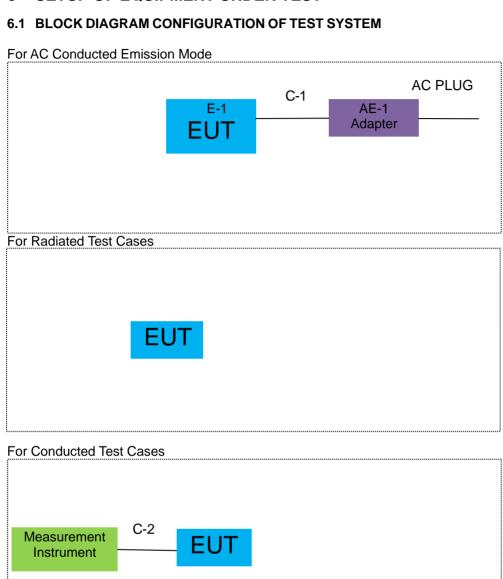
Note: The temporary antenna connector is soldered on the PCB board in order to perform conducted tests and this temporary antenna connector is listed in the equipment list.
