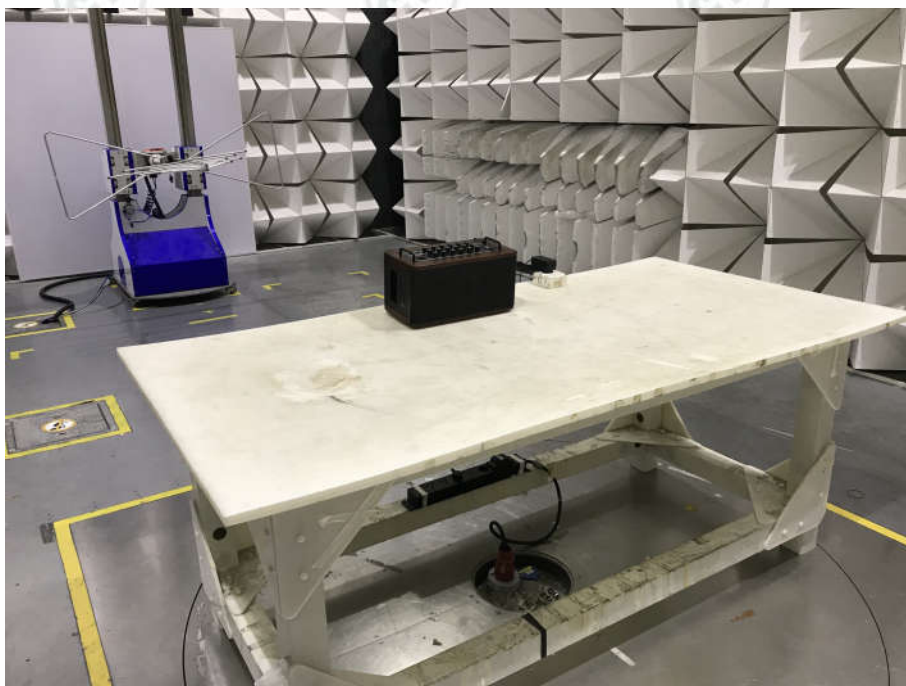
Radiated spurious emission Test Setup-2 (Below 1GHz)
