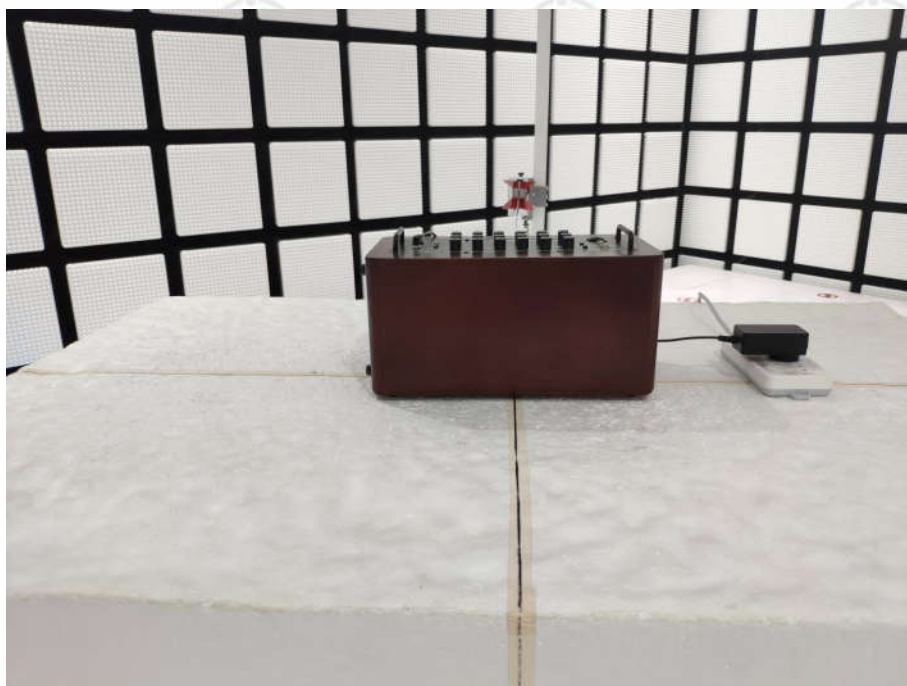
Radiated spurious emission Test Setup-3(Above 1GHz)
