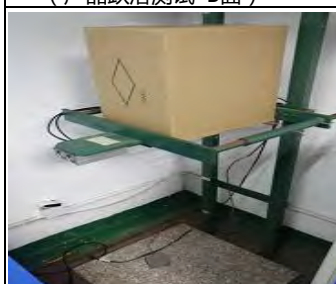
Step 6. Product drop test -D surface (产品跌落测试-D面)
