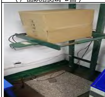
Step 8. Product drop test -F surface (产品跌落测试-F面)
