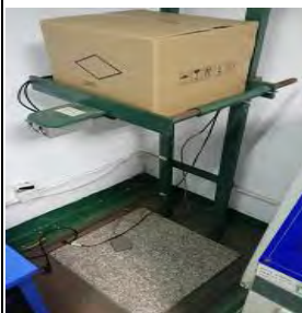
Step 3. Product drop test -A surface (产品跌落测试-A面)
