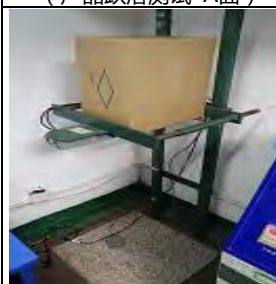
Step 5. Product drop test -C surface (产品跌落测试-C面)
