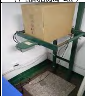
Step 7. Product drop test -E surface (产品跌落测试-E面)
