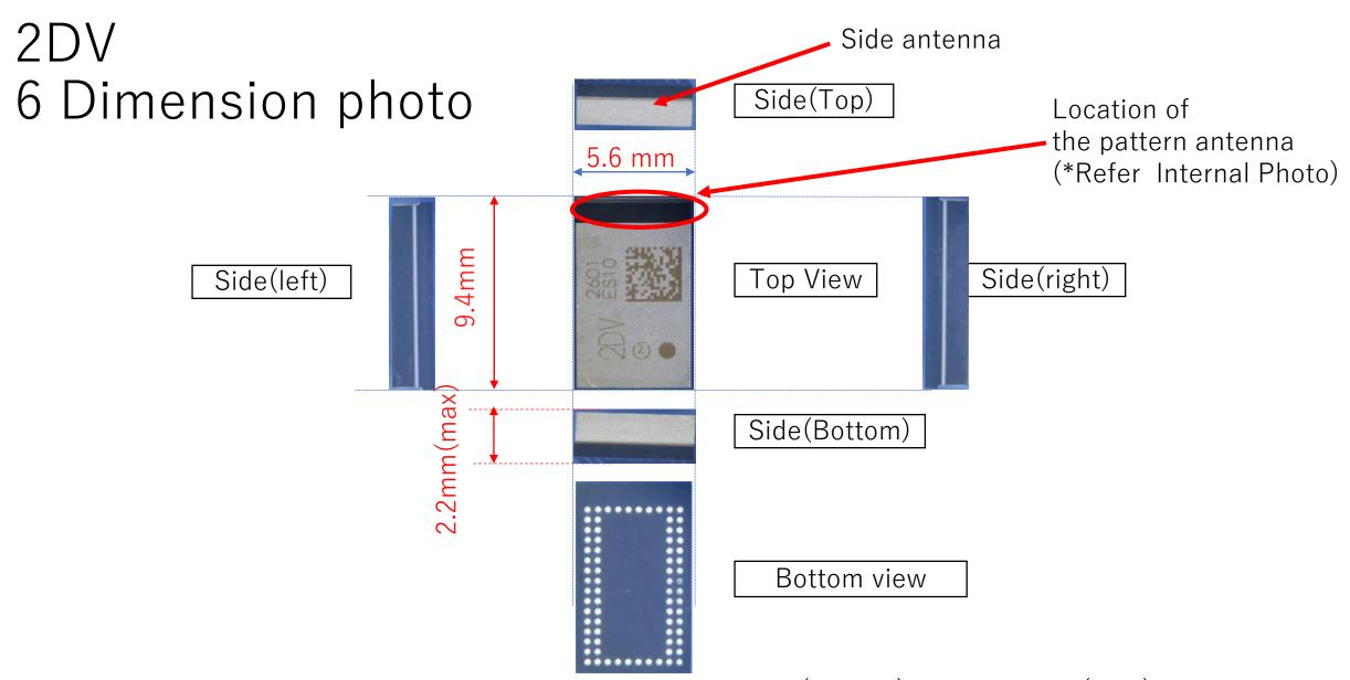
Weight: 0.303g Surface mount type:  $9.4 \times 5.6$  mm (Typical), H = 2.2 mm (Max)
