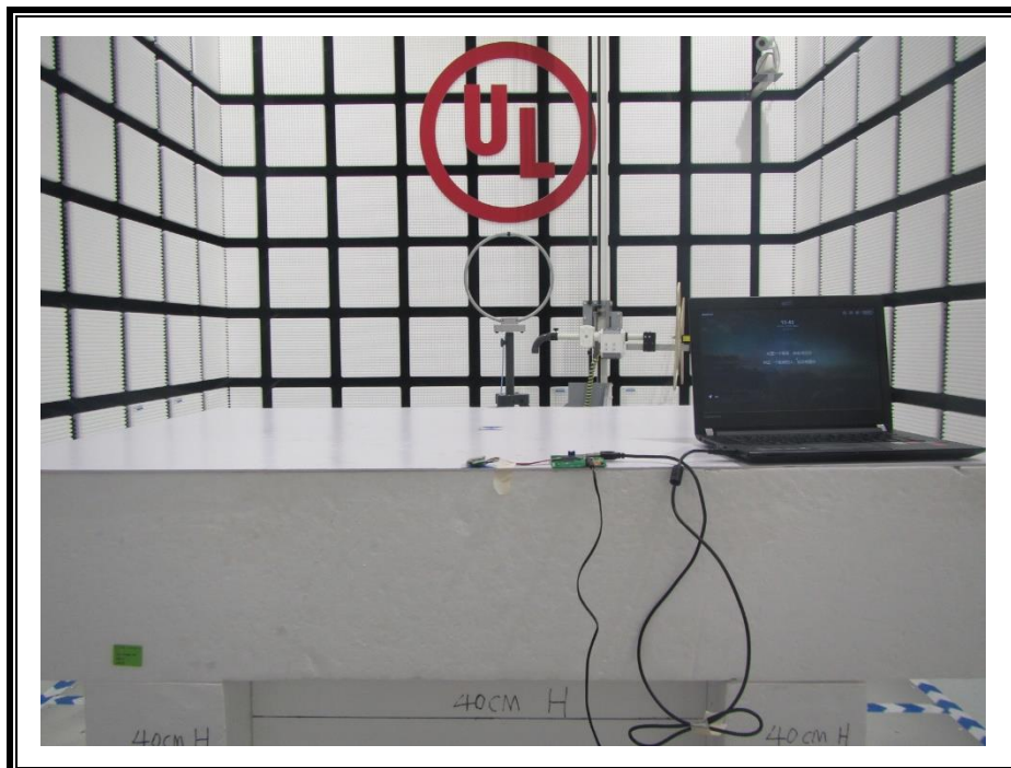
RADIATED RF MEASUREMENT SETUP (Below 30MHz)
