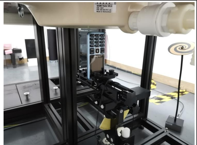
Bottom Side with earphone (10mm)
