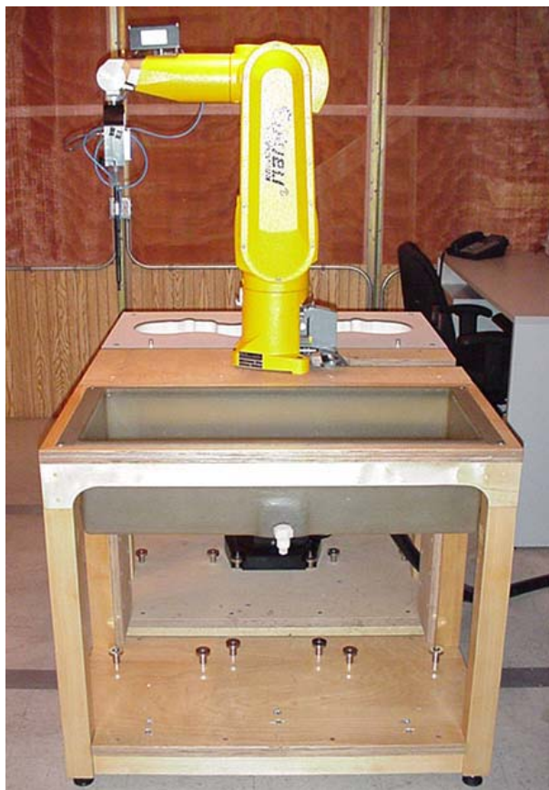
DASY4 SAR Measurement System with planar phantom
