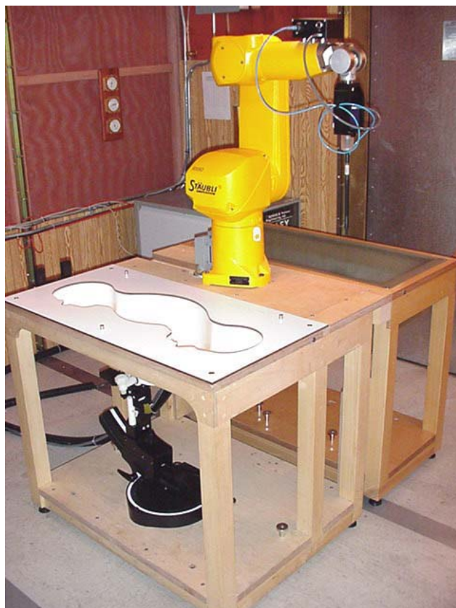
DASY4 SAR Measurement System with SAM phantom
