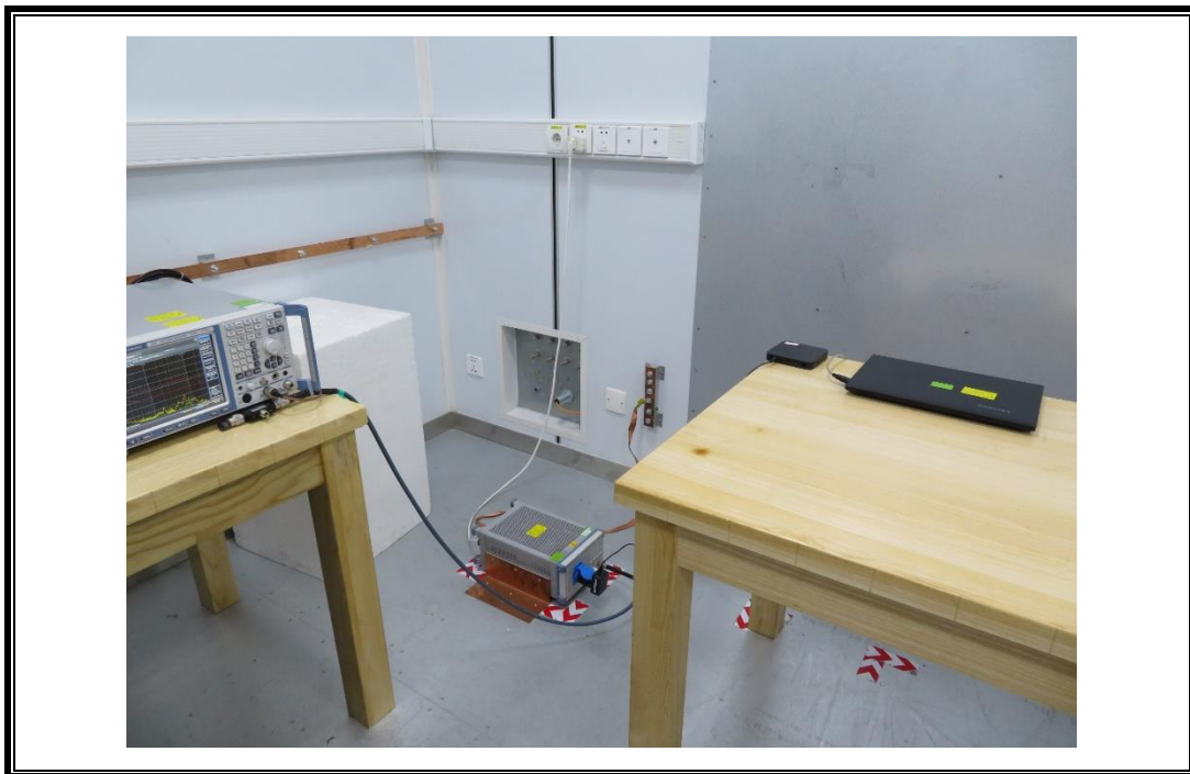
POWERLINE CONDUCTED EMISSIONS MEASUREMENT SETUP-1
