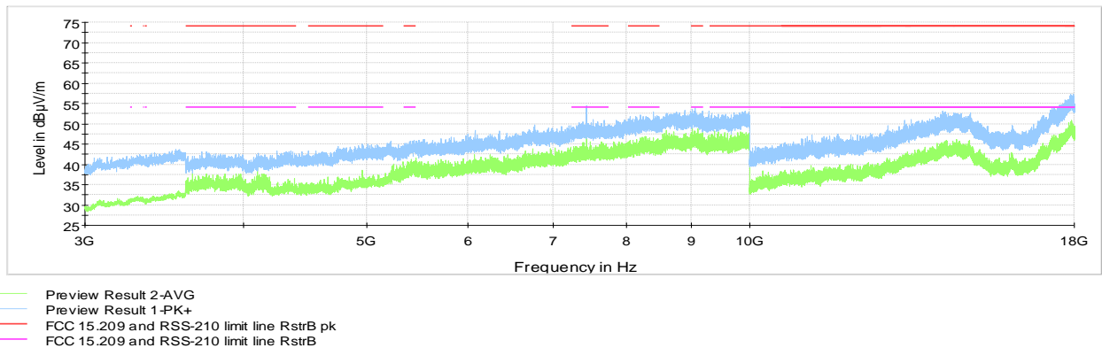
Figure 8.6-26: Radiated spurious emissions 3 to 18GHz, Tx at low channel, variant ES3026
