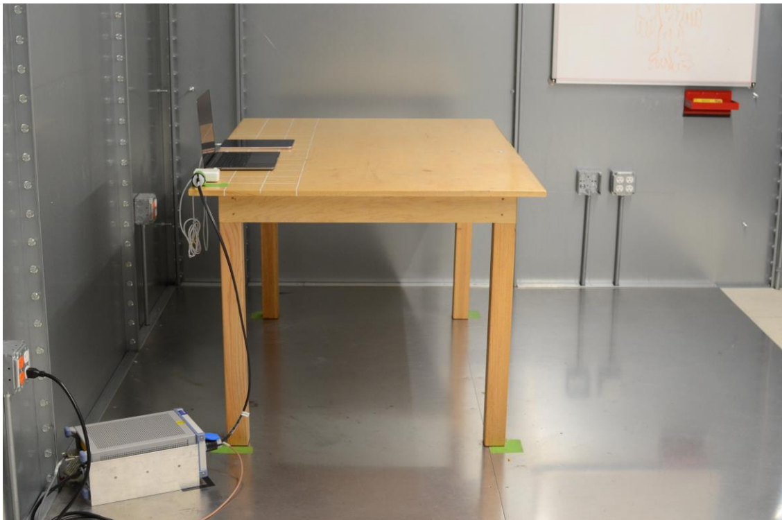
Figure 4: AC Line Conducted Emissions (Side View)
