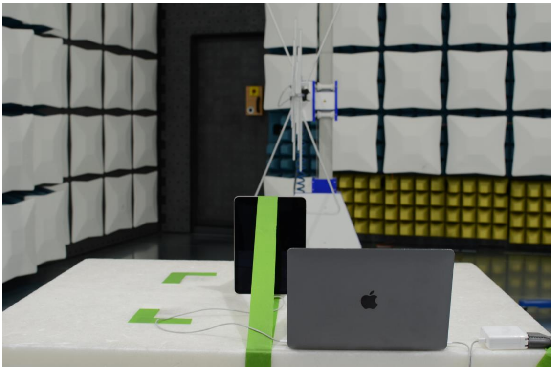
Figure 22: 30MHz-1GHz Test Setup (Rear View)
