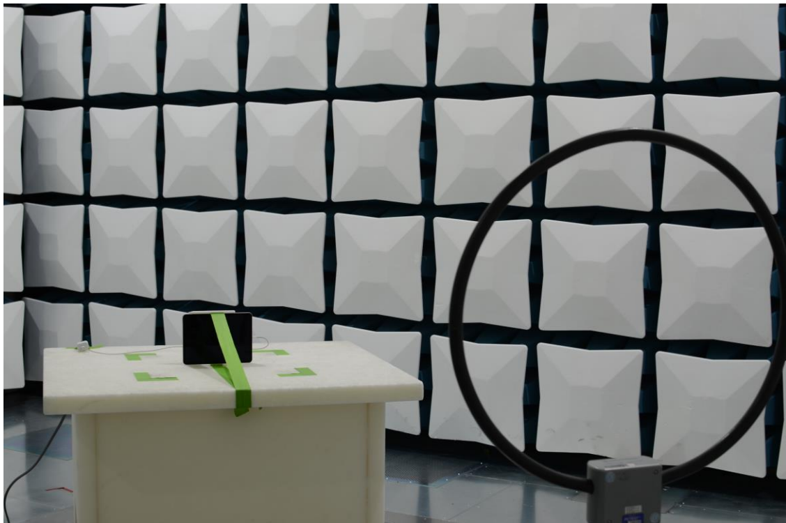
Figure 24: 9kHz-30MHz Test Setup (Front View)
