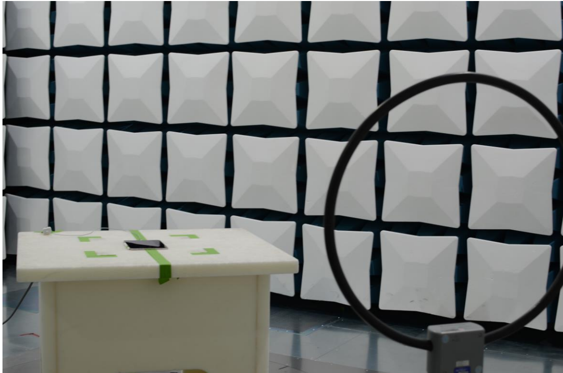
Figure 23: 9kHz-30MHz Test Setup (Front View)
