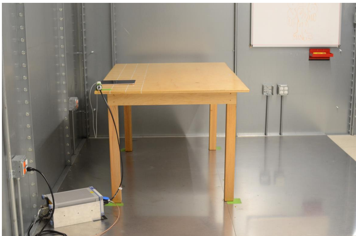
Figure 2: AC Line Conducted Emissions (Side View)
