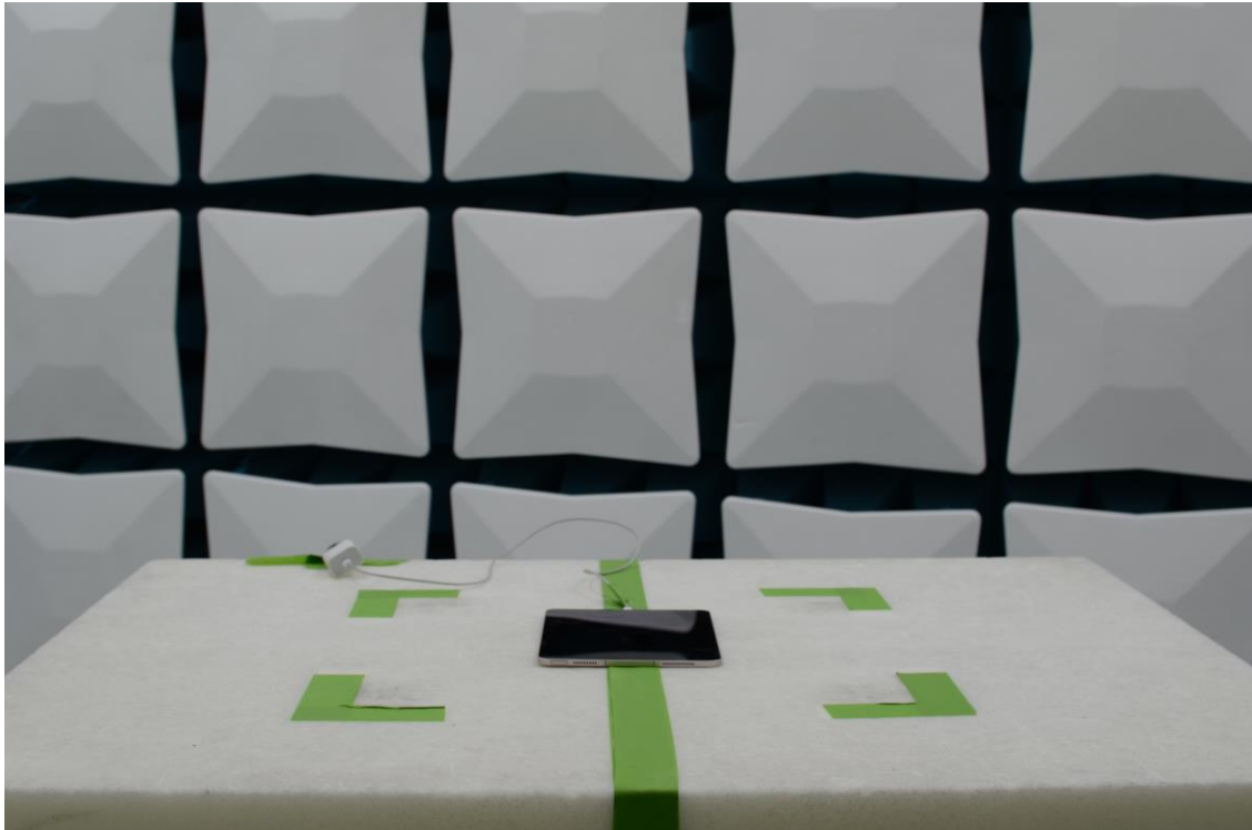
Figure 11: 30MHz-1GHz Test Setup (Front View)
