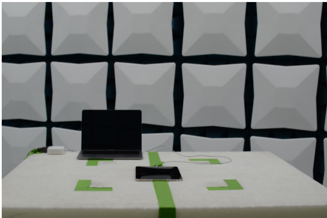
Figure 17: 30MHz-1GHz Test Setup (Front View)
