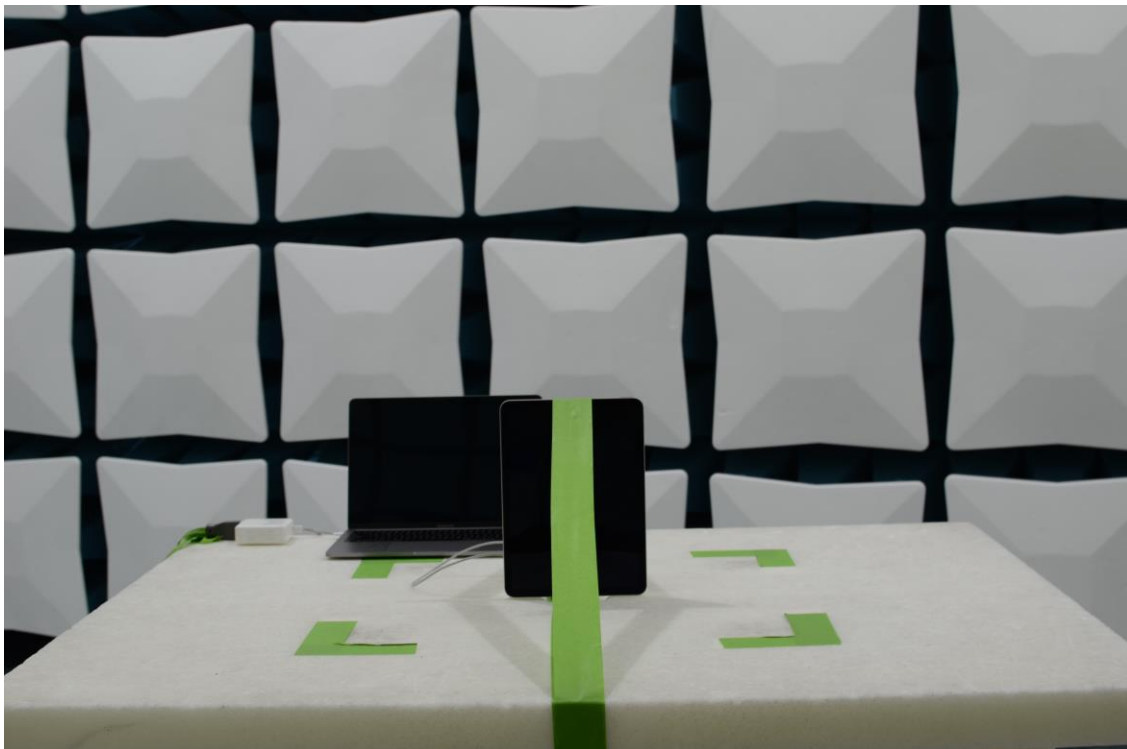
Figure 21: 30MHz-1GHz Test Setup (Front View)
