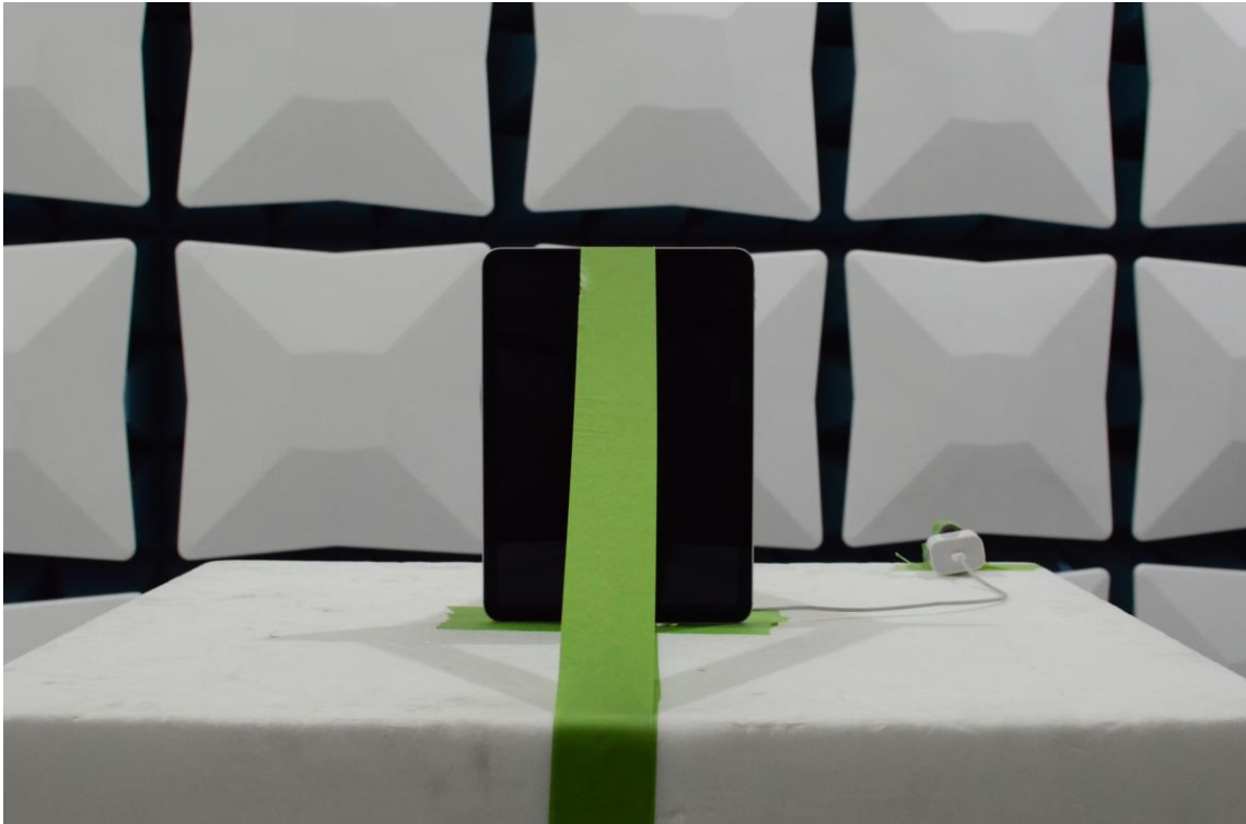
Figure 9: 1-18GHz Test Setup (Front View)
