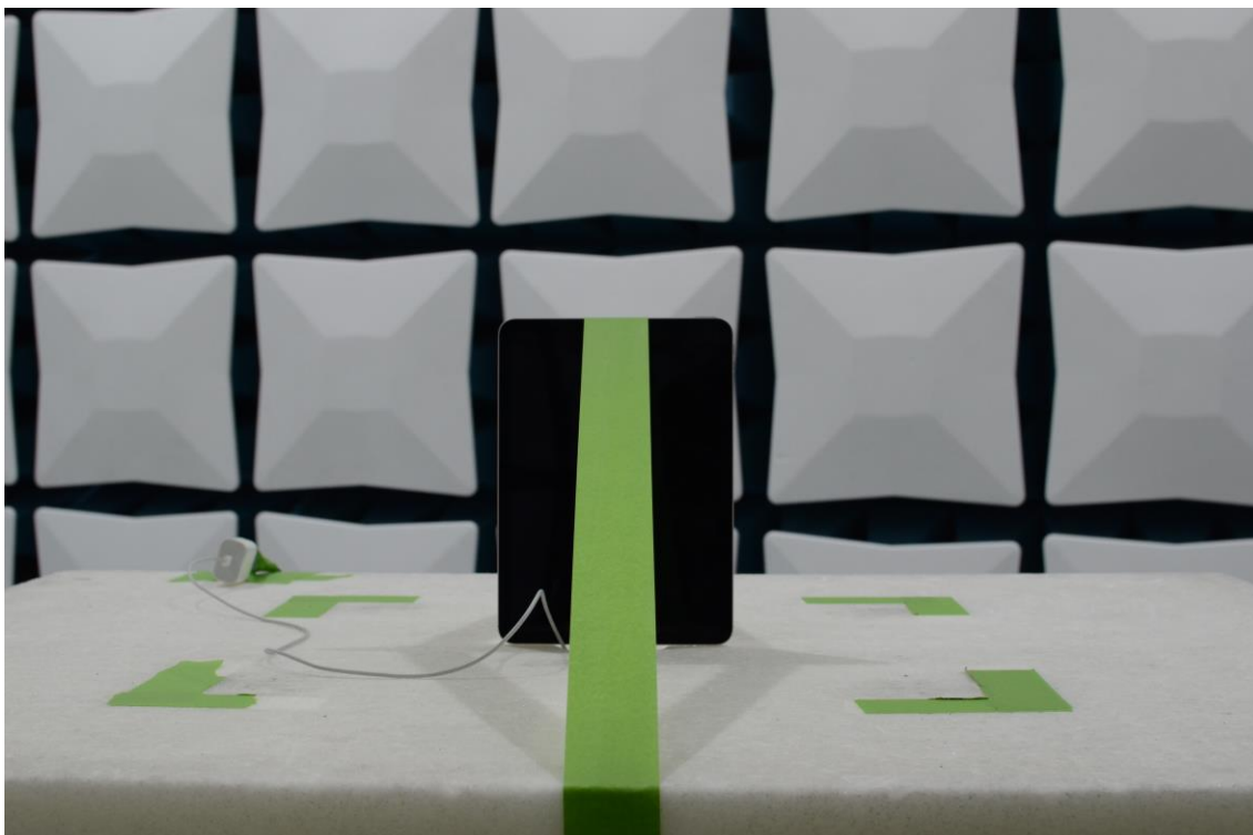
Figure 15: 30MHz-1GHz Test Setup (Front View)
