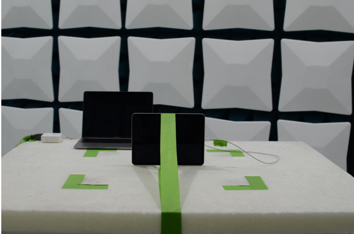
Figure 19: 30MHz-1GHz Test Setup (Front View)
