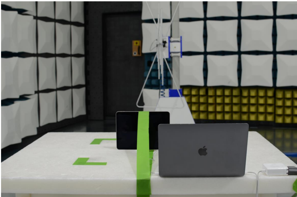
Figure 20: 30MHz-1GHz Test Setup (Rear View)
