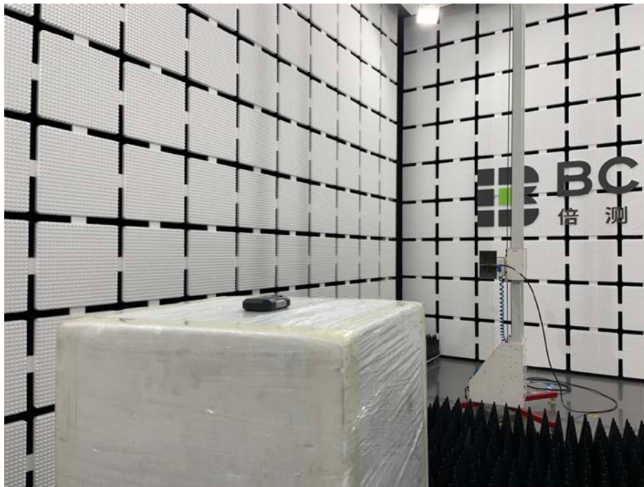
Spurious Emission Test Setup (Above 1GHz)
