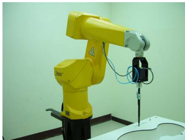
Fig. 5.2 Probe setup on robot
