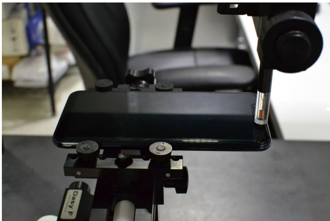
Figure 16-1 Test Setup for Wireless Device
