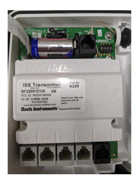
Location of ID Label is inside SIM panel door. Door is user-accessible. This product is designed to be installed outside. The purpose of locating the ID label inside the SIM is to ensure the ID label remains readable over the lifetime of the product.
