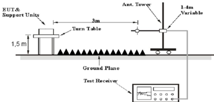
The radiated emission Below 1GHz tests were performed in the 3 meters chamber A, above 1GHz tests were performed in the 3 meters chamber B, using the setup accordance with the ANSI C63.10-2013. The specification used was the FCC 15.209, and FCC 15.247 limits.
