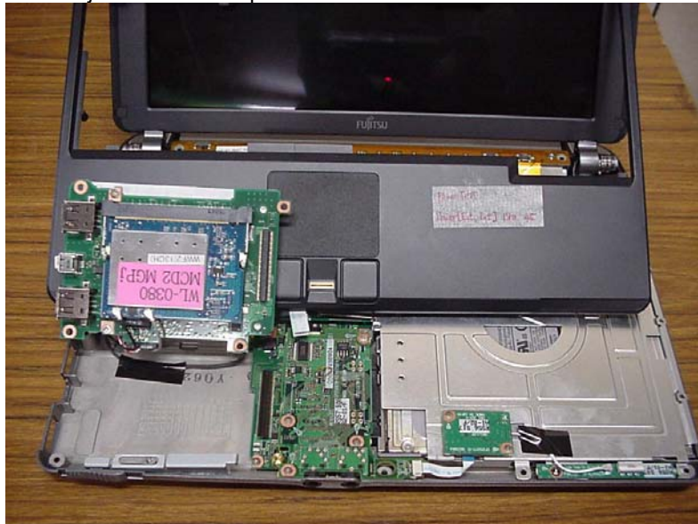
WLL-4070 Inside the Fujitsu Tablet Computer
