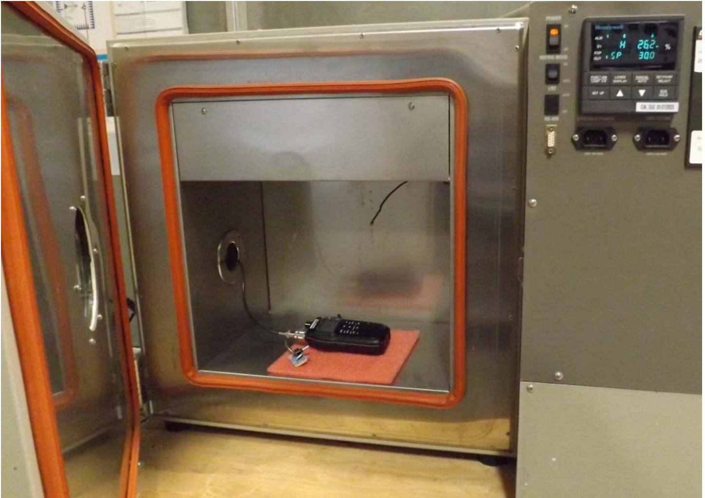
Figure E24.11 – Setup Photo – Frequency Stability
