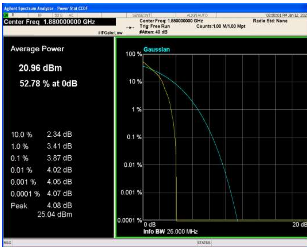
Band2 QAM16 BW=1.4MHz Channel=18900 RB Size=1 Position=#0
