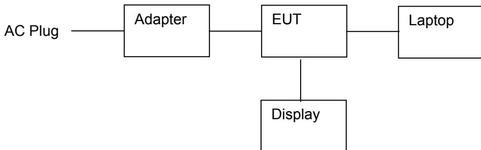
Operation of EUT during radiation above 1GHz testing:
