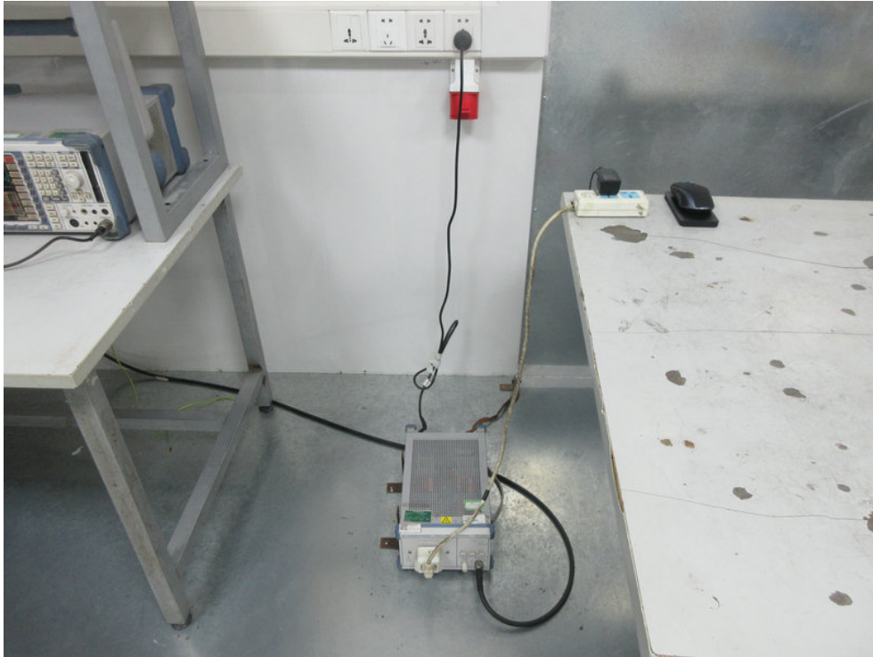
Photo of Power Line Conducted Emission Test
