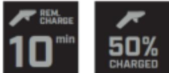
If no action after 15 sec on the controller the screen will close. If the user touch any buttons the screen will wake up to show the battery status
