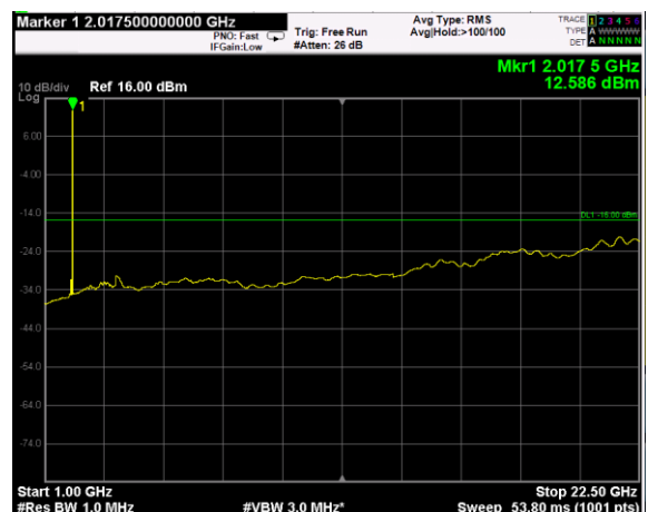
Channel: TOP, Modulation: QPSK, BW=5MHz, Range: Upper
