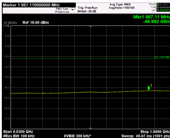
Channel: MIDDLE, Modulation: 64QAM, BW=15MHz, Range: Lower
