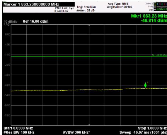
Channel: BOTTOM, Modulation: 16QAM, BW=15MHz, Range: Lower
