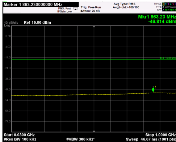
Channel: BOTTOM, Modulation: 256QAM, BW=15MHz, Range: Lower
