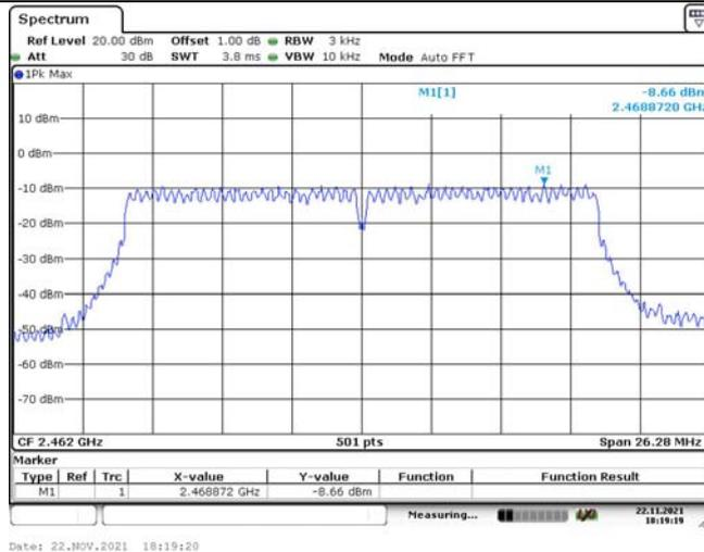
**4.6 100 kHz Bandwidth of Frequency Band Edge:**
