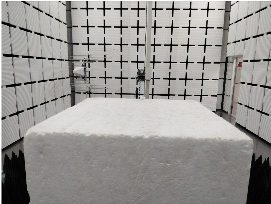
Radiated Spurious Emission (below 1GHz)
