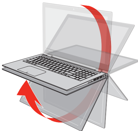
Figure 2-2 Opening the display panel to any angel (L50W-C)
