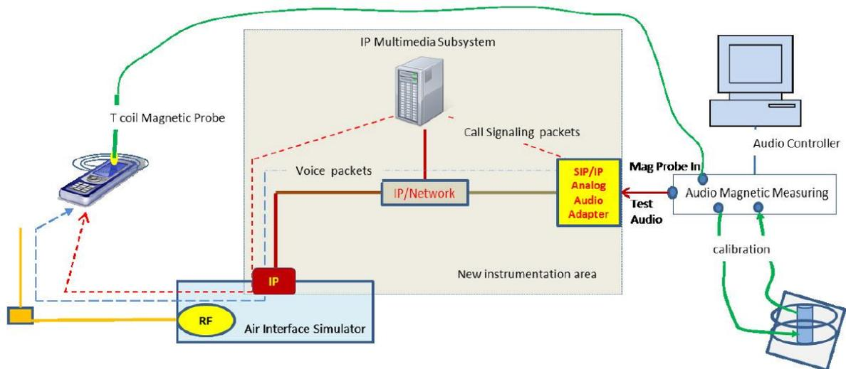
**Figure 11.1 Test Setup for VoWiFi over IMS T-coil Measurements**
