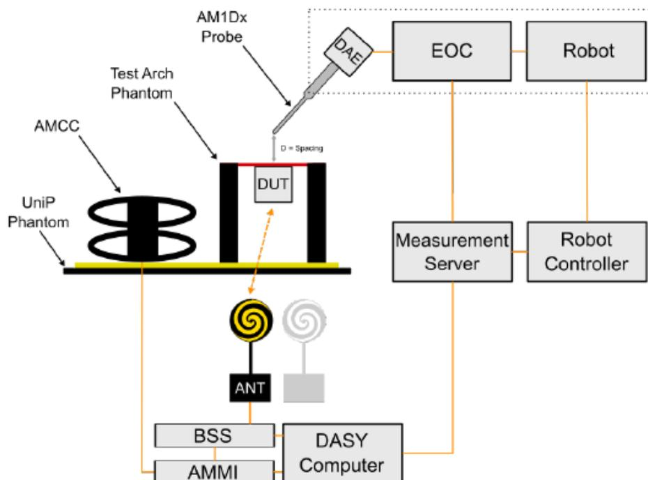
**Figure 5.1 HAC Test Measurement Set-up**
