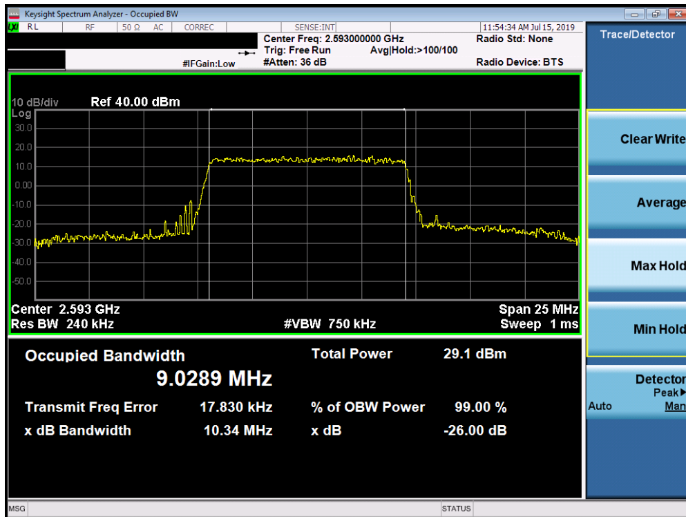
Plot 7-99. Occupied Bandwidth Plot (Band 41 - 10.0MHz 64-QAM - Full RB Configuration)
