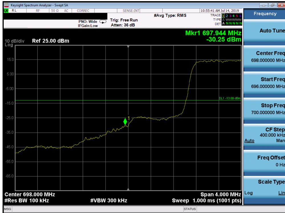
Plot 7-171. Lower Band Edge Plot (Band 12 - 1.4MHz QPSK - Full RB Configuration)
