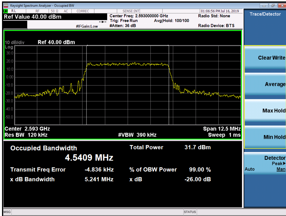
Plot 7-84. Occupied Bandwidth Plot (Band 41 - 5.0MHz 64-QAM - Full RB Configuration)
