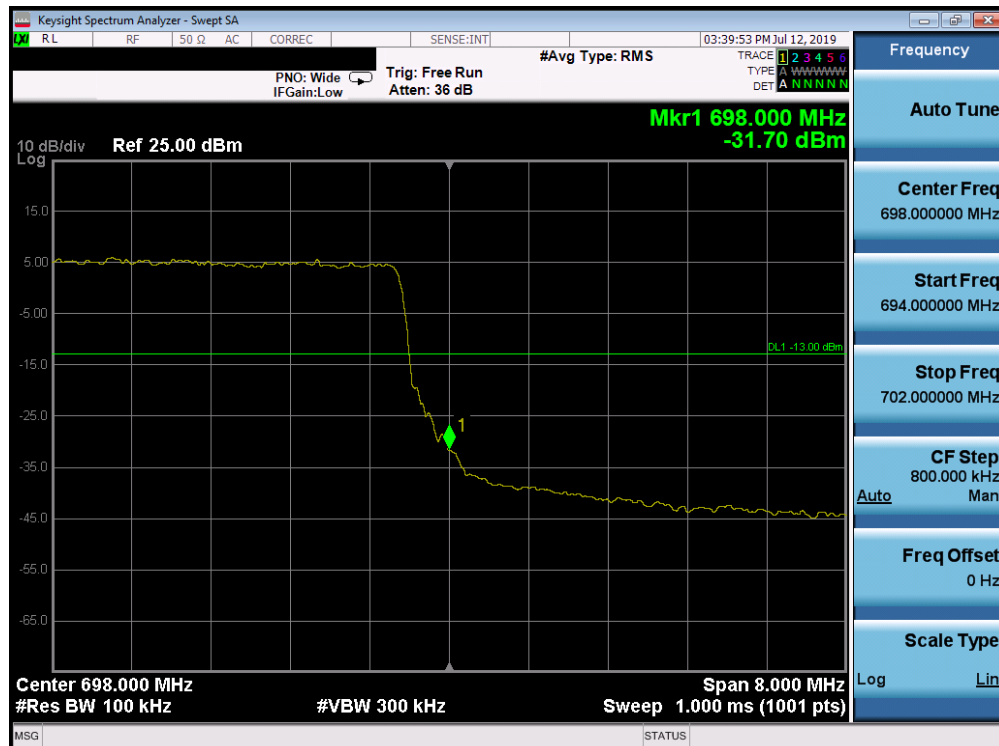
Plot 7-166. Upper Band Edge Plot (Band 71 - 10.0MHz QPSK - Full RB Configuration)
