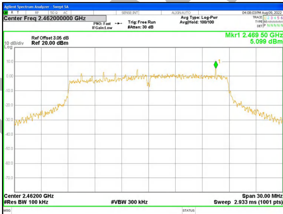
Band Edge NVNT n20 2462MHz Ant1 Emission
