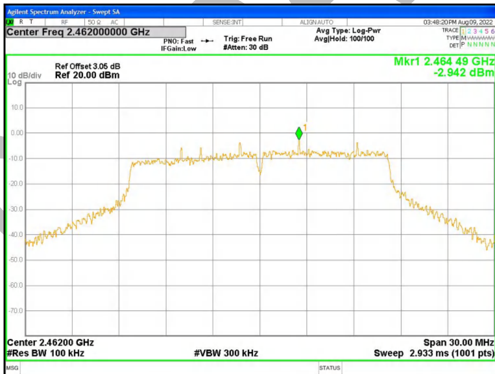
Band Edge NVNT g 2462MHz Ant1 Emission
