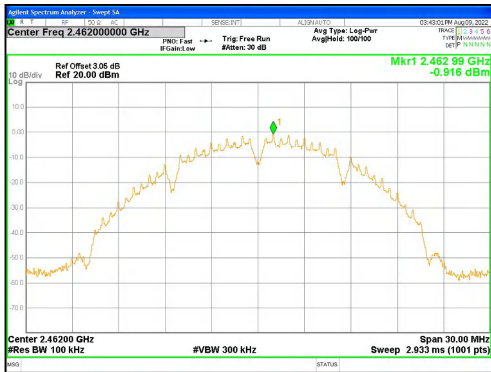
PSD NVNT b 2412MHz Ant2
