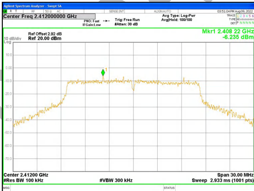
Band Edge NVNT g 2412MHz Ant2 Emission
