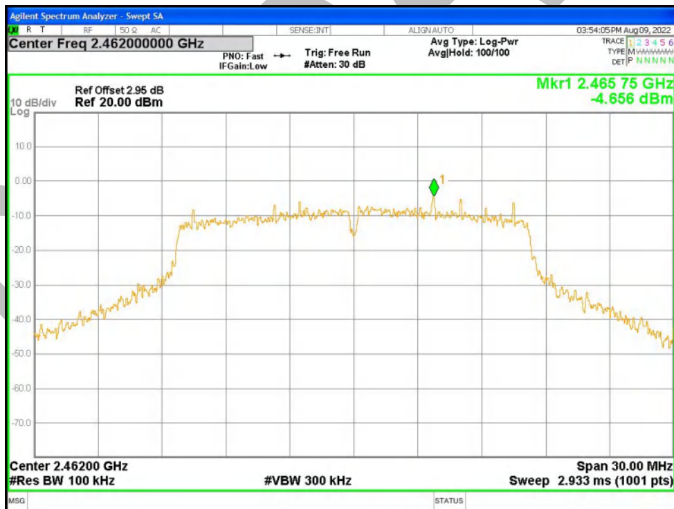
Band Edge NVNT g 2462MHz Ant2 Emission
