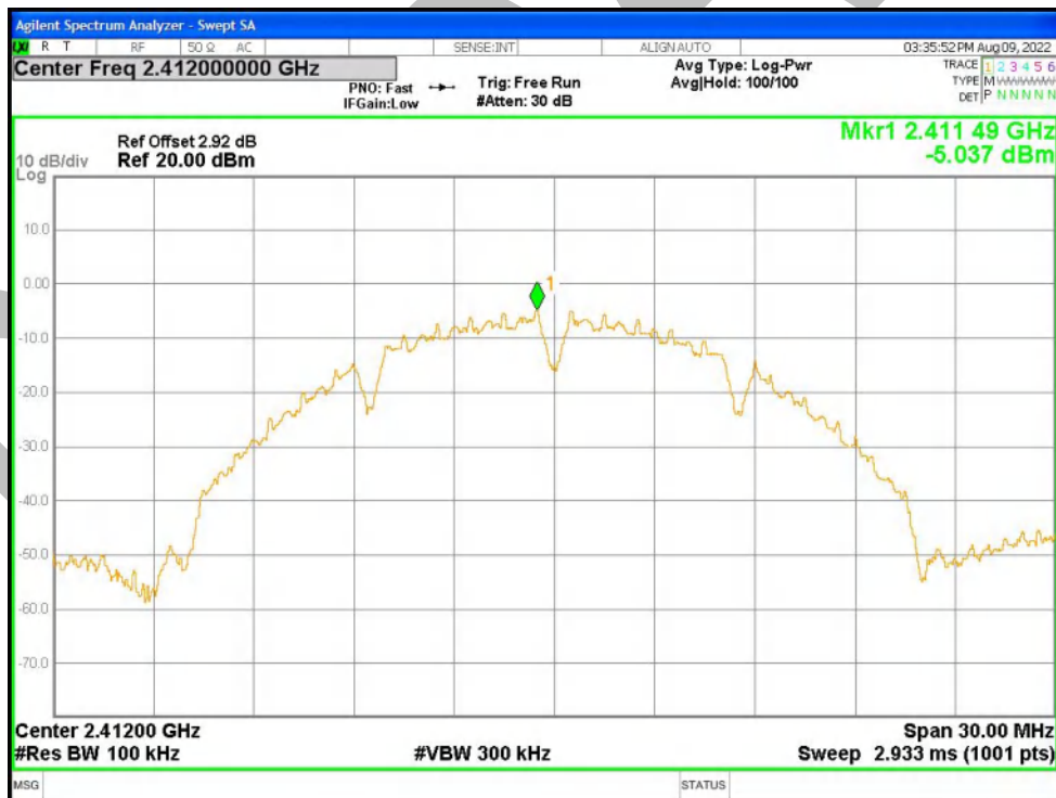
Band Edge NVNT b 2412MHz Ant2 Emission
