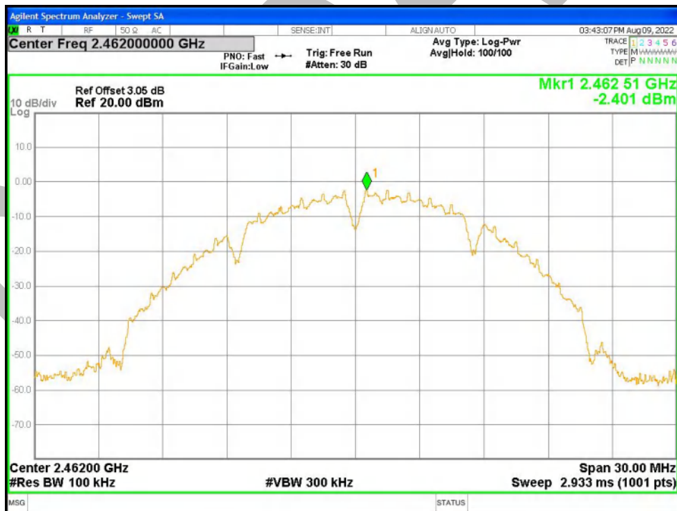
Band Edge NVNT b 2462MHz Ant1 Emission
