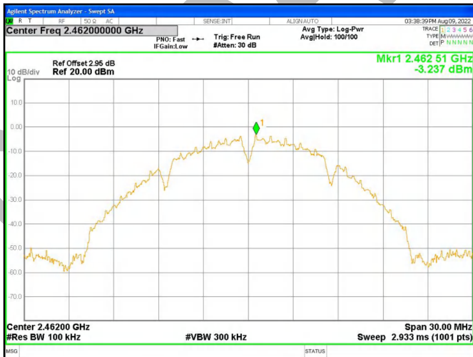
Band Edge NVNT b 2462MHz Ant2 Emission
