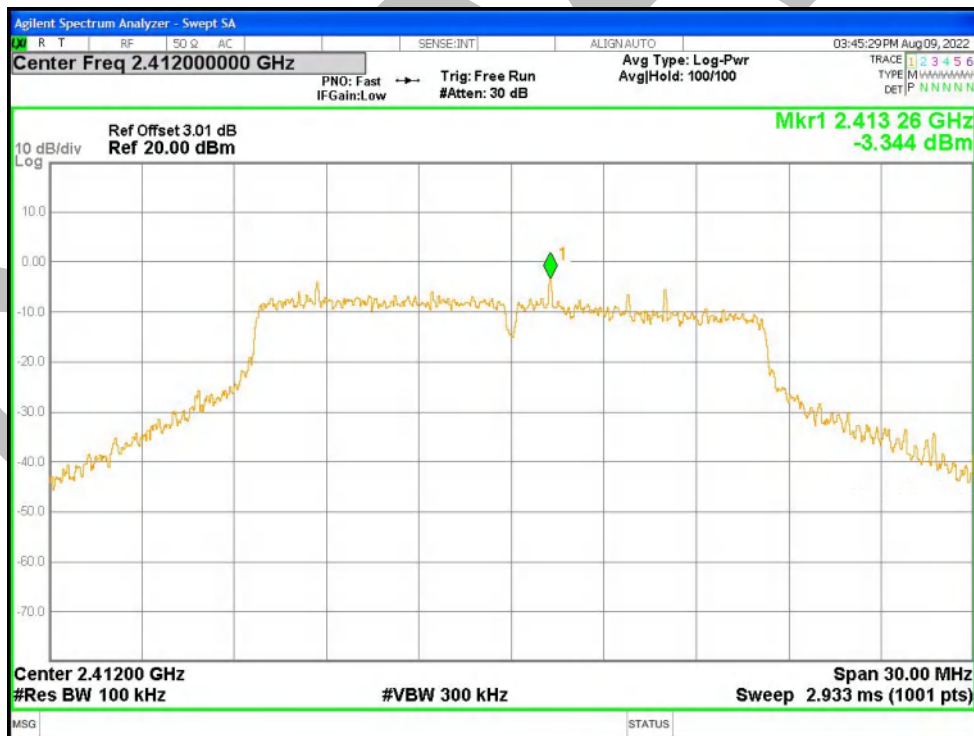
Band Edge NVNT g 2412MHz Ant1 Emission
