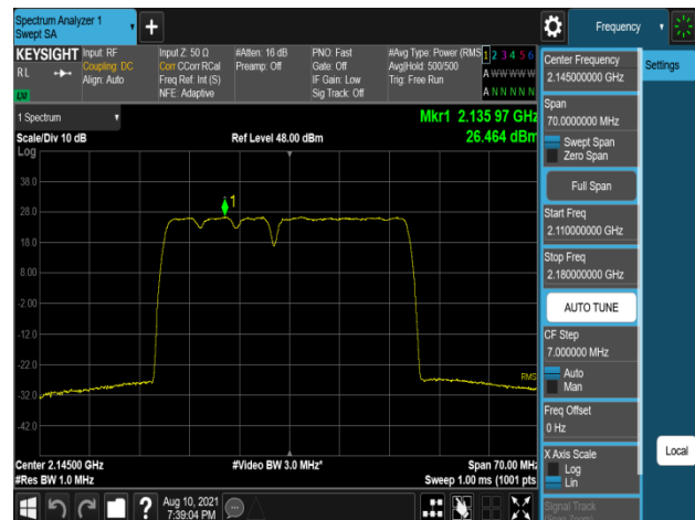
Plot 7-774. Peak Power Spectral Density Plot (B66_5M+5M+5M+20M_4C_16QAM - Mid Channel, Port 1)
