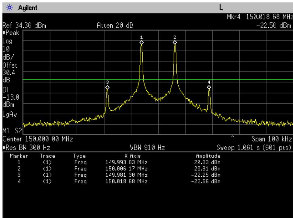
**Uplink 150 - 6.25 kHz - Intermodulation**
