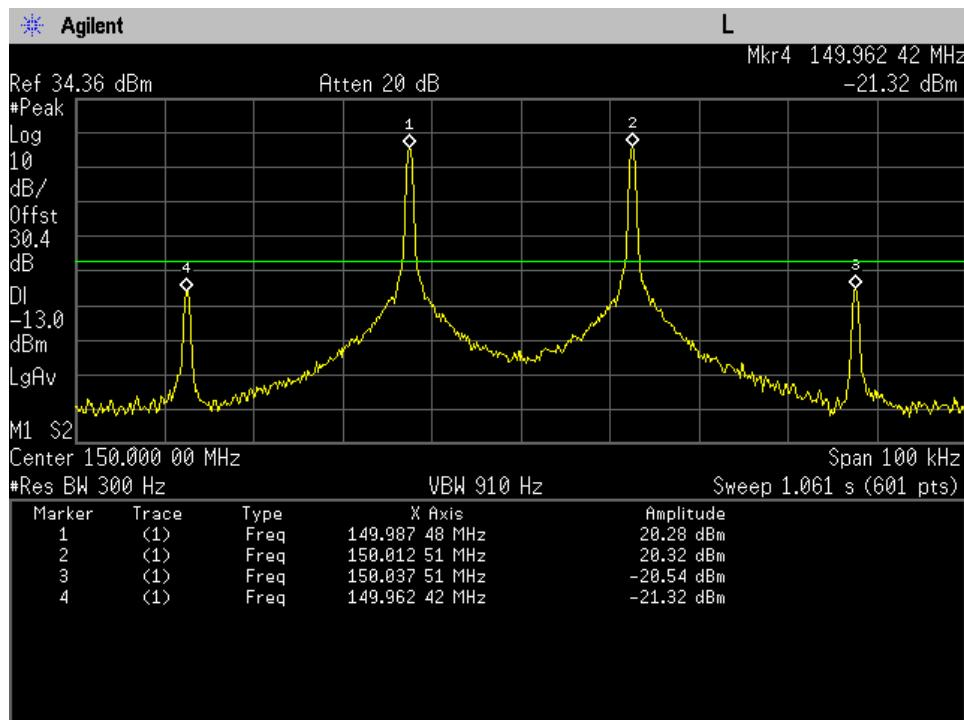
**Uplink 150 - 12.5 kHz - Intermodulation**
