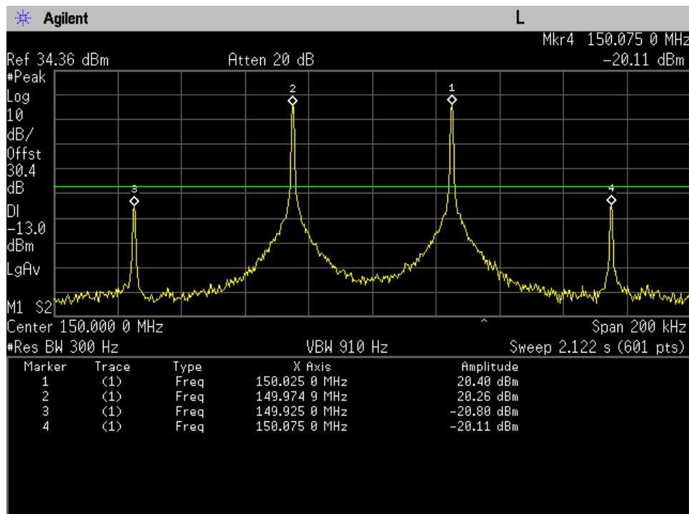
**Uplink 150 - 25 kHz - Intermodulation**
