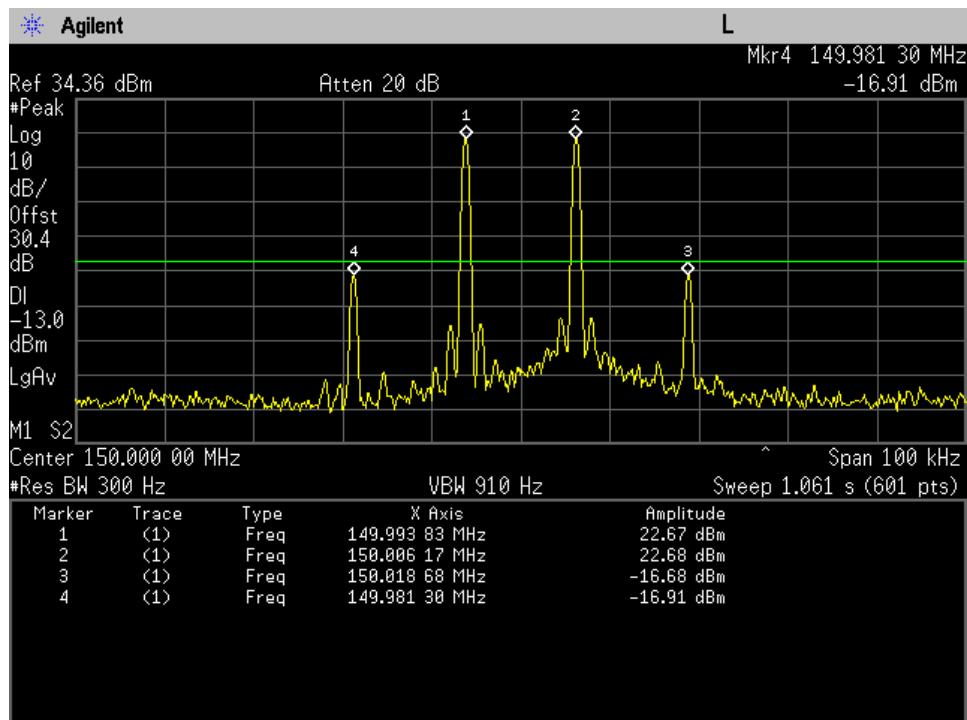
**Downlink 150 - 6.25 kHz - Intermodulation**
