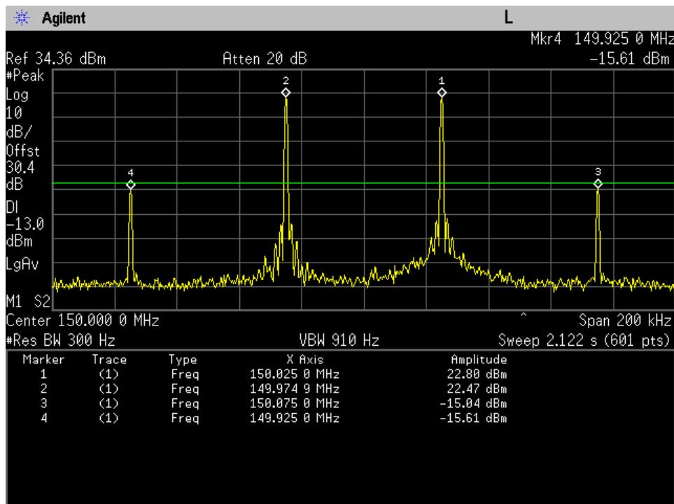
**Downlink 150 - 25 kHz - Intermodulation**
