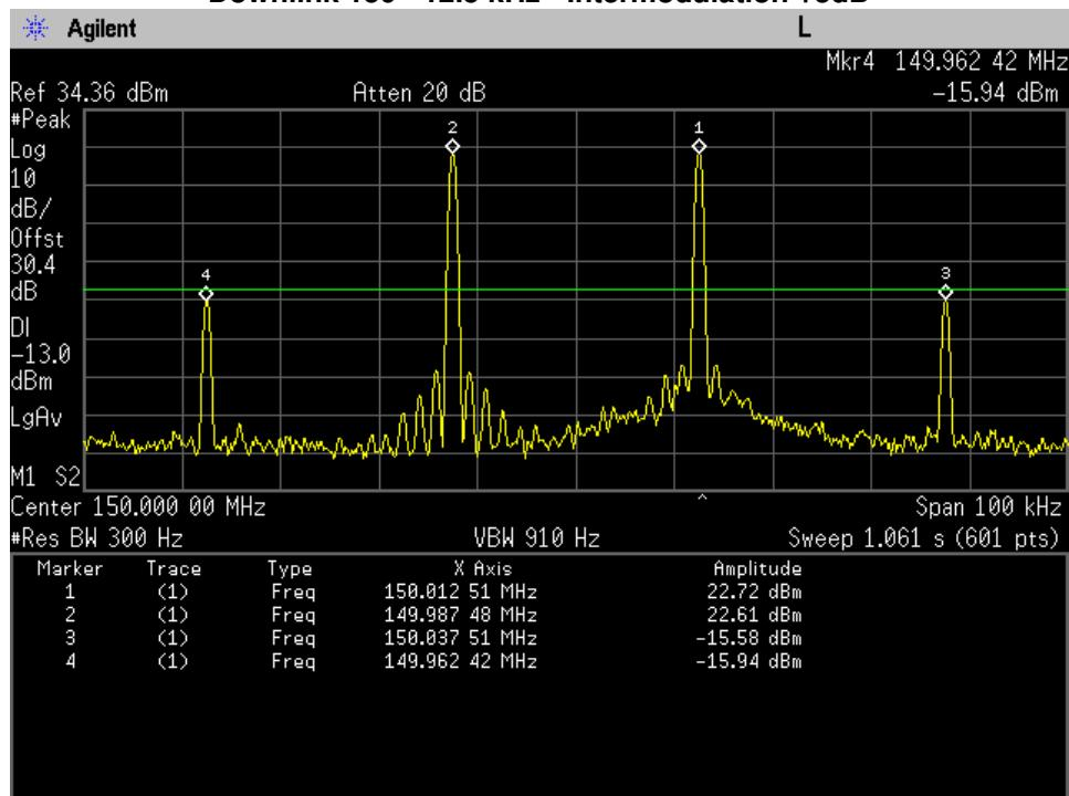
**Downlink 150 - 12.5 kHz - Intermodulation**
